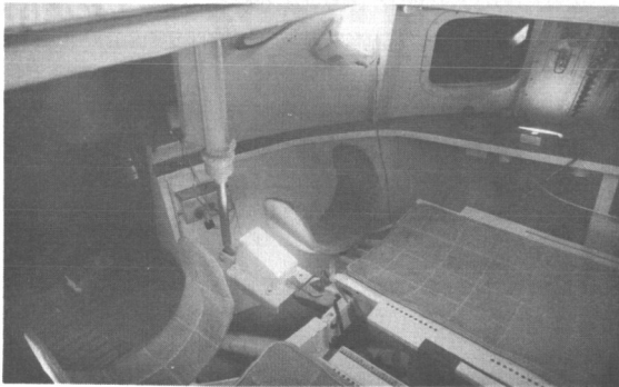
Figure 4. - Command module floodlighting system.
