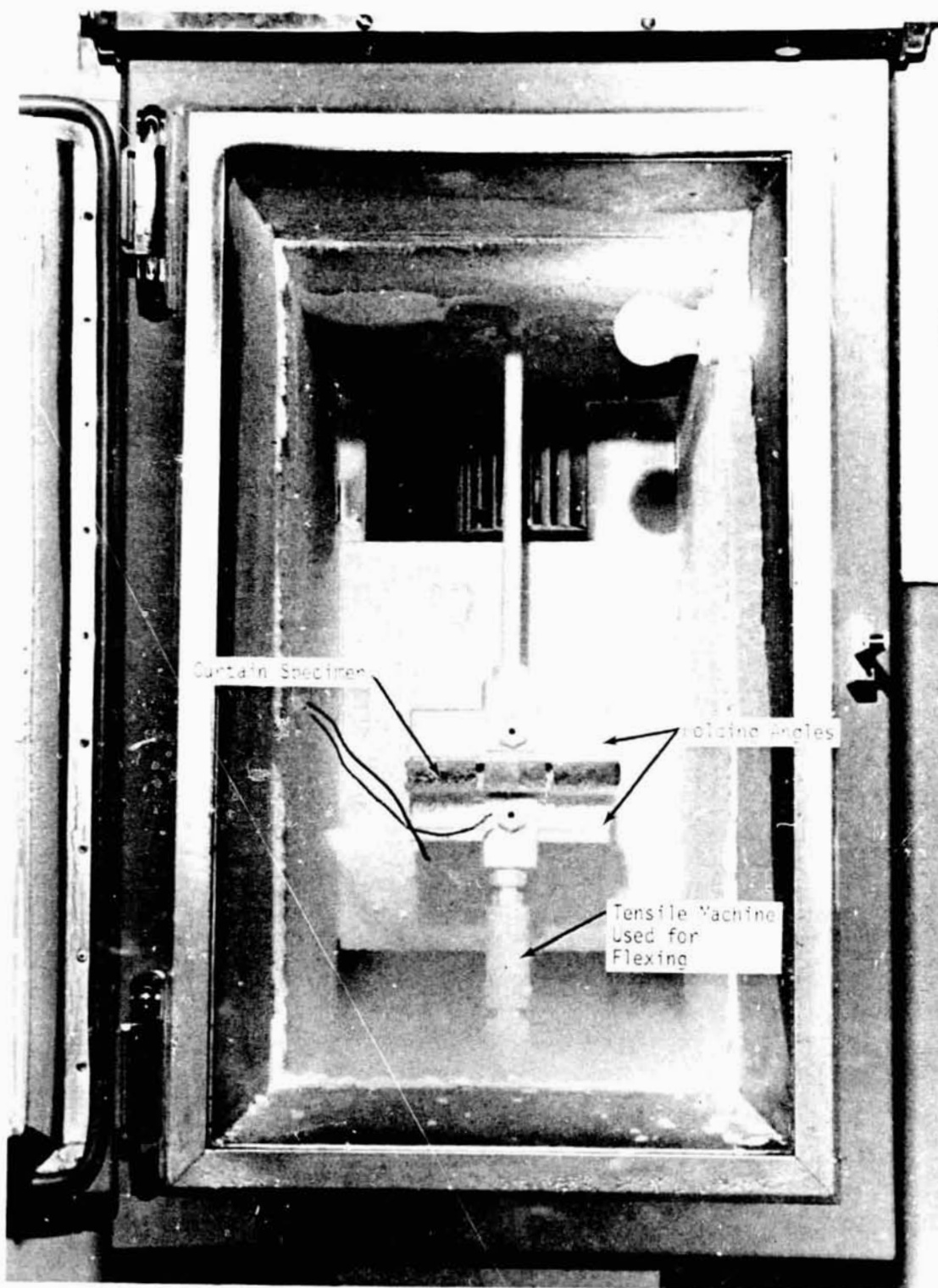
Fig. 38 Curtain Seal Materials in -200^{\circ}\text{F} Cold Soak
