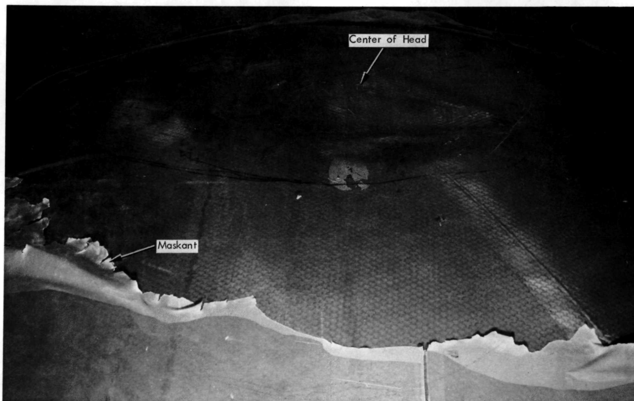
b: Buckled area with maskant removed
