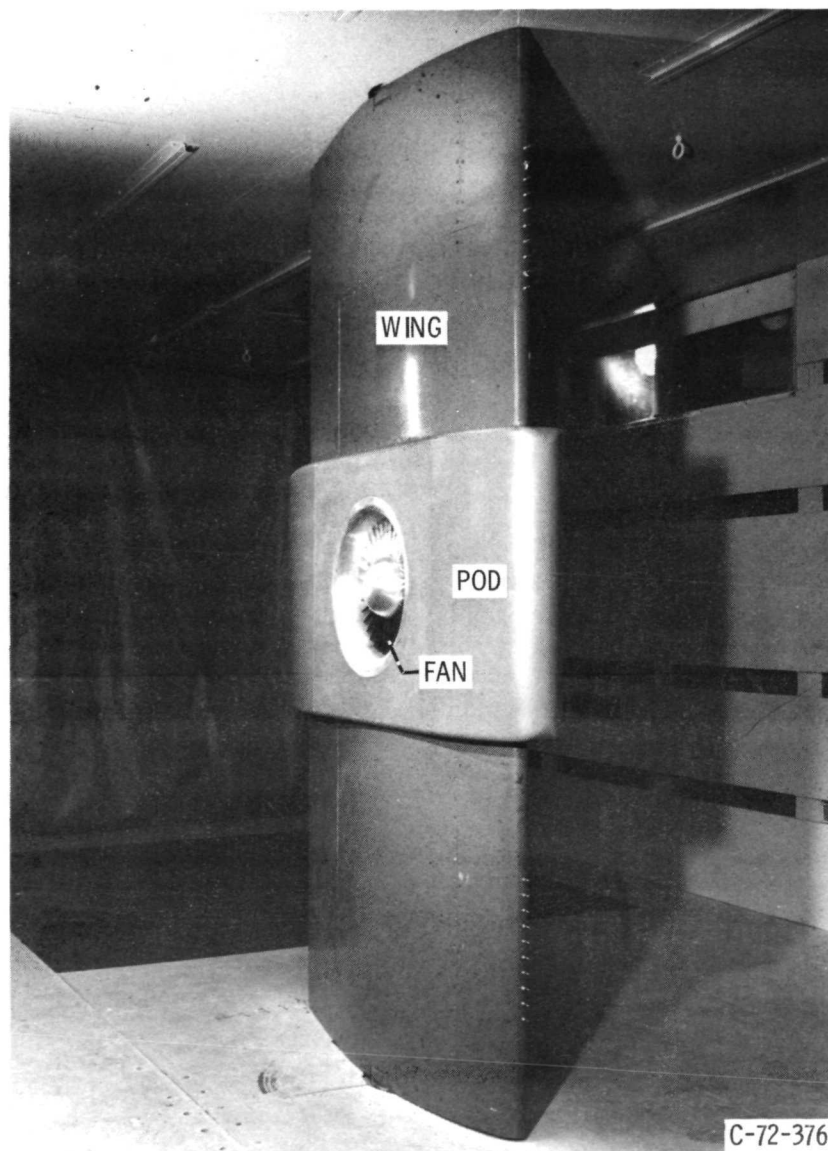
Figure 3. - Fifteen-inch fan-in-pod installed in the Lewis Research Center 9- by 15-foot V/STOL propulsion test section.
