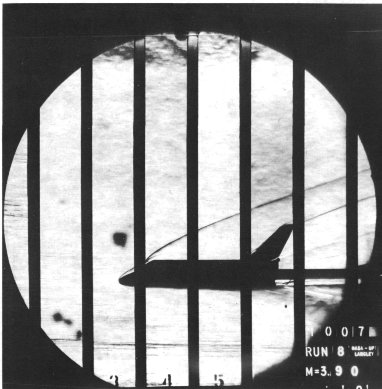
Figure 9.- Schlieren photograph of model. M = 3.90 ; \alpha = 0^\circ .
