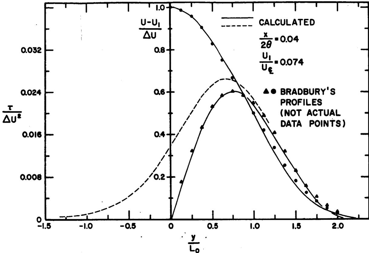
Figure 7.- Two-dimensional jet with small external flow.
