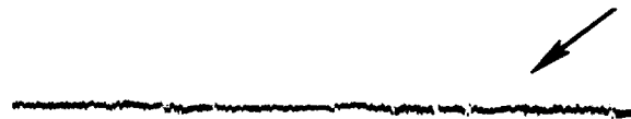
FIGURE 8-39.—Typical magnetic field perturbation scan recording of a ball bearing ring showing a "signature" which was correlated with a subsurface nonmetallic inclusion.
