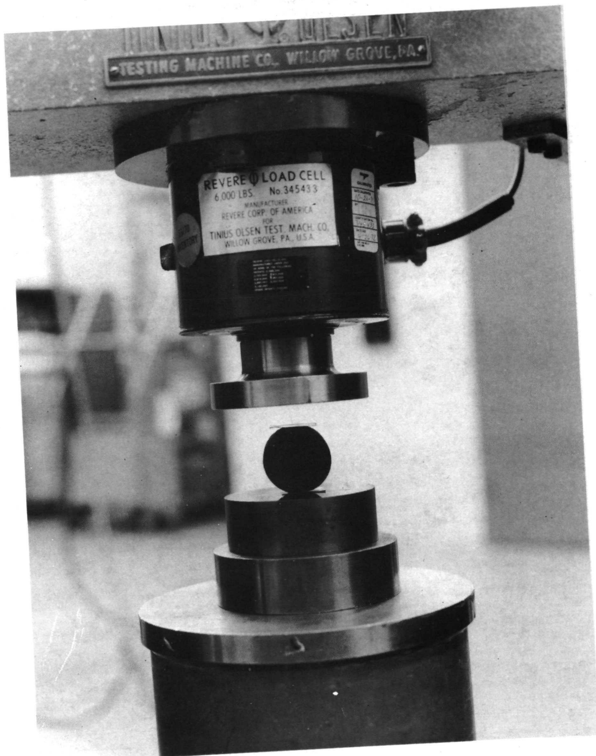
Fig. 54 Close-up of Diametral Compression Fixture. Brass pads atop and under specimen ease transition of loading from machine platens to specimen.
