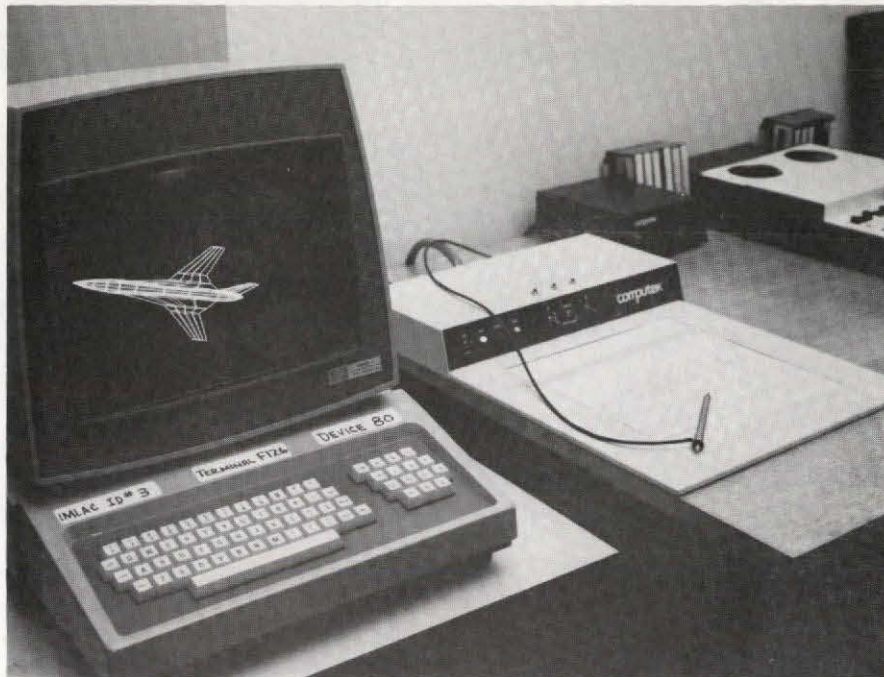
Figure 12.- Computer terminal with CRT, keyboard and digitizing tablet.
