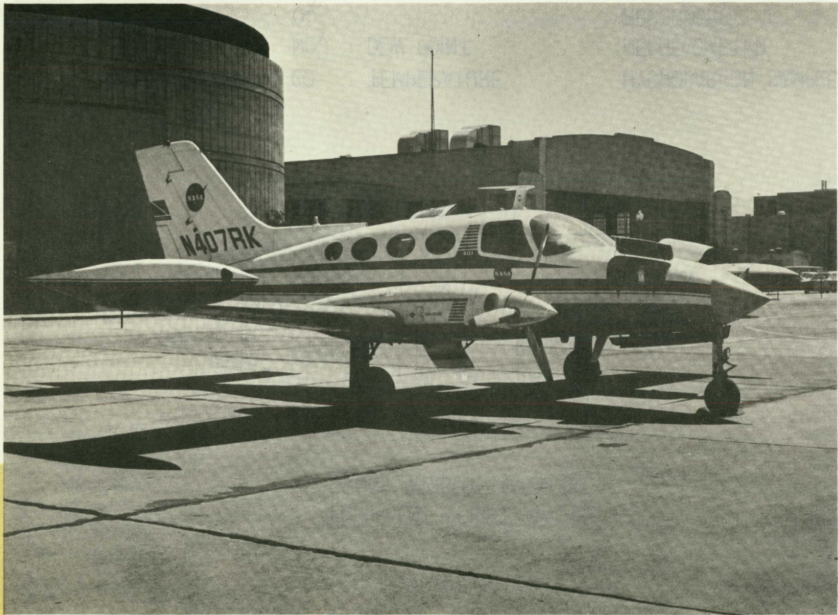
Figure 1. Cessna 401-A, twin-engine aircraft modified for air pollution sampling
