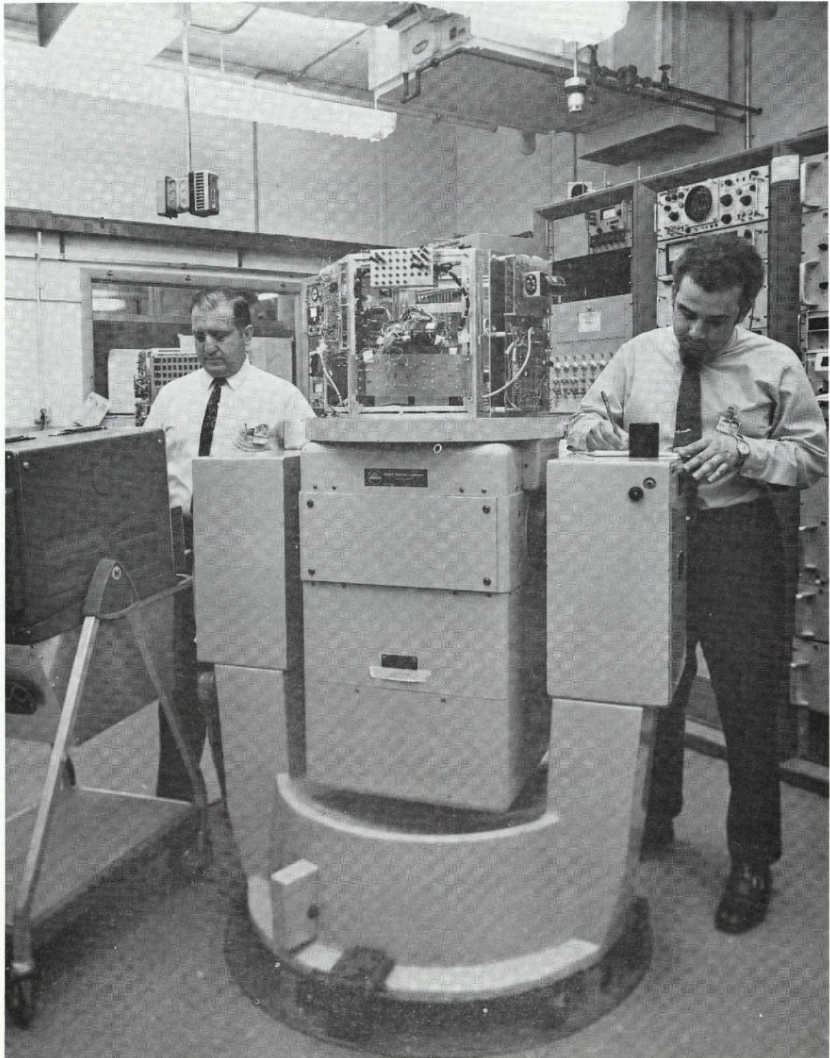
Fig. 5.1 Gyro Module Component Testing
