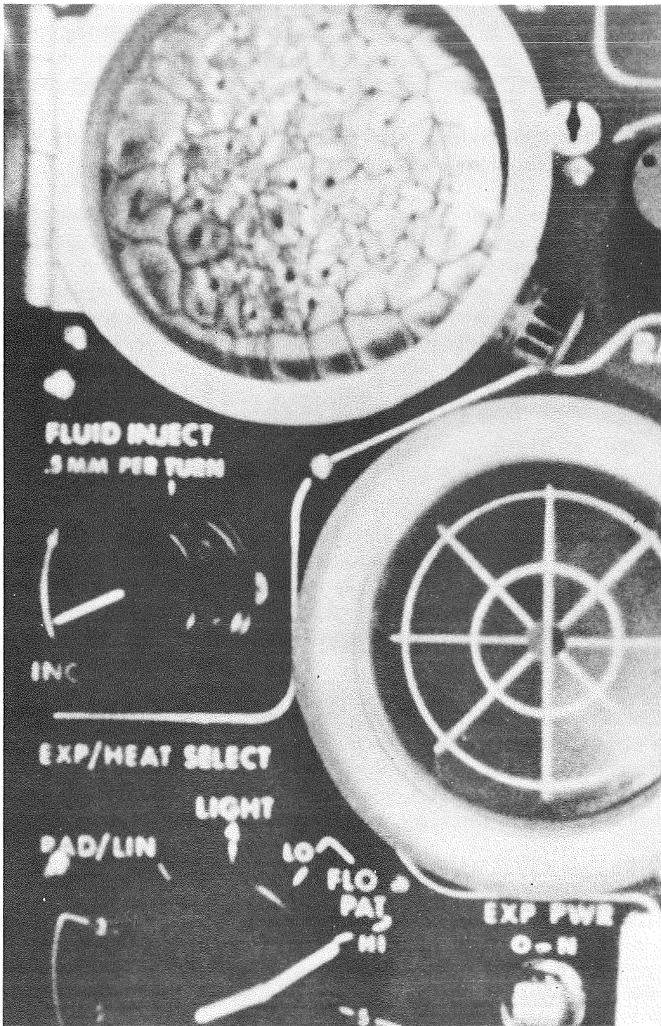
Figure 7. Convection cells obtained in 2-mm deep oil during Apollo 17 flight (14 min 19 sec after convection onset, 7.5-W heating rate).
