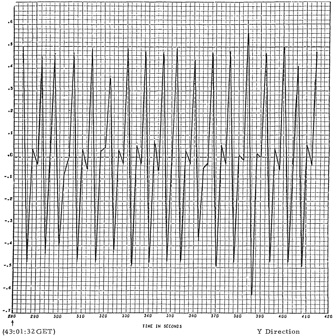
Figure 4c. Gravity level in y direction of the HFC apparatus.
