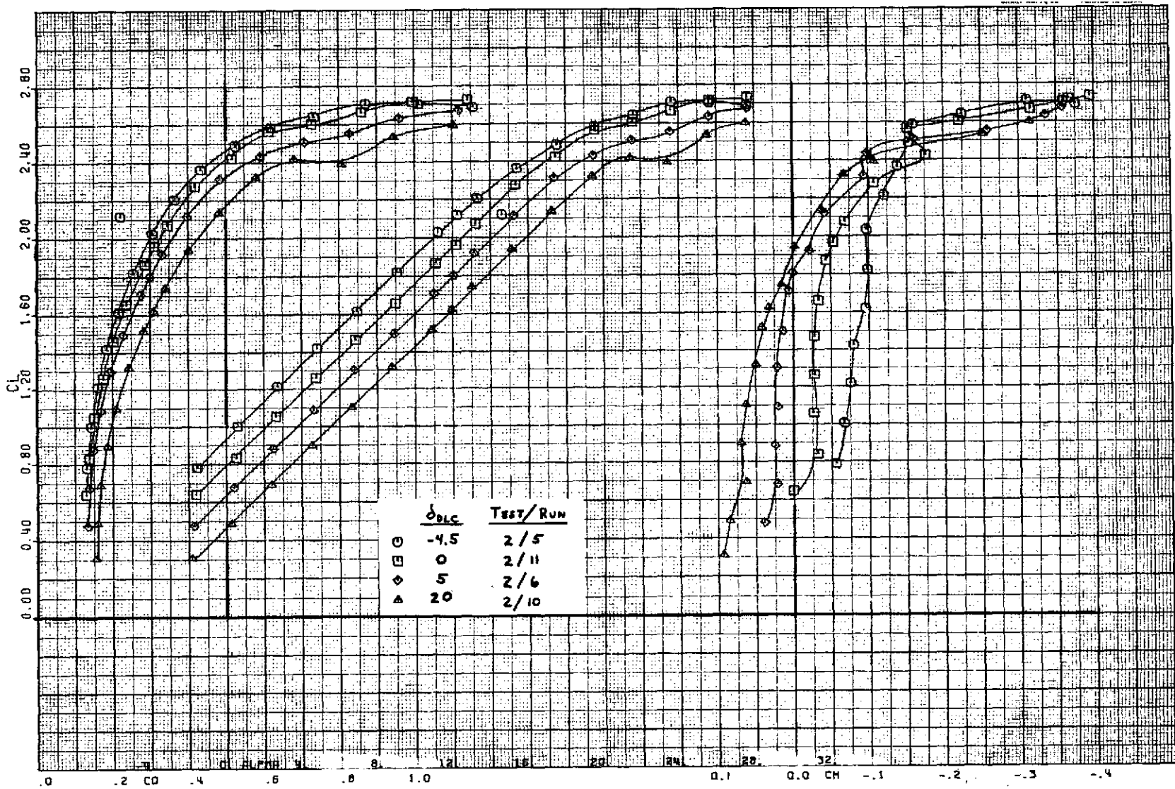
Figure 12.- Effect of direct lift control (spoilers).
