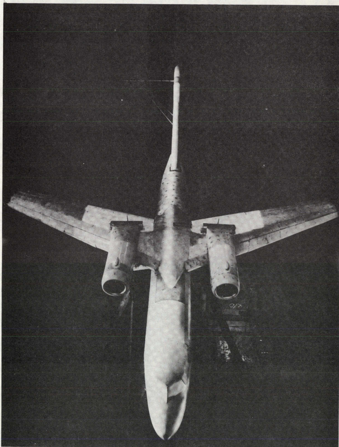
Figure 1.— Photograph of the model as mounted in the the Ames 40- by 80-Foot Wind Tunnel.
