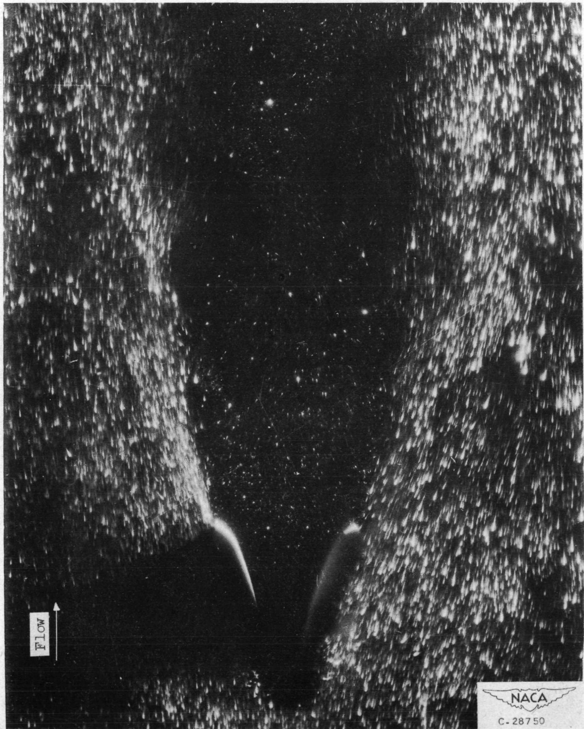
Figure 1. - Recirculation behind flame-holder model; approach air-stream velocity, approximately 50 feet per second.
