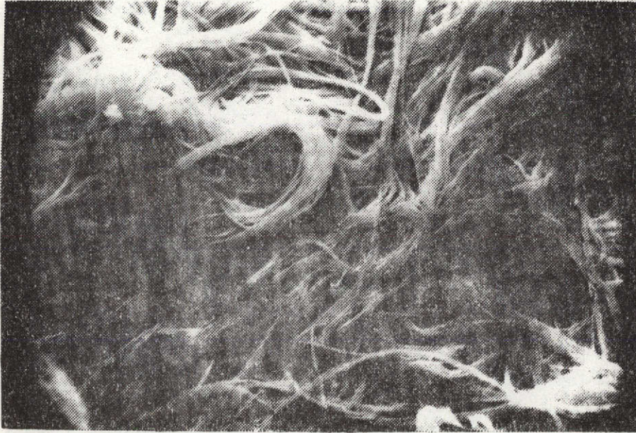
Asbestos-1 (John Mansville) 1800X
