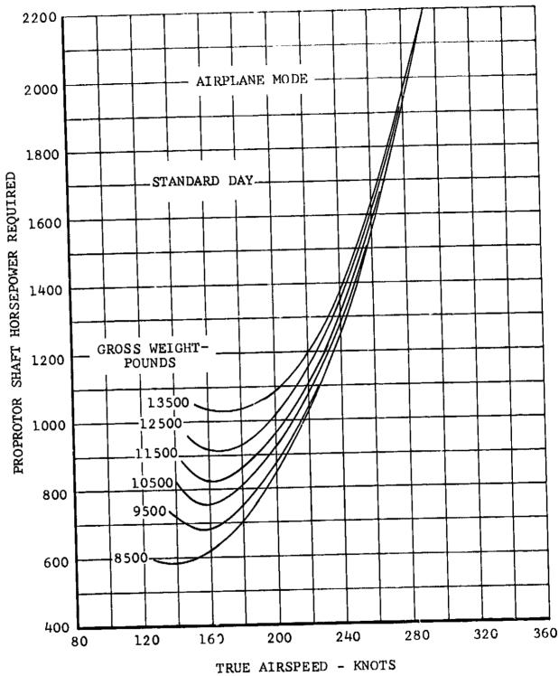
Figure V-29. Proprotor Shaft Horsepower Required Versus True Airspeed, Airplane Mode, Sea Level.
