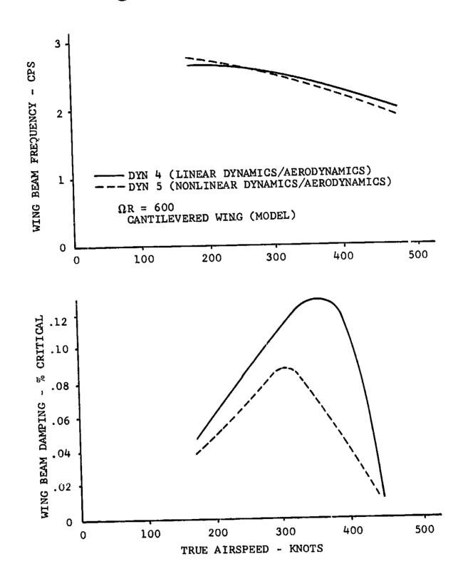
Figure VI-16. Comparison of Stability Analysis Method.
