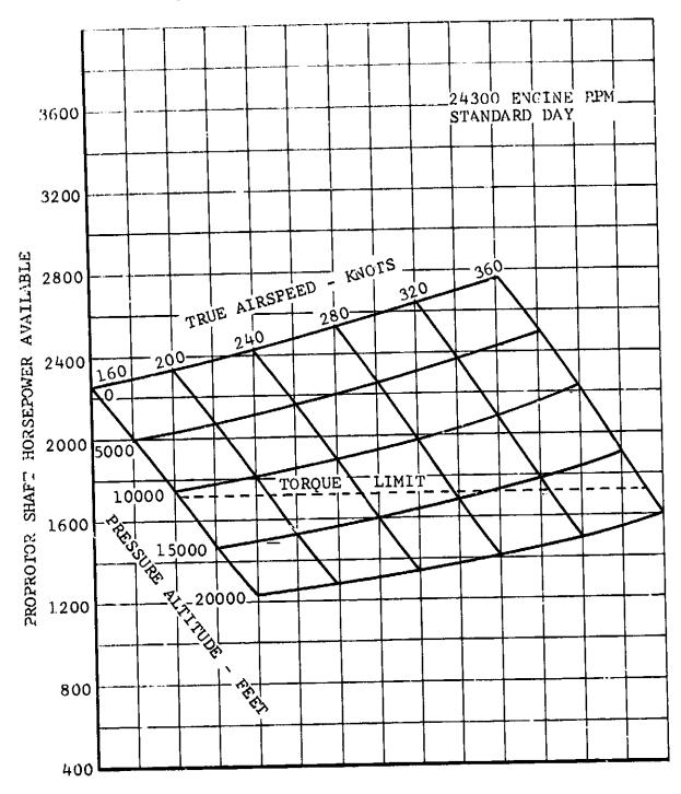
Figure V-18. Proprotor Shaft Horsepower Available, Takeoff and 30-Minute Power.
