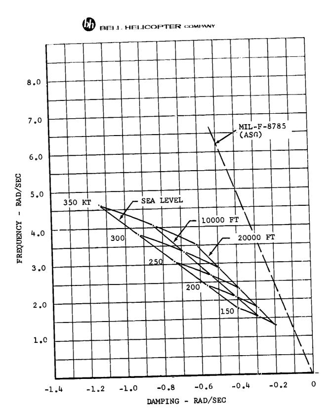
Figure VI-23. Root Locus of Dutch-Roll Mode for Basic Airframe.
