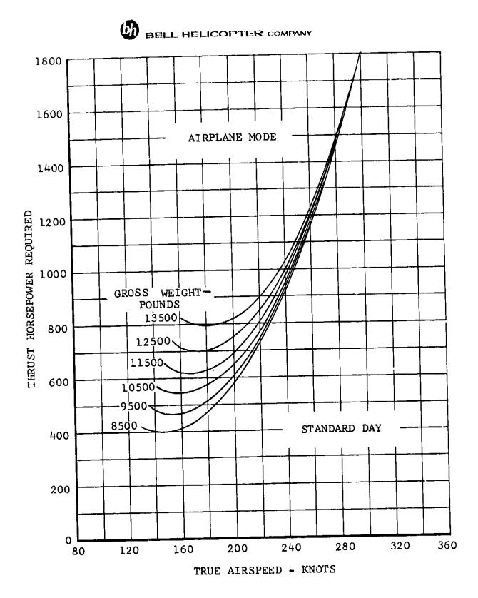
Figure V-26. Thrust Horsepower Required Versus True Airspeed, Sea Level.
