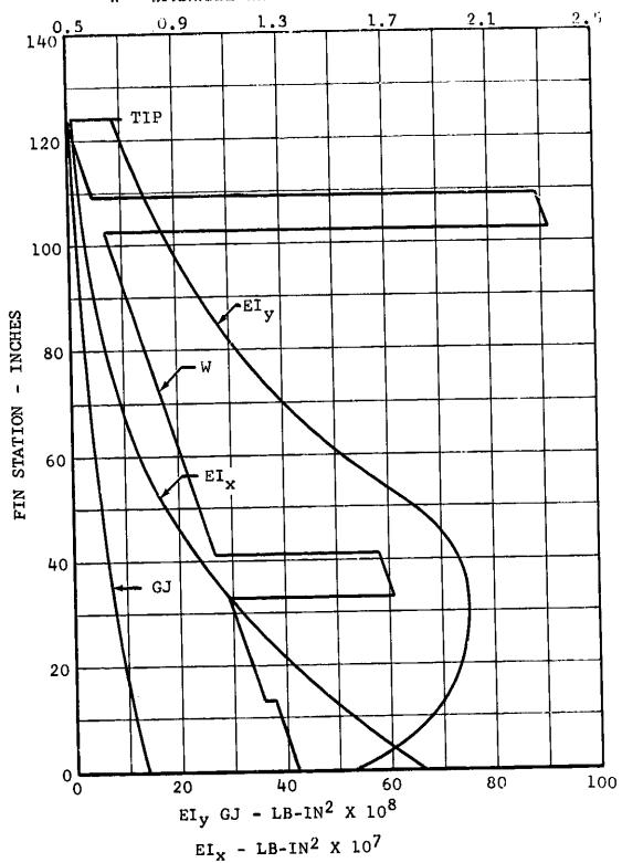
Figure III-5. Vertical Tail Stiffness and Weight Distribution.
