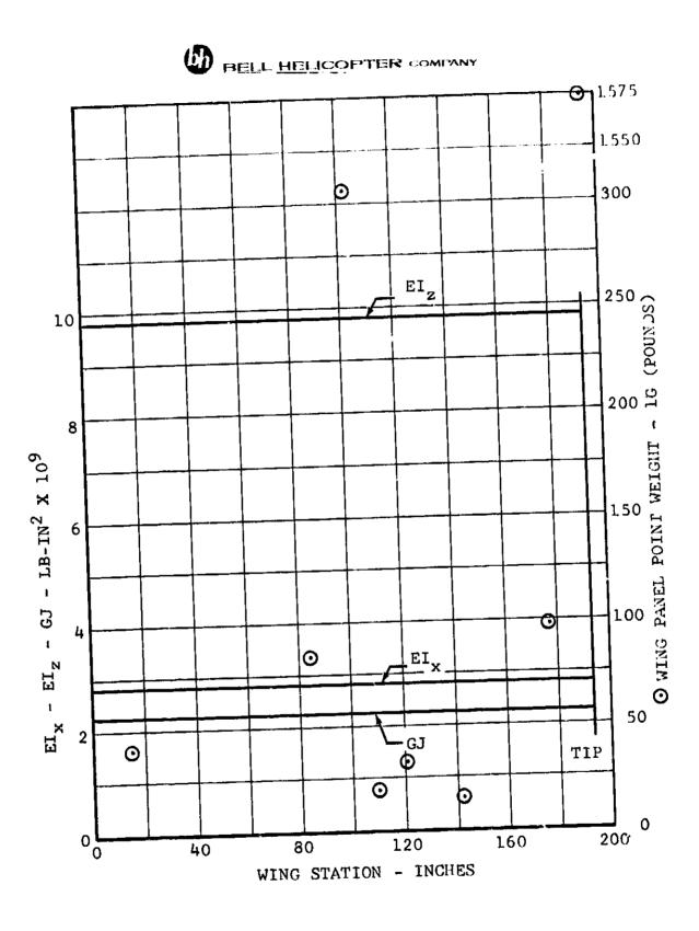
Figure III-3. Wing Stiffness and Panel Point Weight.
