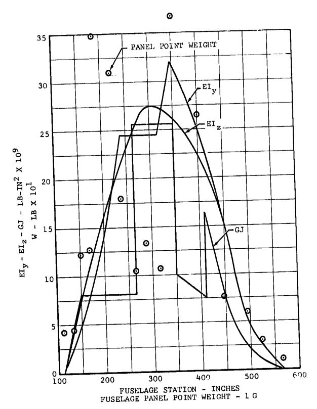
Figure III-4. Fuselage Stiffness and Panel Point Weight.
