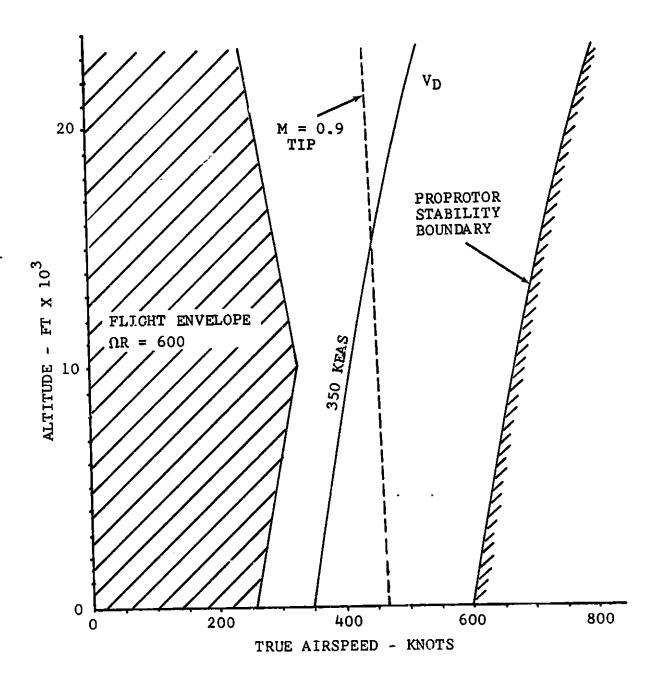
Figure VI-11. Model 300 Proprotor Stability Boundary.
