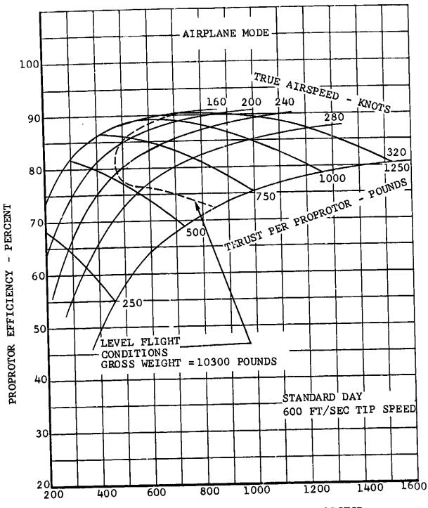
PROPROTOR SHAFT HORSEPOWER PER PROPROTOR
