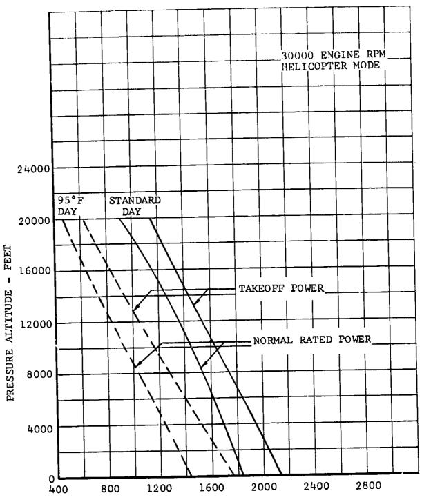
TOTAL PROPROTOR HORSEPOWER AVAILABLE
