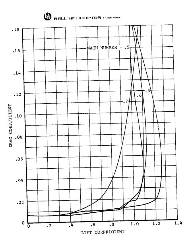
Figure V-8. Proprotor Blade Station Data, Radial Station 0.70 to 0.90.
