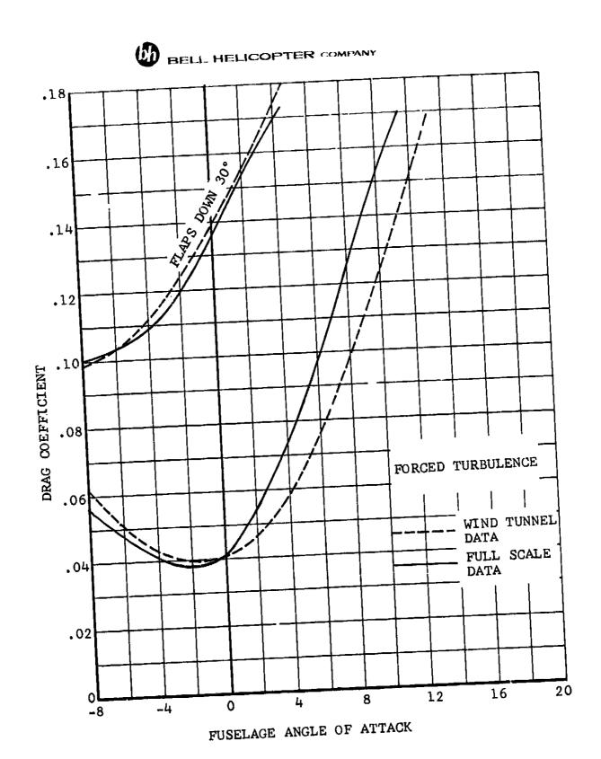
Figure V-3. Airframe Drag Coefficient Versus Fuselage Angle of Attack.
