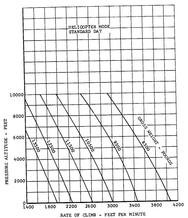
Figure V-25. Rate of Climb, Helicopter Mode.
