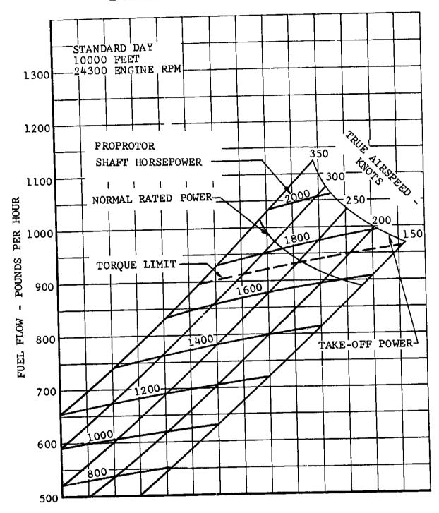
Figure V-20. Fuel Flow, Airplane Mode.
