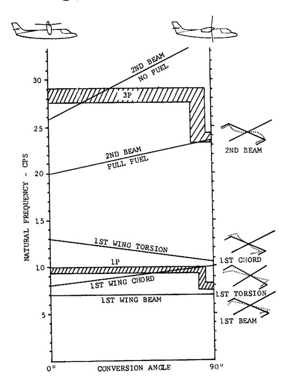
Figure VI-7. Airframe Asymmetric Mode Natural Frequencies.
