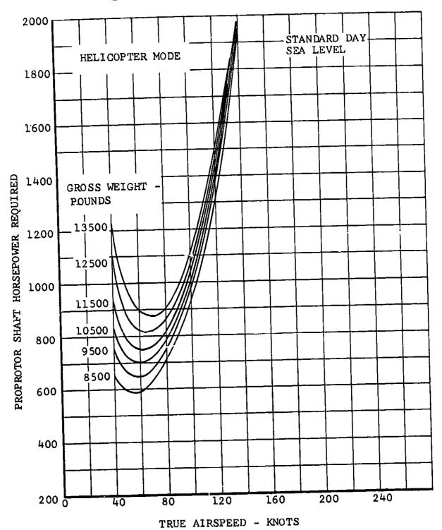
Figure V-23. Proprotor Shaft Horsepower Required Versus True Airspeed, Helicopter Mode.
