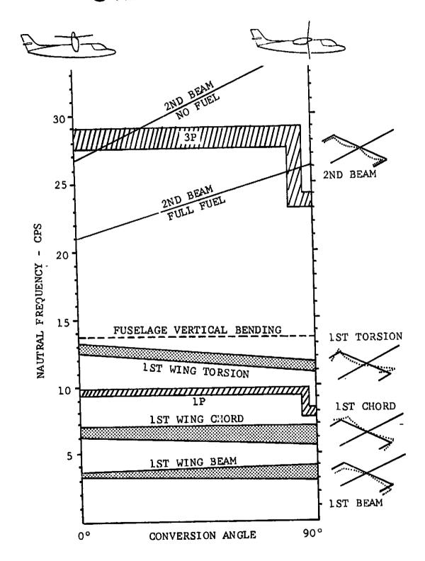
Figure VI-6. Airframe Symmetric Mode Natural Frequencies.
