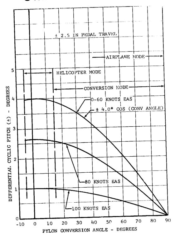
Figure III-10. Differential Cyclic Pitch Versus Conversion Angle.
