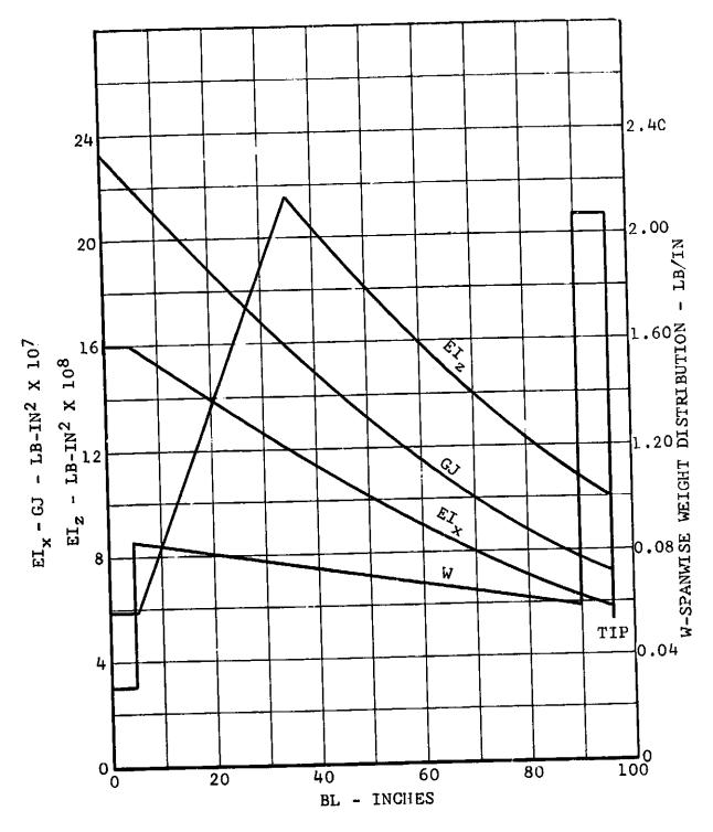
Figure III-6. Horizontal Tail Stiffness and Weight Distribution.
