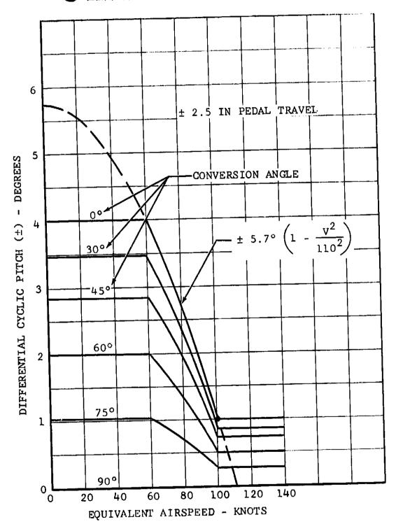
Figure III-11. Differential Cyclic Pitch Versus Airspeed.
