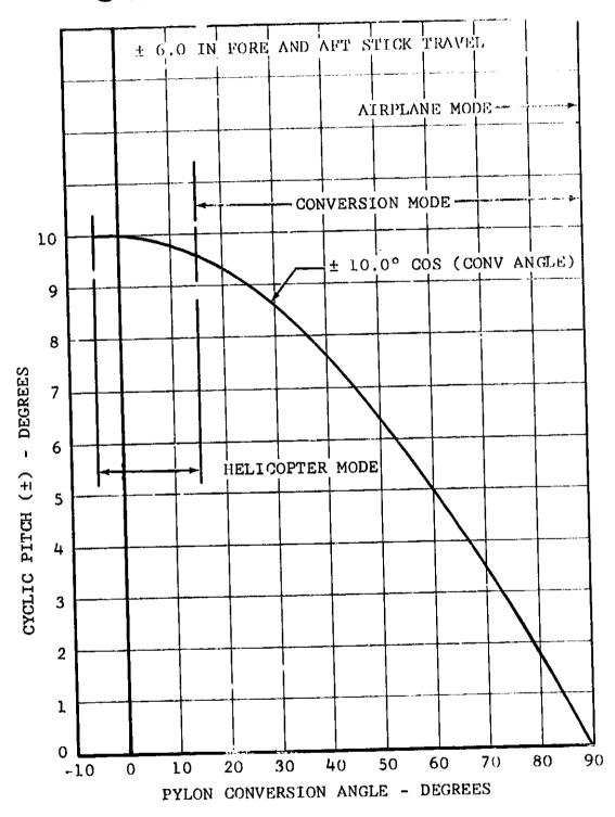
Figure II1-9. Fore and Aft Cyclic Pitch Versus Conversion Angle.
