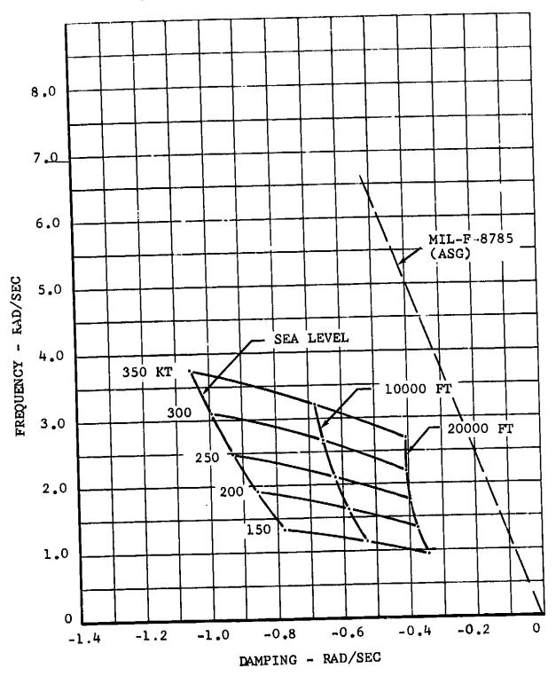
Figure VI=22. Root Locus of Dutch-Roll Mode.
