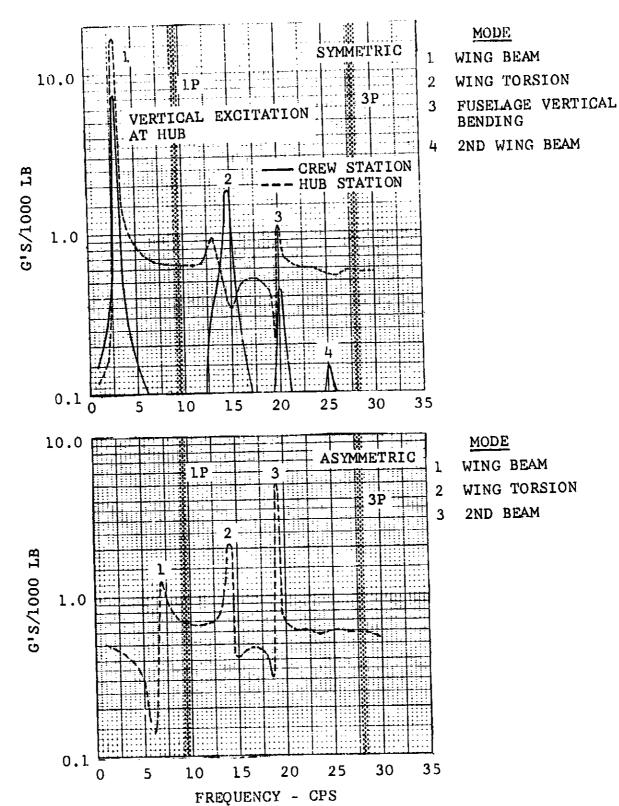
Figure VI-9. Pylon and Crew Station Frequency Response, Helicopter Mode.
