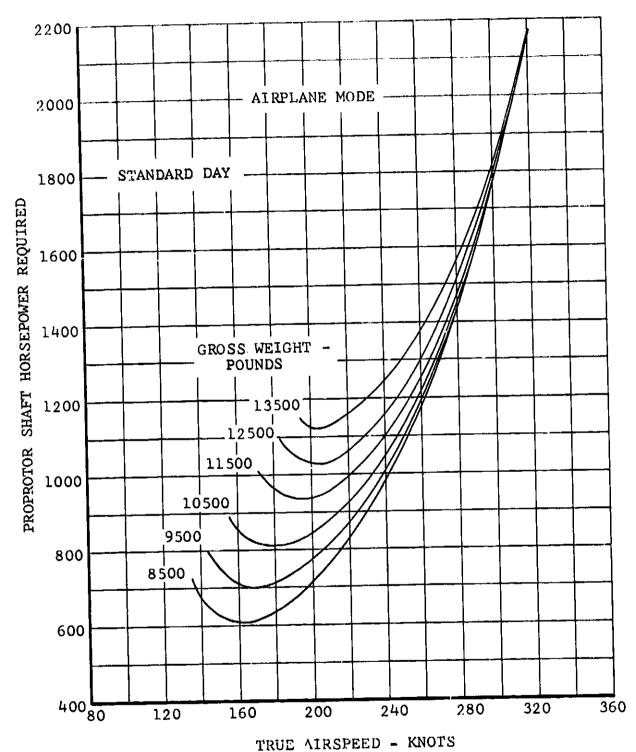
Figure V-30. Proprotor Shaft Horsepower Required Versus True Airspeed, Airplane Mode, 10,000 Feet.
