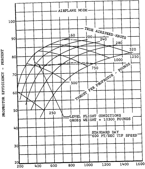
PROPROTOR SHAFT HORSEPOWER PER PROPROTOR
