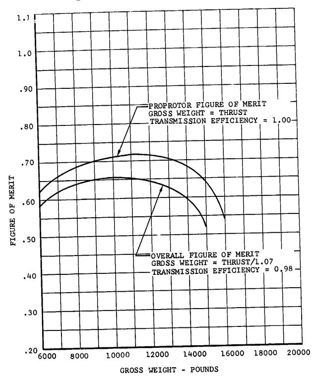
Figure V-22. Hovering Figure of Merit.
