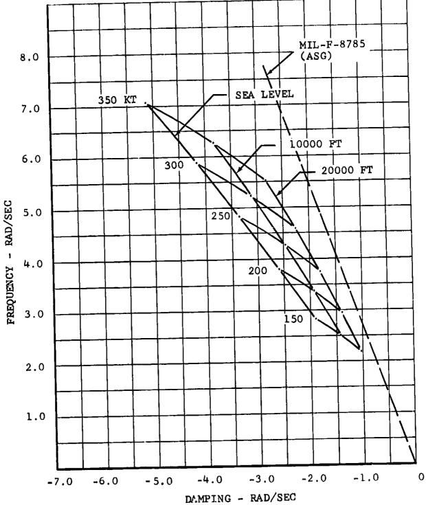
Figure VI-21. Root Locus of Longitudinal Short-Period Mode of Basic Airframe.
