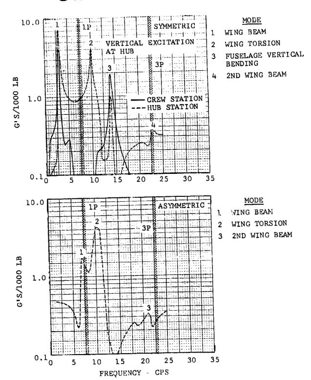
Figure VI-10. Pylon and Crew Station Frequency Response, Airplane Mode.
