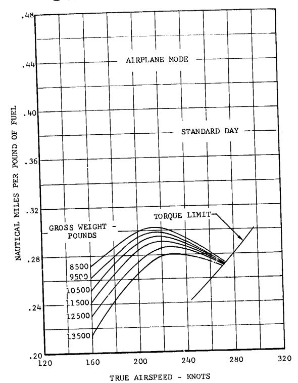
Figure V-34. Nautical Miles Per Pound of Fuel Versus True Airspeed, Airplane Mode, Sea Level.
