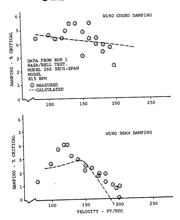
Figure VI-12. Correlation of Calculated and Measured Proprotor Stability - NASA-Bell Test of Model 266 Aeroelastic Model.
