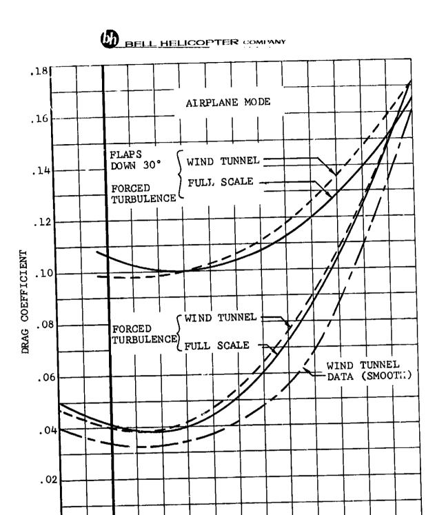
Figure V-4. Airframe Drag Coefficient Versus Lift Coefficient.
