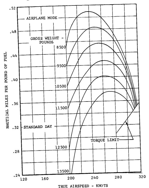
Figure V-36. Nautical Miles Per Pound of Fuel Versus True Airspeed, Airplane Mode, 20,000 Feet.
