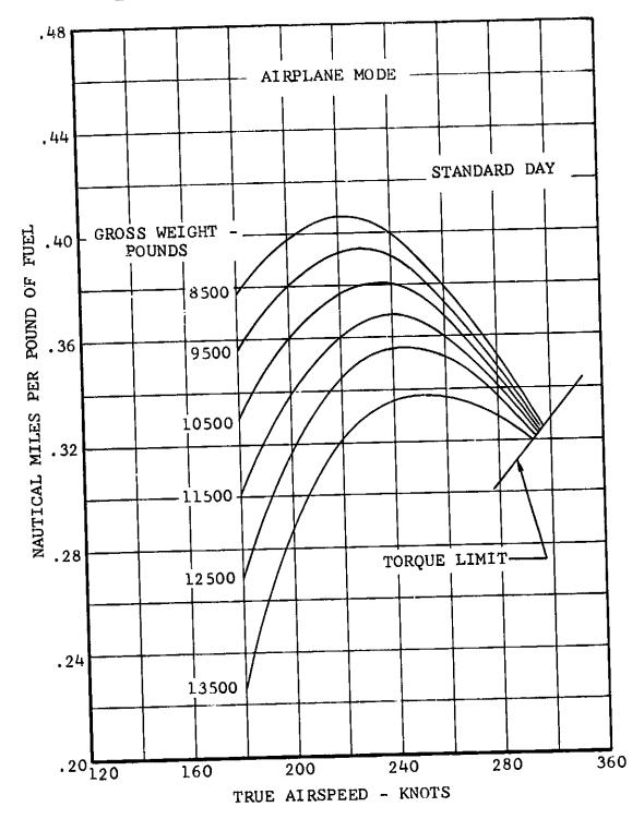
Figure V-35. Nautical Miles Per Pound of Fuel Versus True Airspeed, Airplane Mode, 10,000 Feet.
