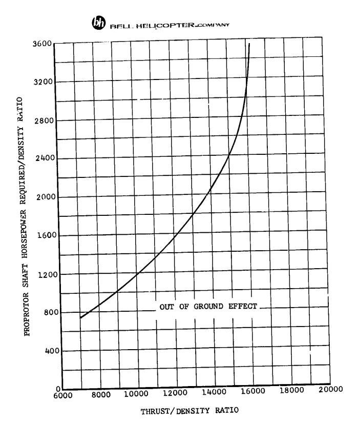
Figure V-12. Proprotor Hovering Power Required Versus Thrust.
