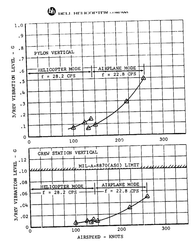
Figure VI-8. Pylon and Crew Station Vibration.
