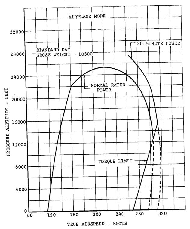
Figure V-32. Flight Envelope and Maximum Speed, Airplane Mode.
