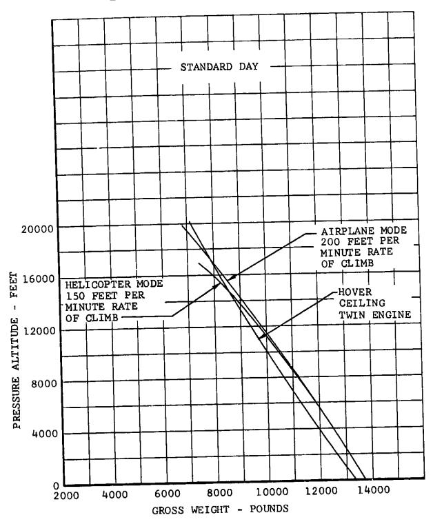
Figure V-37. Single Engine Performance.
