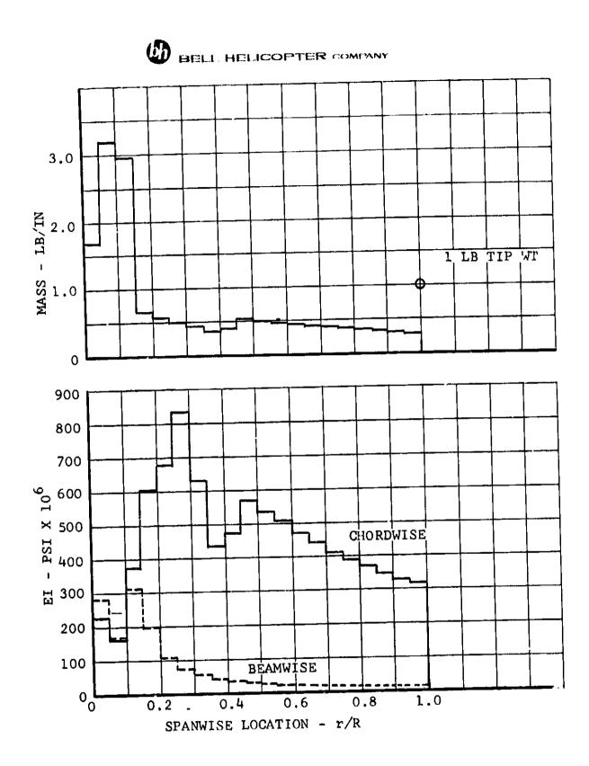
Figure III-2. Proprotor Stiffness and Mass Distribution.
