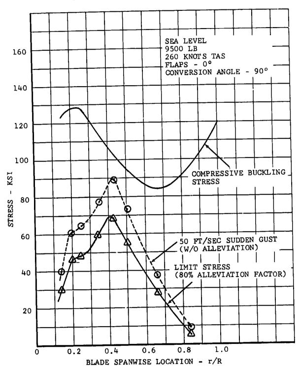
Figure VI=4. Blade Limit Stress at  $V_H$ , Airplane Mode.
