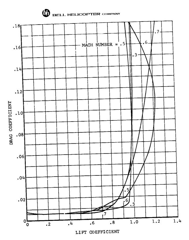
Figure V-9. Proprotor Blade Section Data, Radial Station 0.90 to 1.00.
