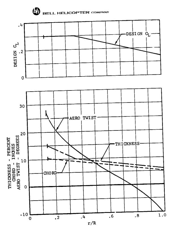
Figure V-11. Boeing-Vertol 13-Foot Diameter Proprotor Blade Parameters (Blade "E").
