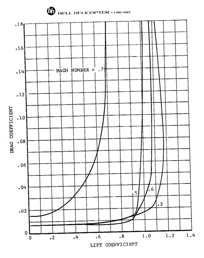
Figure V-7. Proprotor Blade Section Data Blade Station 0.45 to 0.70.
