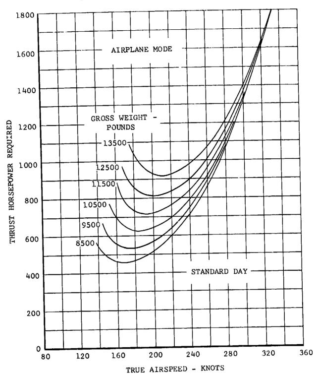
Figure V-27. Thrust Horsepower Required Versus True Airspeed, 10,000 Feet.
