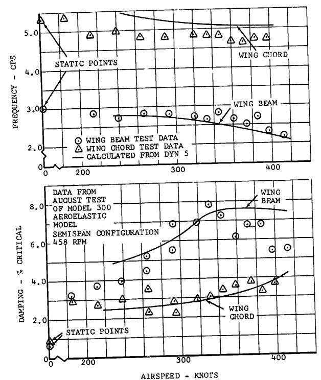
Figure VI-13. Model 300 Aeroelastic Model Proprotor Stability (Full-Scale Frequency and Airspeed).
