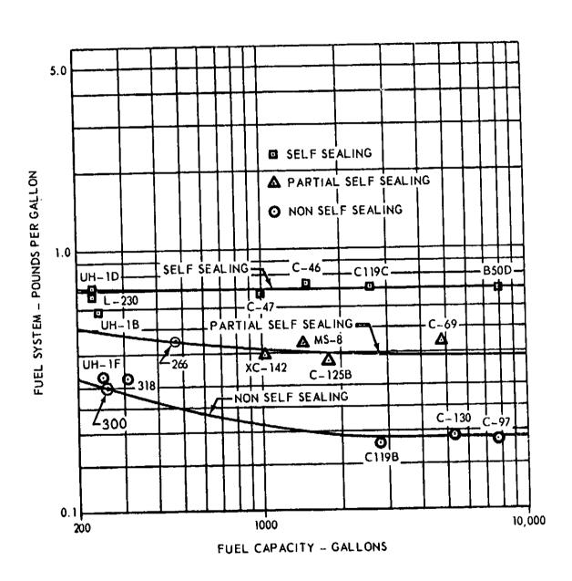
Figure IV-3. Fuel System Weight.
