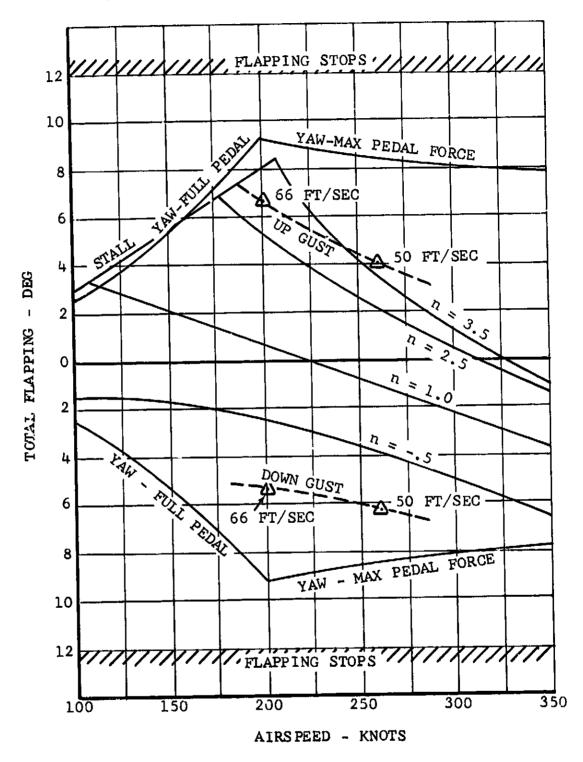
Figure VI-5. Flapping Envelope in Airplane Mode.
