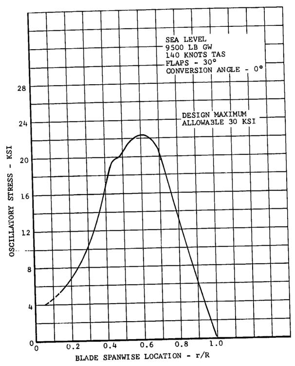
Figure VI-3. Blade Oscillatory Stress at  $V_{\rm H}$ , Helicopter Mode.
