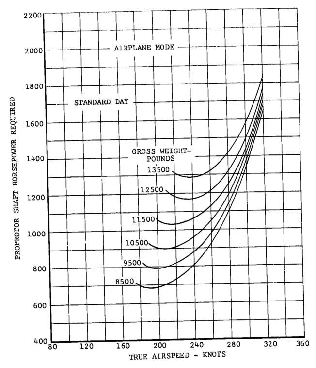
Figure V-31. Proprotor Shaft Horsepower Required Versus True Airspeed, Airplane Mode, 20,000 Feet.
