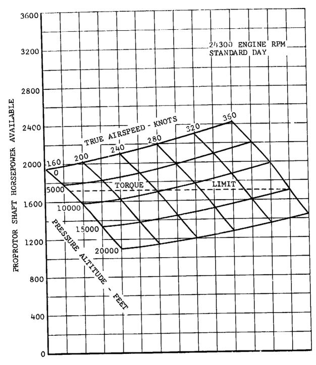
Figure V-19. Proprotor Shaft Horsepower Available, Normal Rated Power
