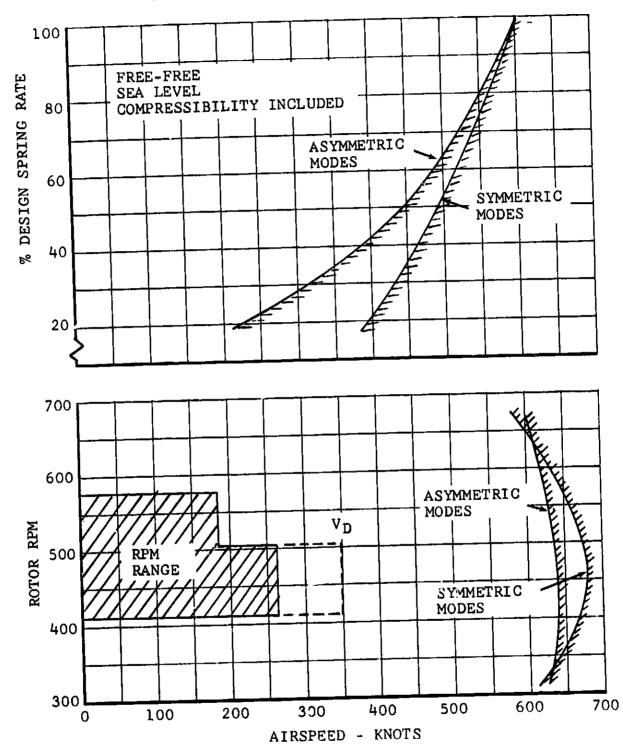
Figure VI-19. Proprotor Stability Sensitivity to Wing Stiffness and RPM.
