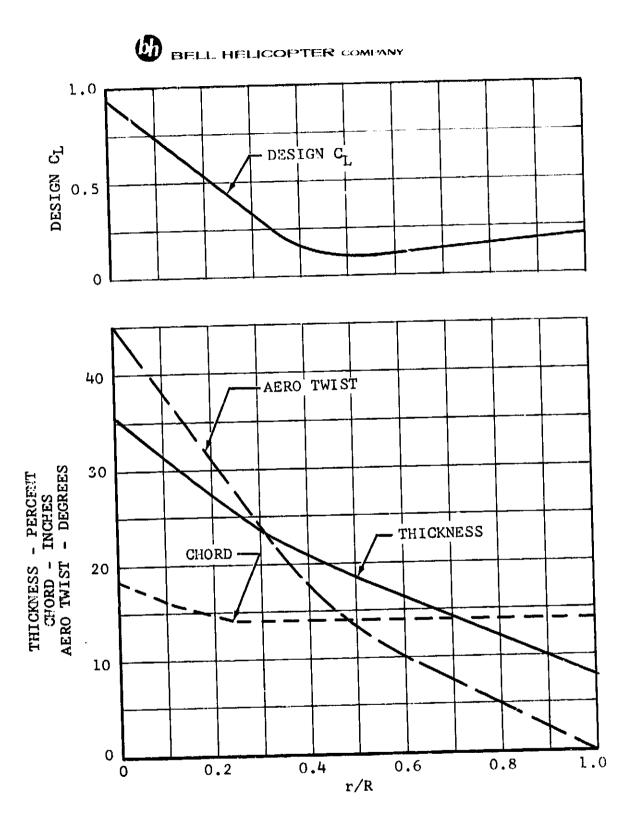
Figure III-1. 25-Foot Proprotor Parameters.
