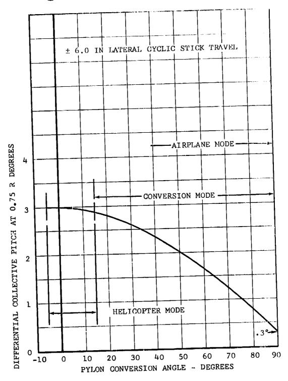
Figure III-8. Differential Collective Pitch Versus Conversion Angle.
