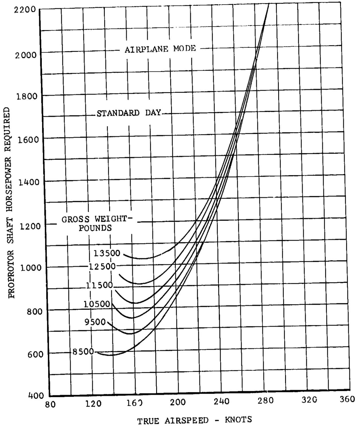
Figure V-29. Proprotor Shaft Horsepower Required Versus True Airspeed, Airplane Mode, Sea Level.
