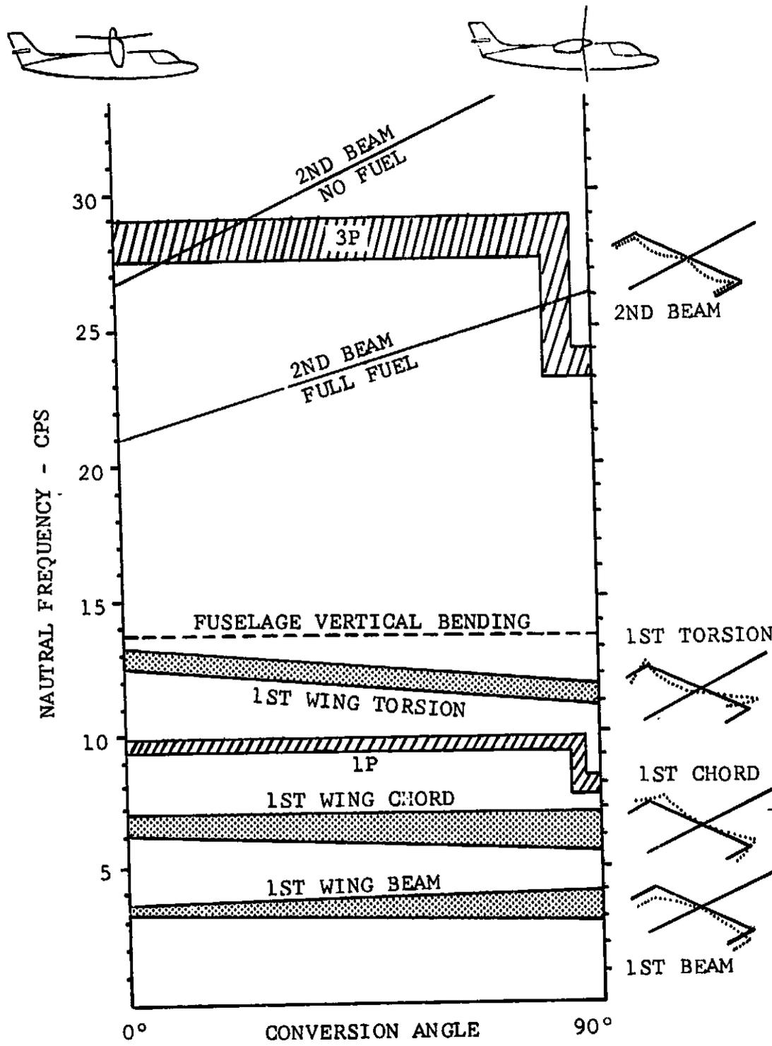
Figure VI-6. Airframe Symmetric Mode Natural Frequencies.
