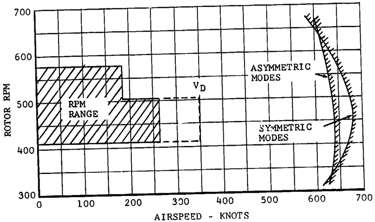
Figure VI-19. Proprotor Stability Sensitivity to Wing Stiffness and RPM.
