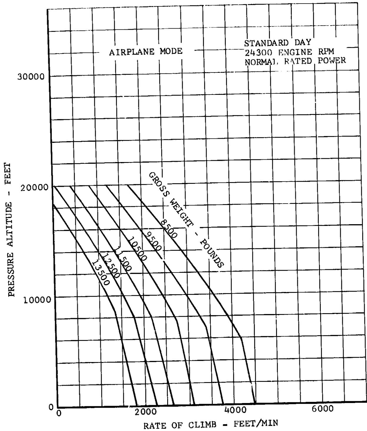
Figure V-33. Maximum Rate of Climb, Airplane Mode.
