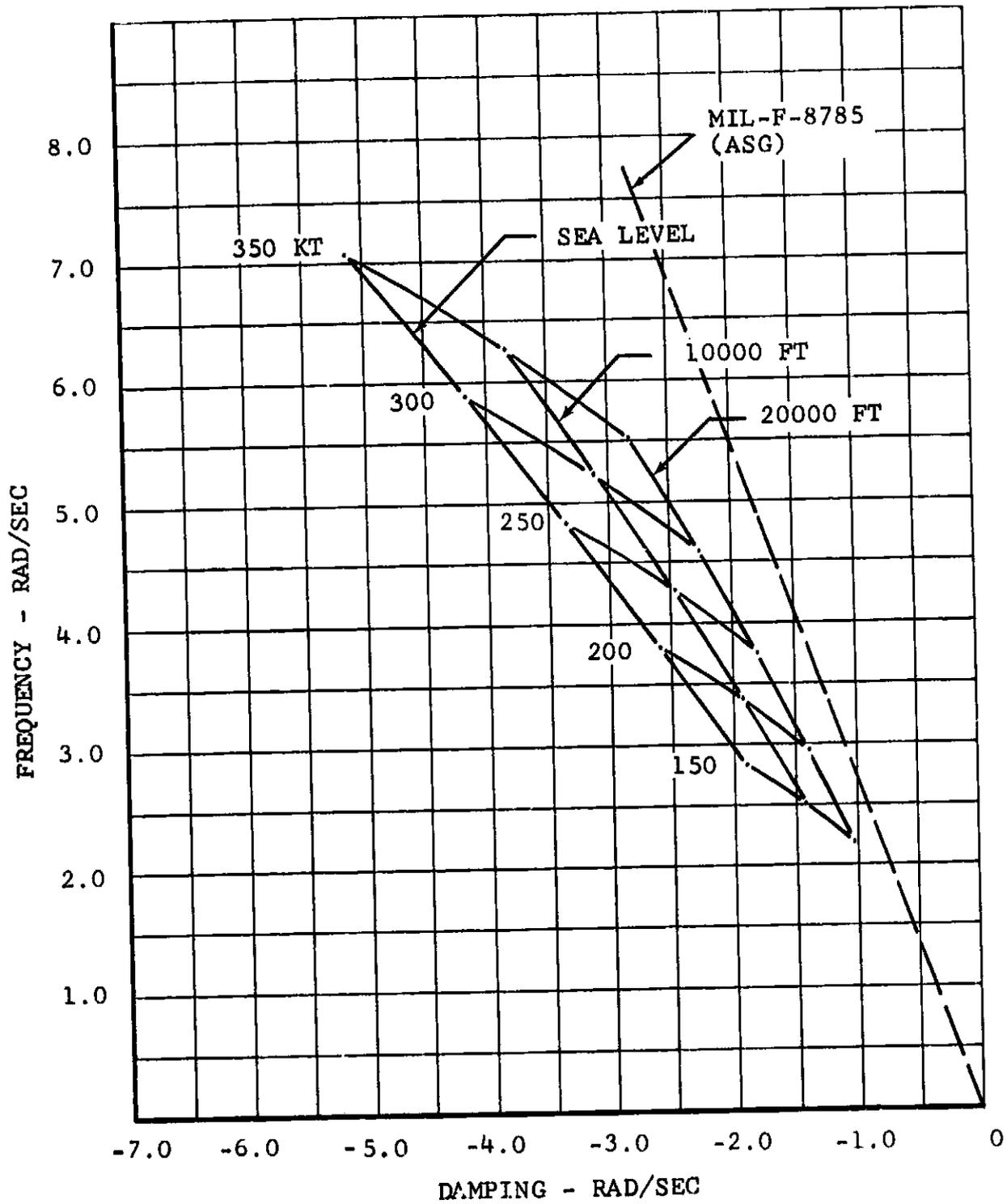
Figure VI-21. Root Locus of Longitudinal Short-Period Mode of Basic Airframe.
