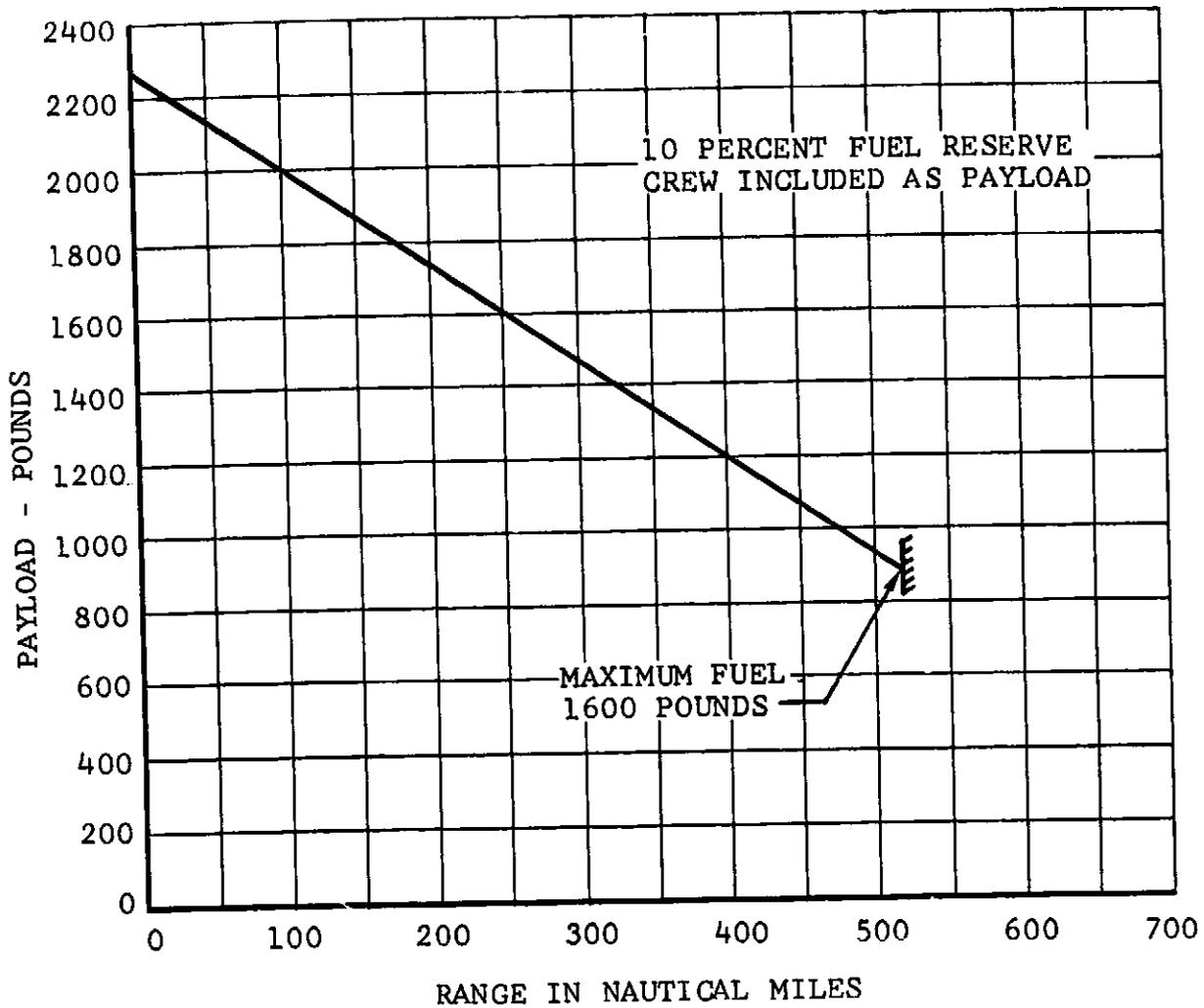
CRUISE AT  $V_{LRC} = 240$  KNOTS
