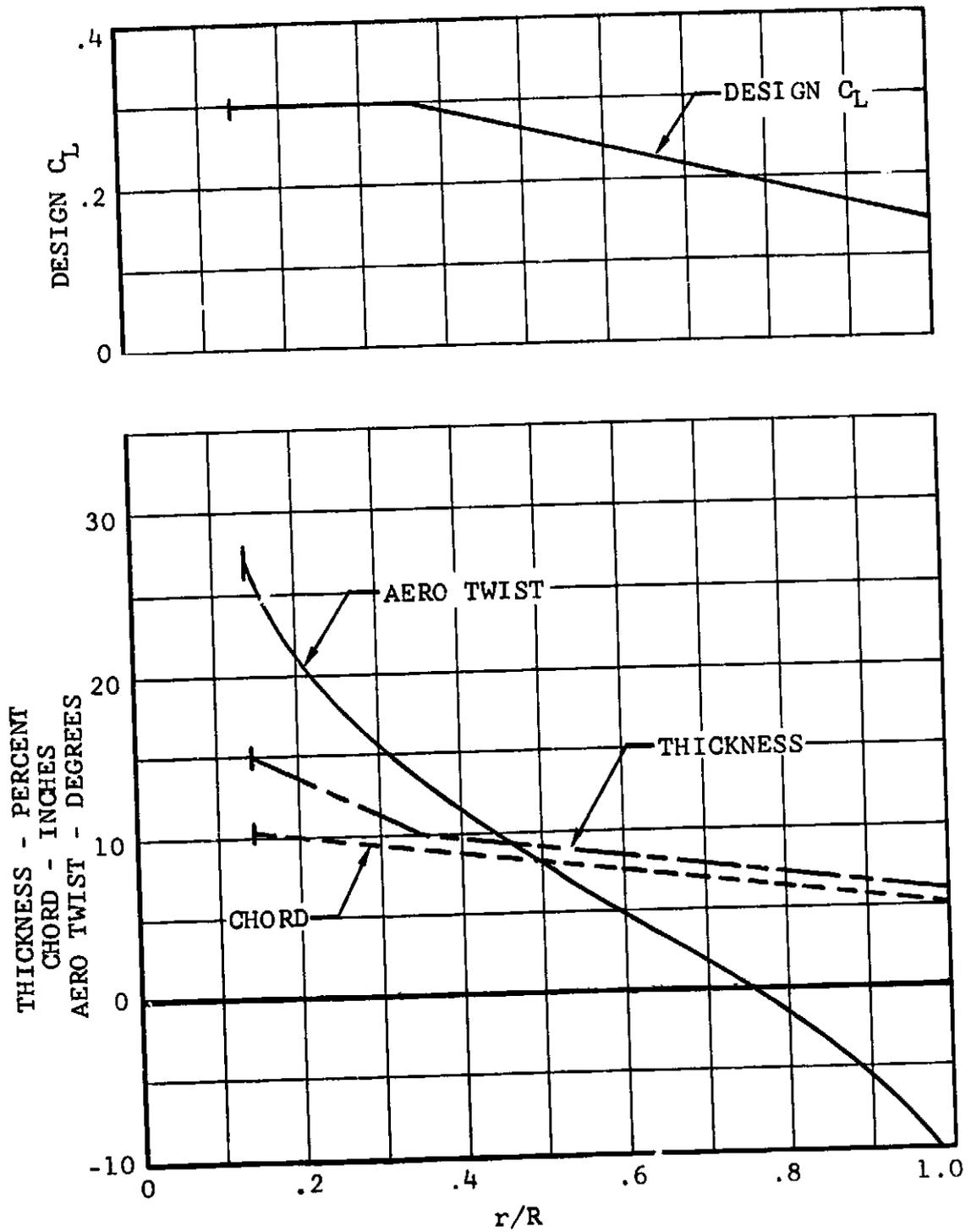
Figure V-11. Boeing-Vertol 13-Foot Diameter Proprotor Blade Parameters (Blade "E").
