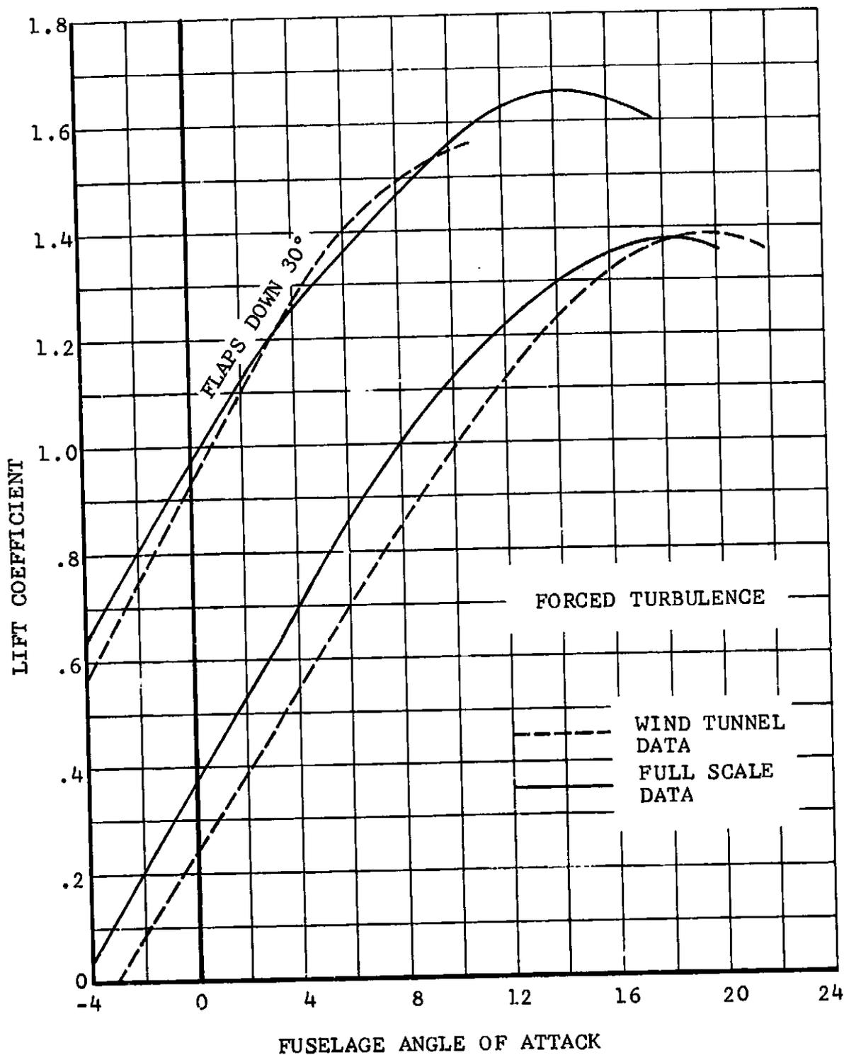
Figure V-2. Airframe Lift Coefficient Versus Fuselage Angle of Attack.
