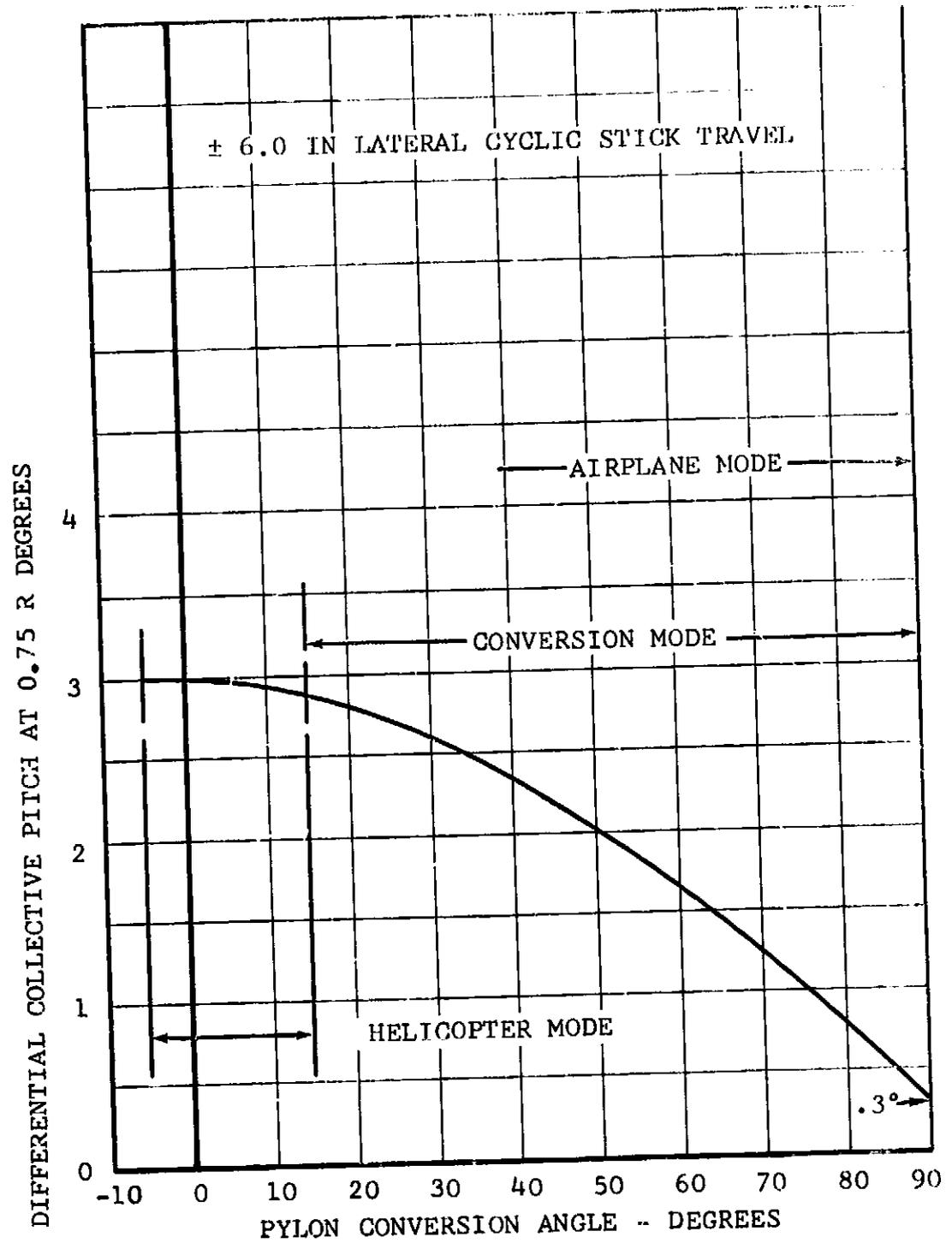
Figure III-8. Differential Collective Pitch Versus Conversion Angle.
