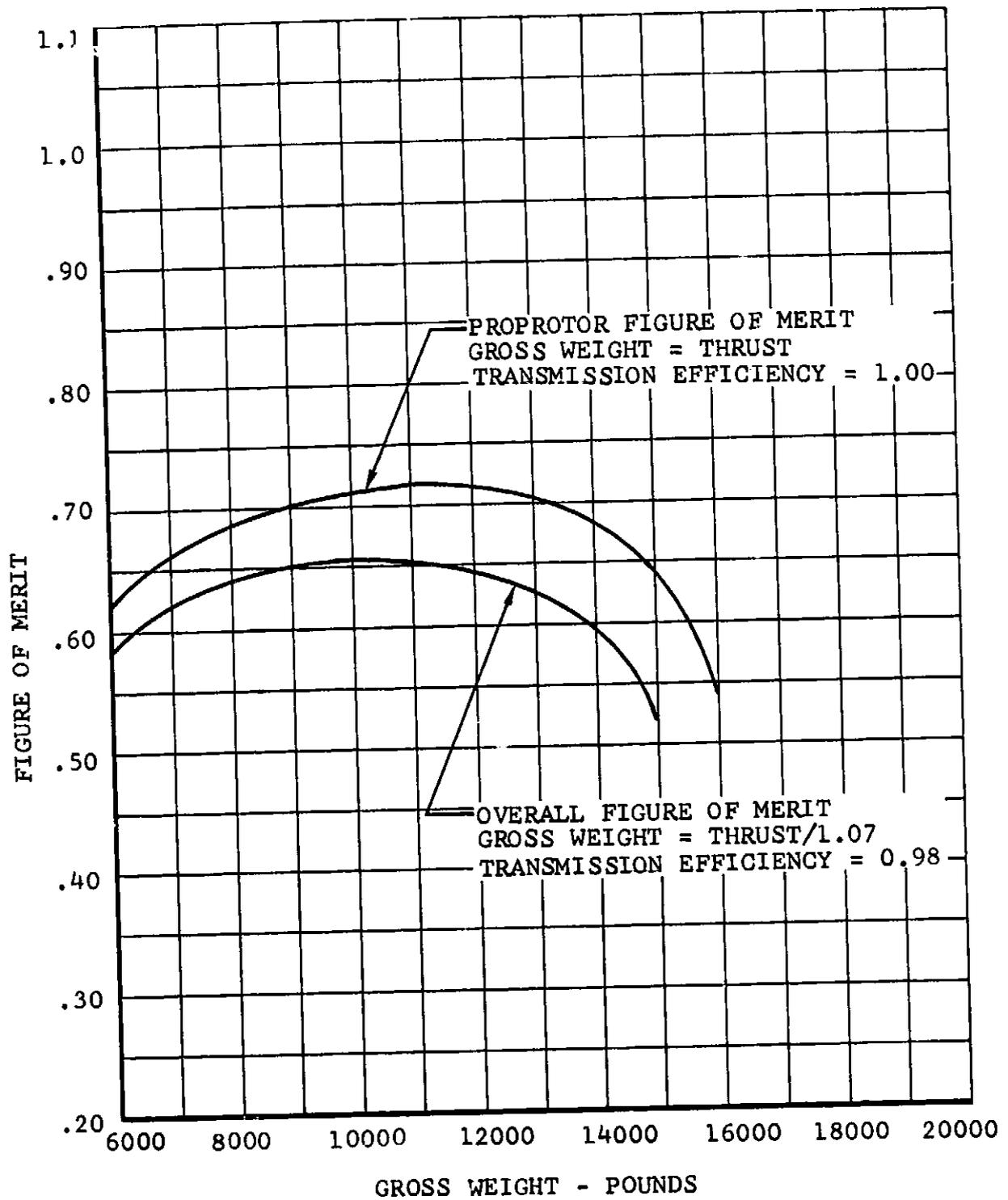
Figure V-22. Hovering Figure of Merit.
