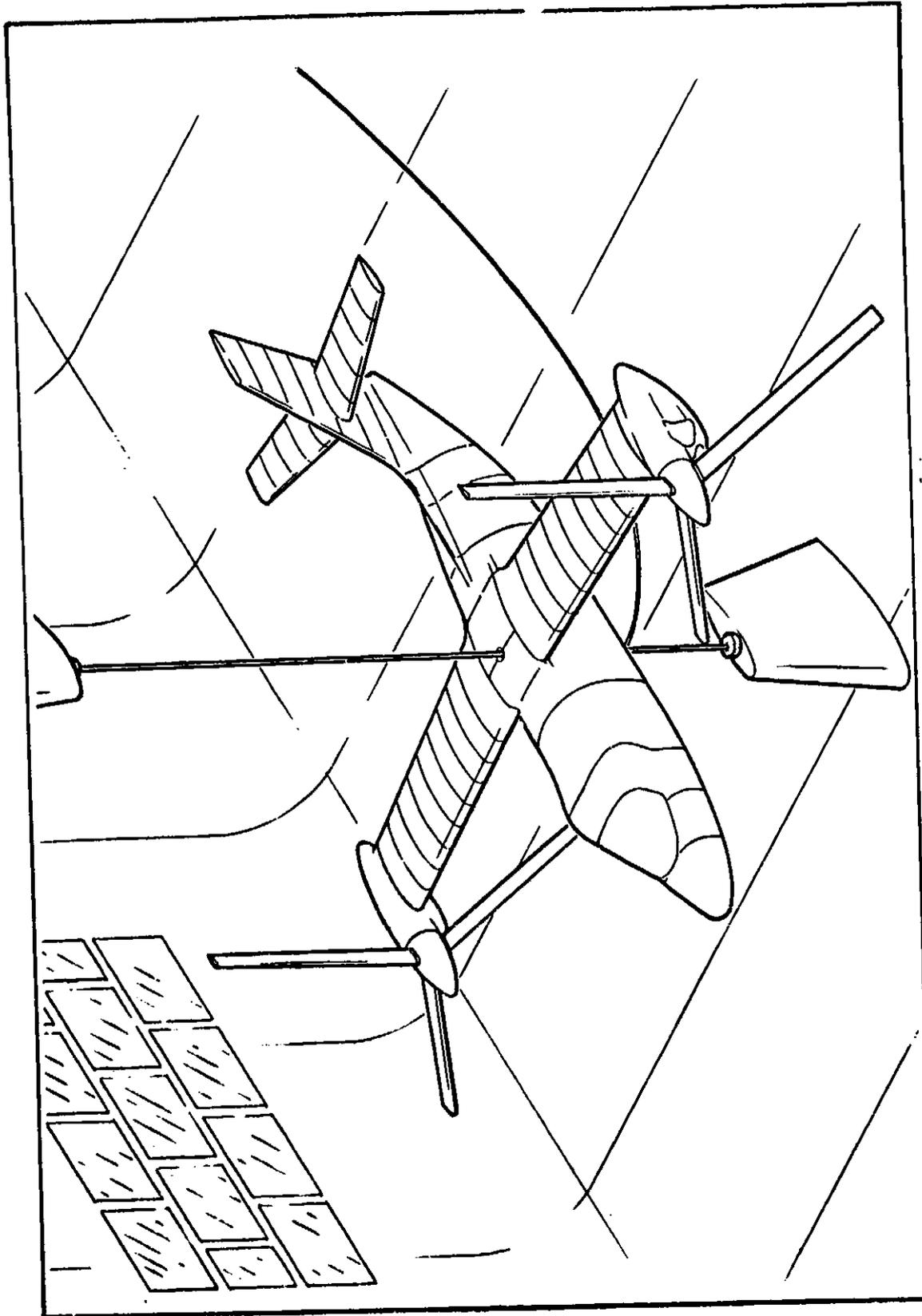
Figure VI-15. Model 300 Full-Span Model in NASA-Langley 16-Foot Transonic Dynamic Tunnel.
