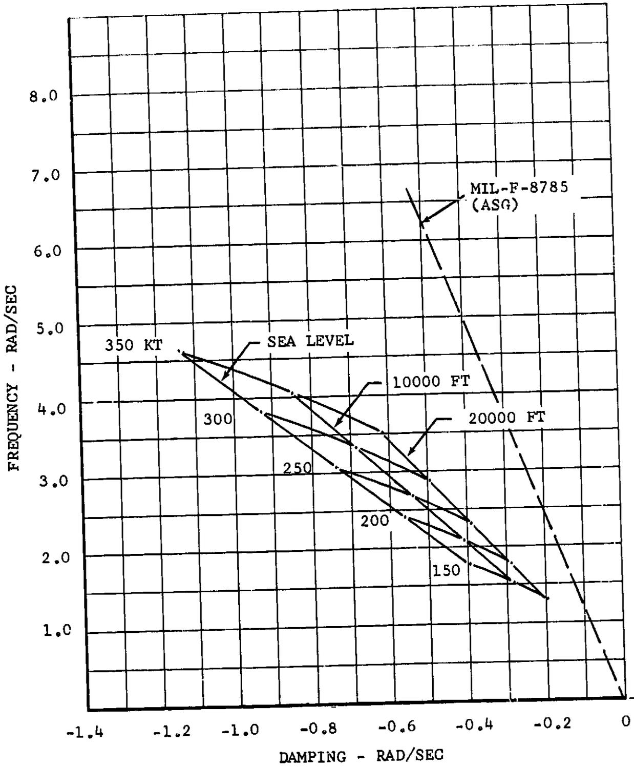
Figure VI-23. Root Locus of Dutch-Roll Mode for Basic Airframe.
