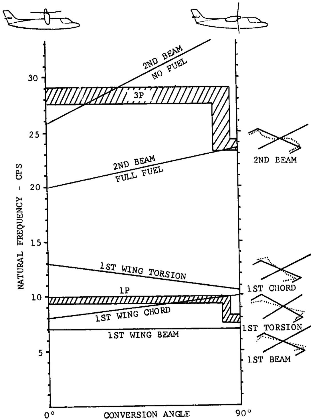
Figure VI-7. Airframe Asymmetric Mode Natural Frequencies.
