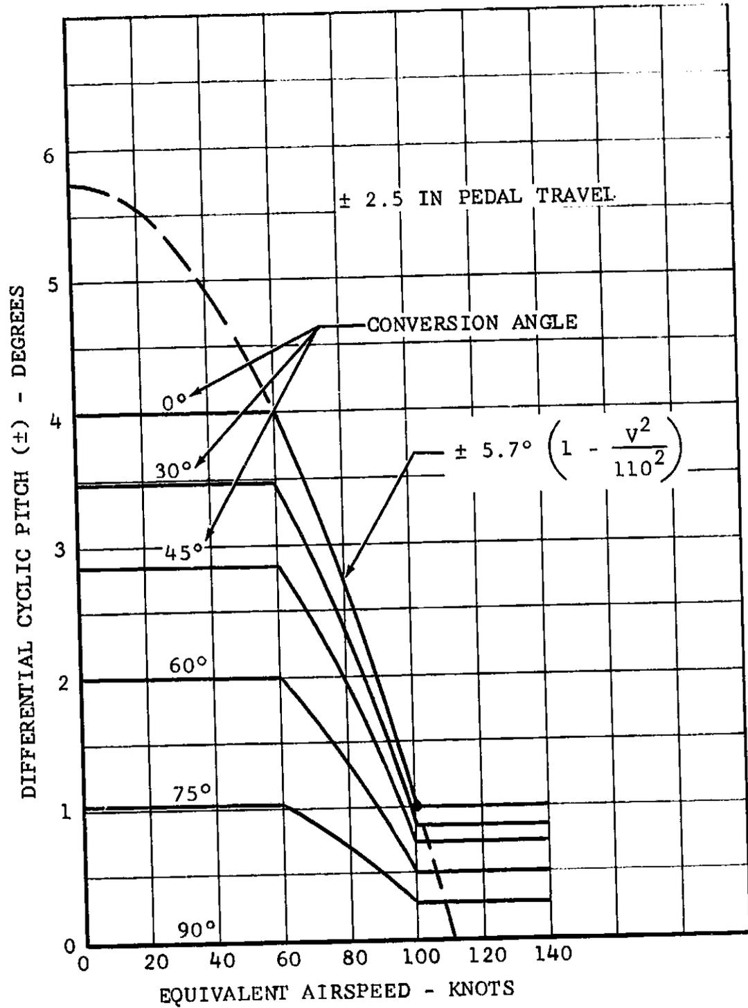
Figure III-11. Differential Cyclic Pitch Versus Airspeed.
