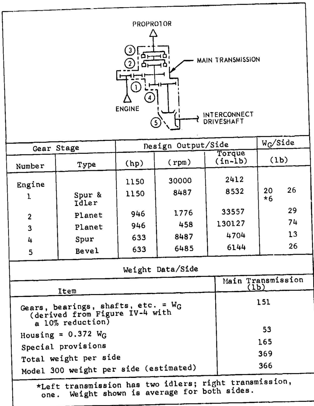
Figure IV-5. Main Transmission Schematic and Weight Data.
