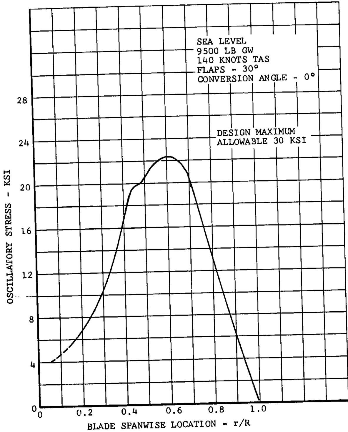
Figure VI-3. Blade Oscillatory Stress at  $V_H$ , Helicopter Mode.
