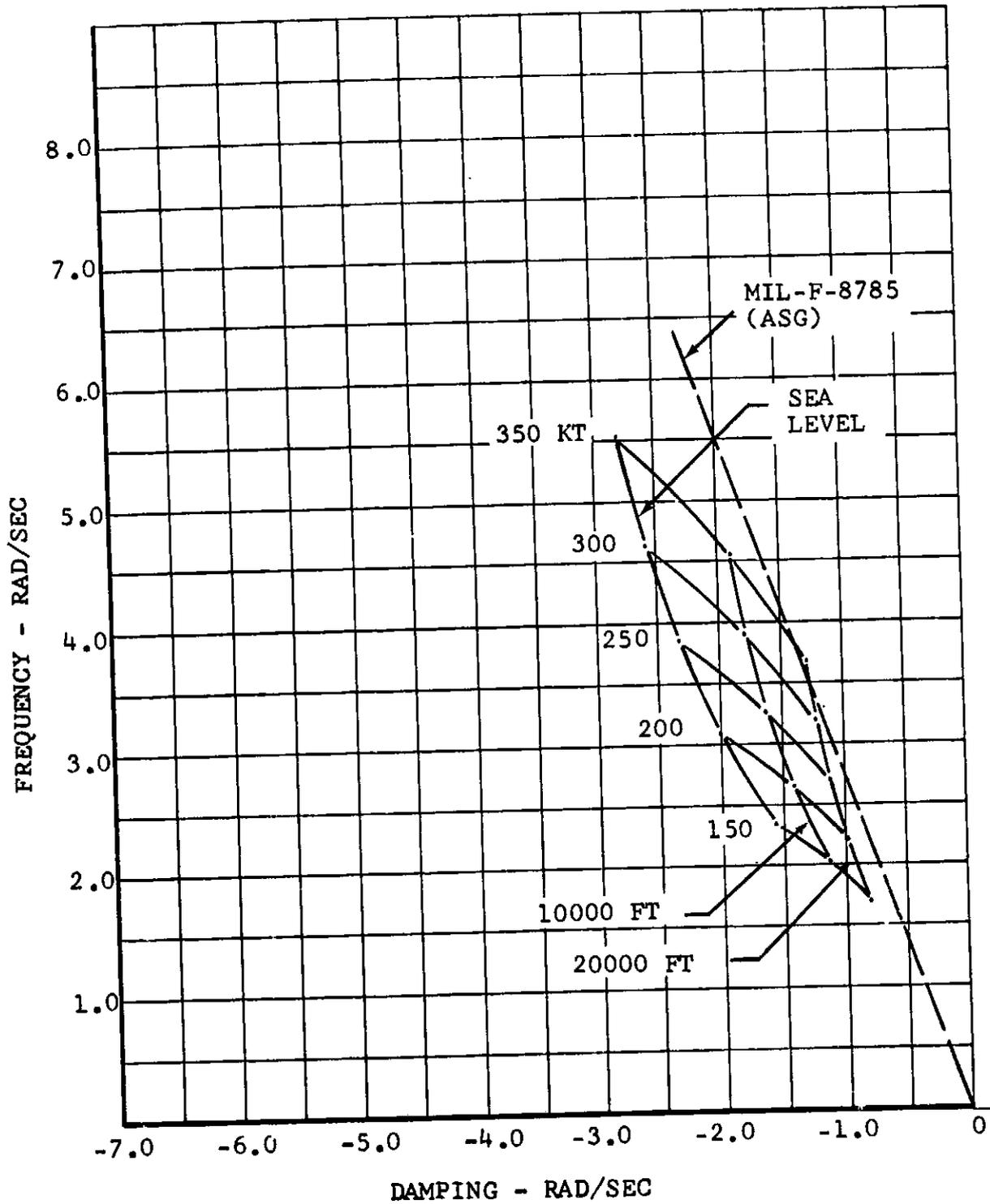
Figure VI-20. Root Locus of Longitudinal Short-Period Mode.
