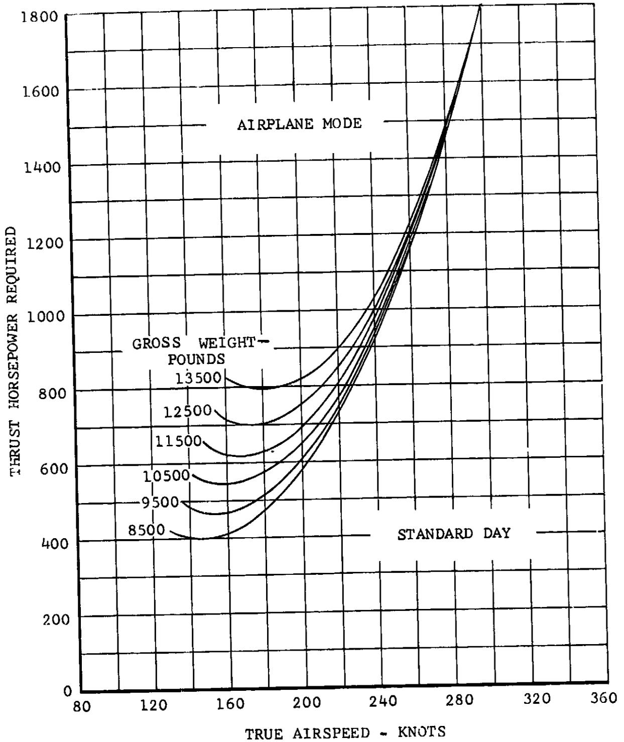
Figure V-26. Thrust Horsepower Required Versus True Airspeed, Sea Level.
