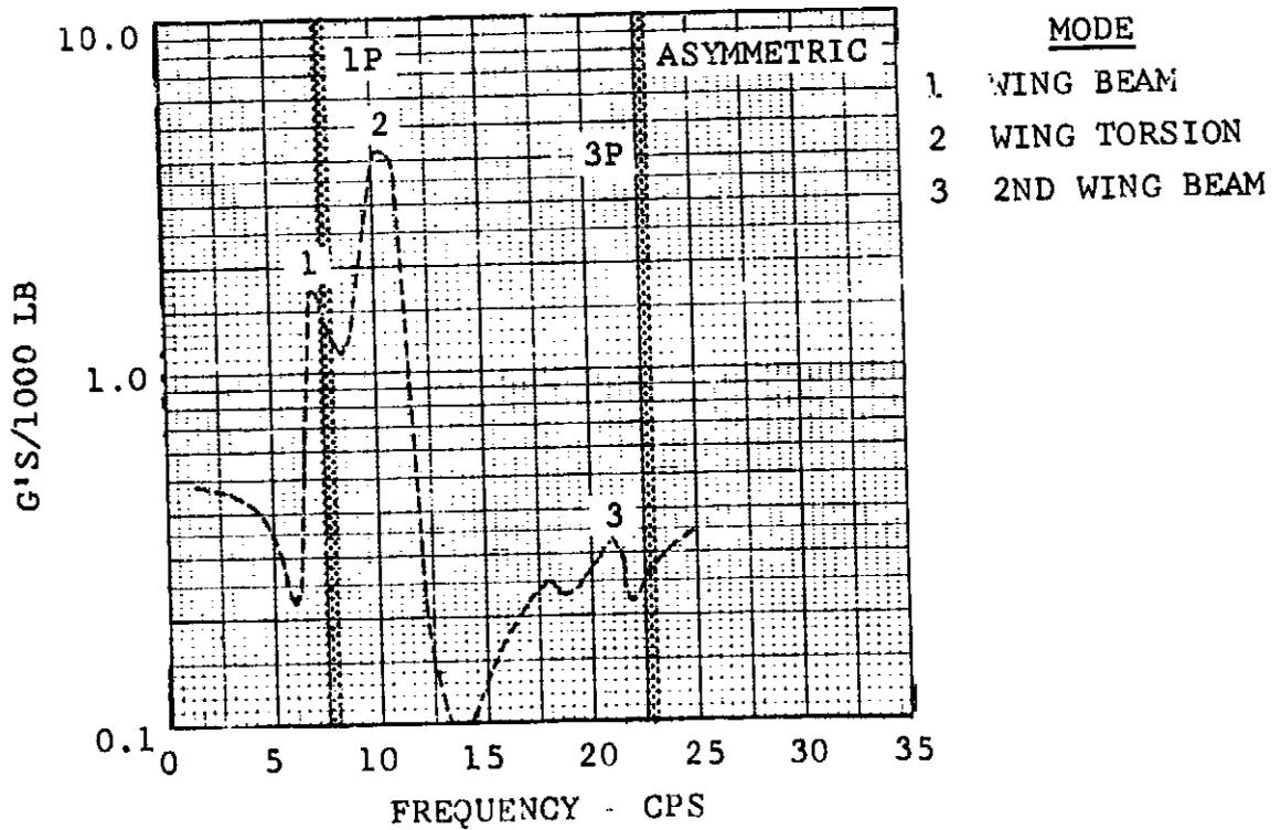
Figure VI-10. Pylon and Crew Station Frequency Response, Airplane Mode.
