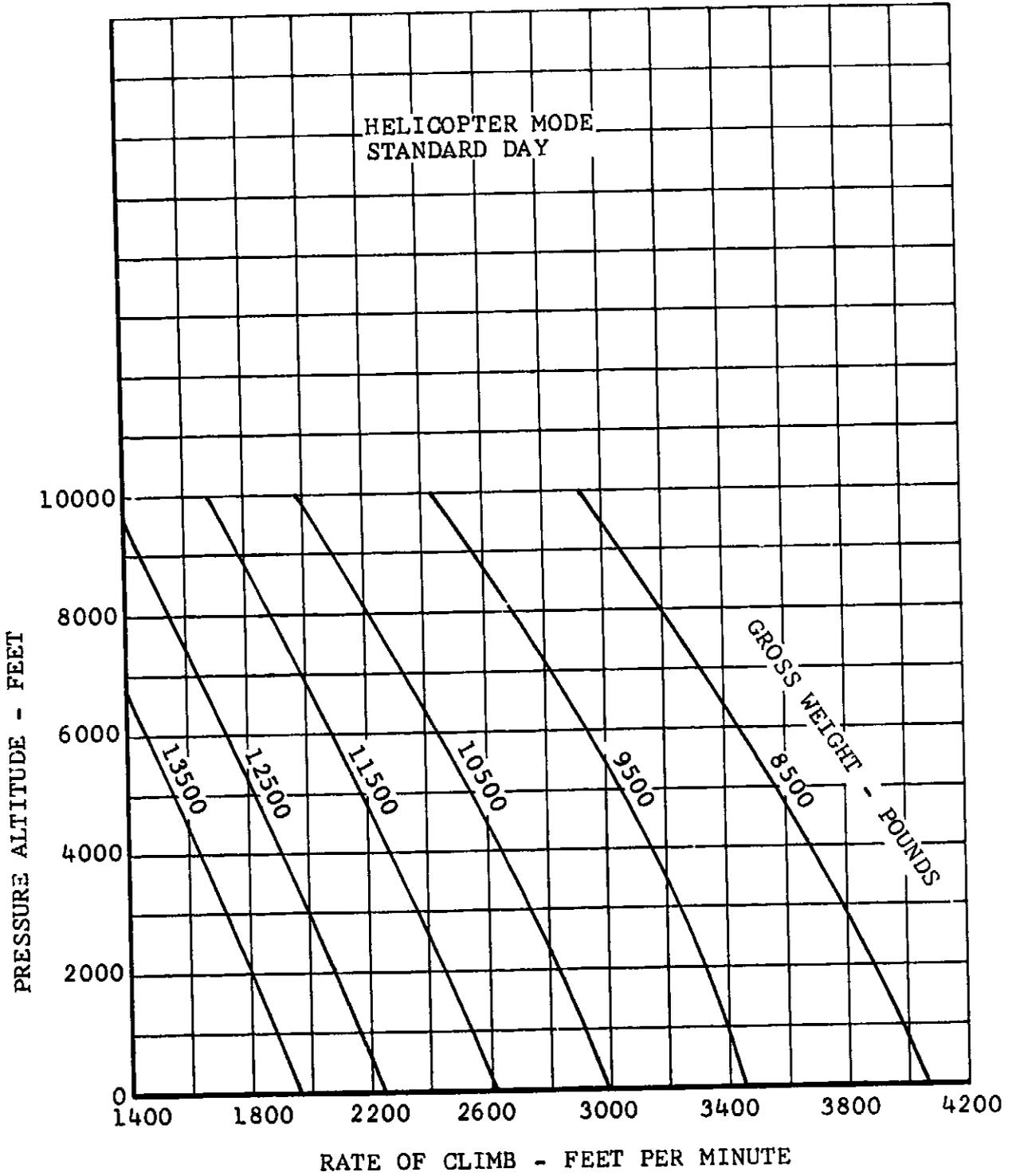
Figure V-25. Rate of Climb, Helicopter Mode.
