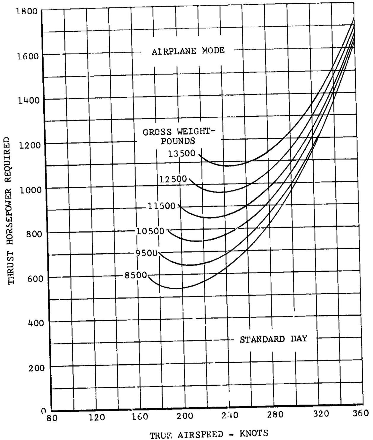
Figure V-28. Thrust Horsepower Required Versus True Airspeed, 20,000 Feet.
