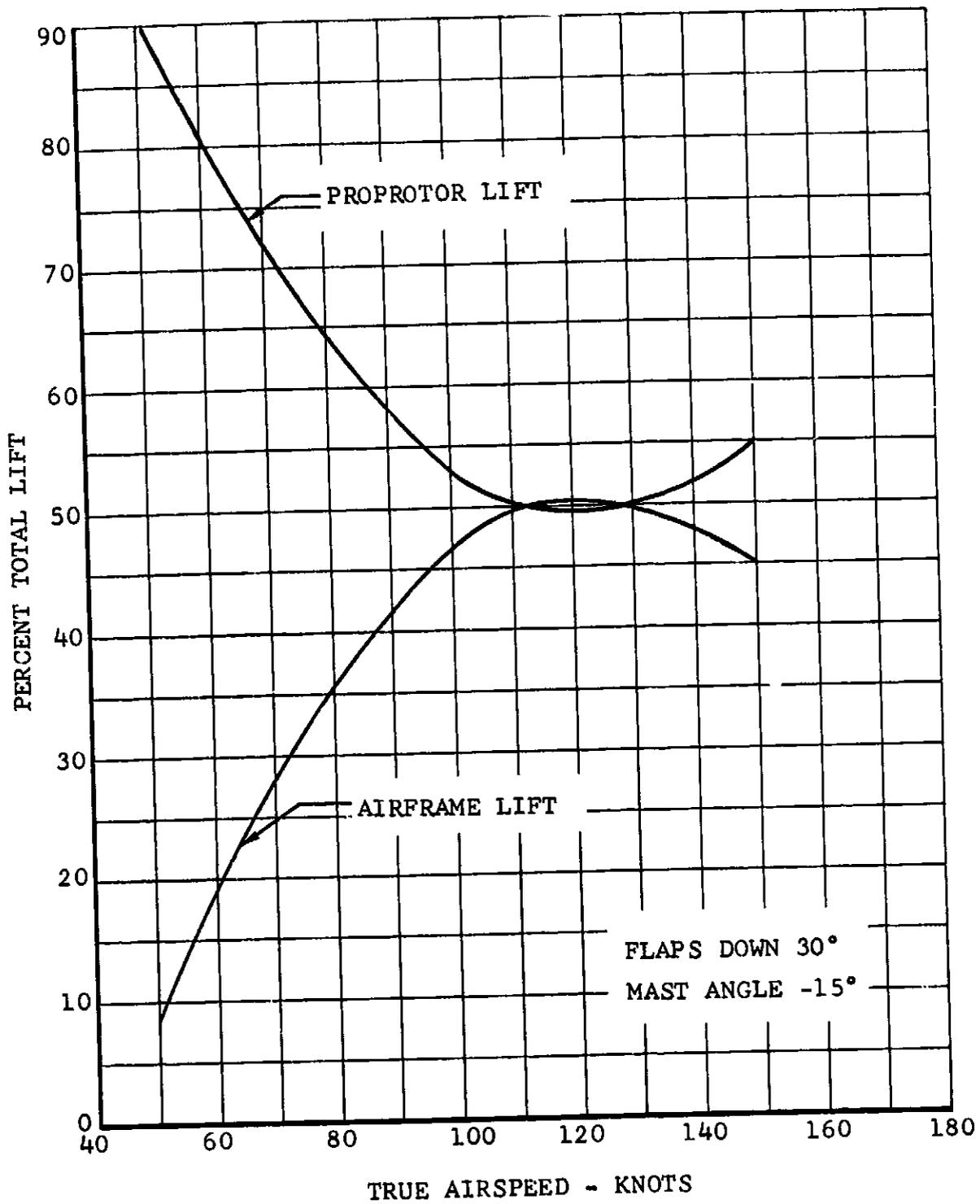
Figure V-24. Lift Distribution Between Proprotor and Airframe in Helicopter Level Flight.
