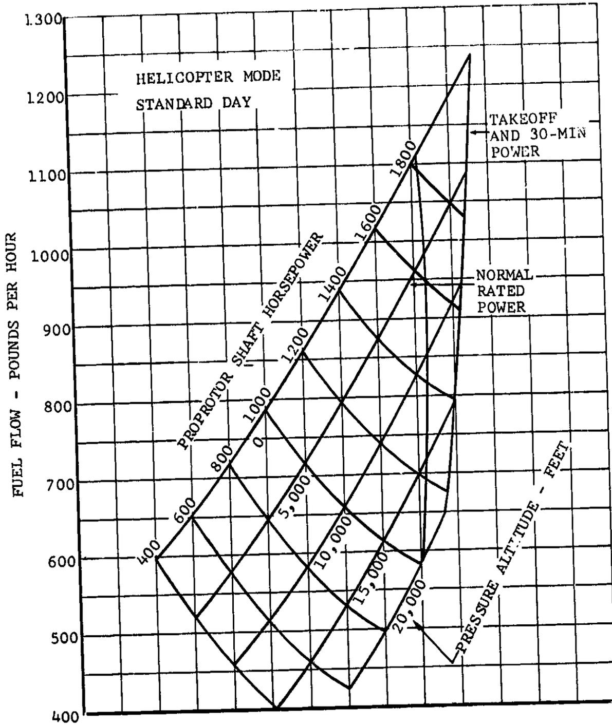
Figure V-17. Fuel Flow, Helicopter Mode.
