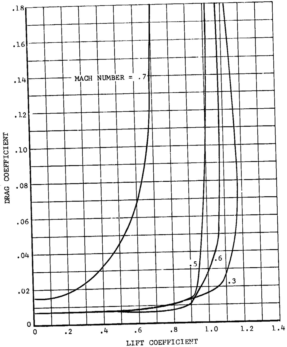
Figure V-7. Proprotor Blade Section Data Blade Station 0.45 to 0.70.
