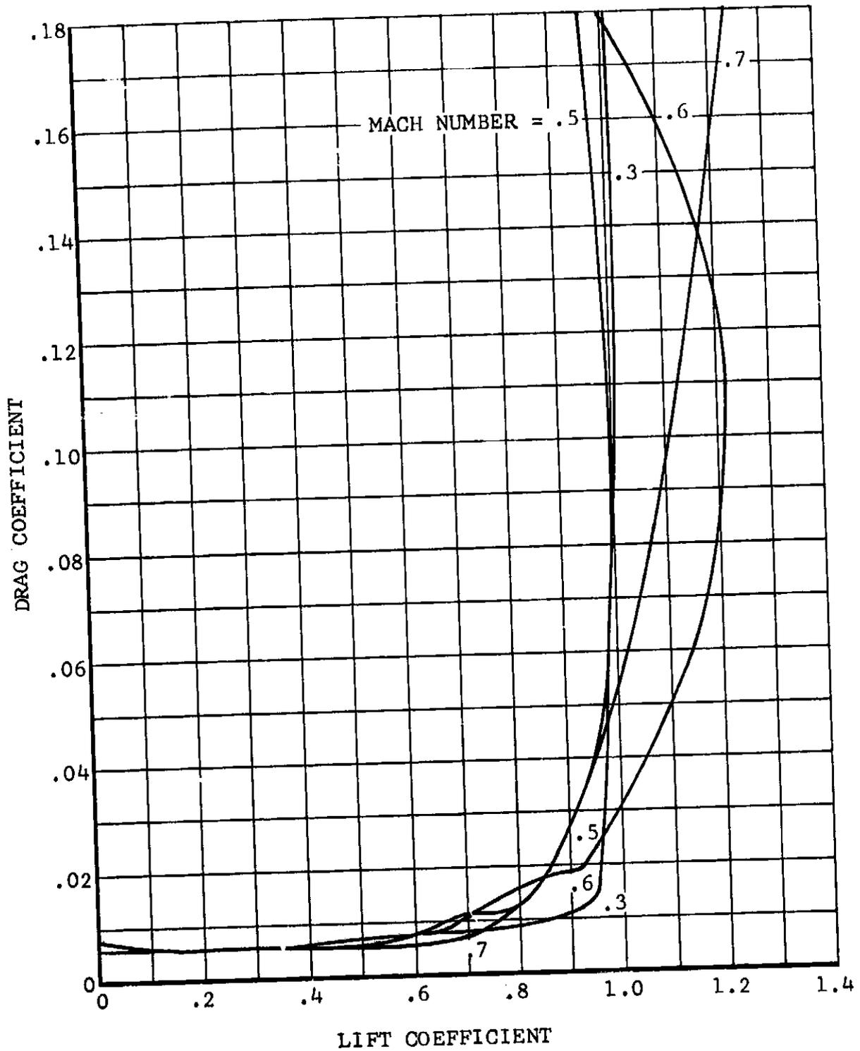
Figure V-9. Proprotor Blade Section Data, Radial Station 0.90 to 1.00.
