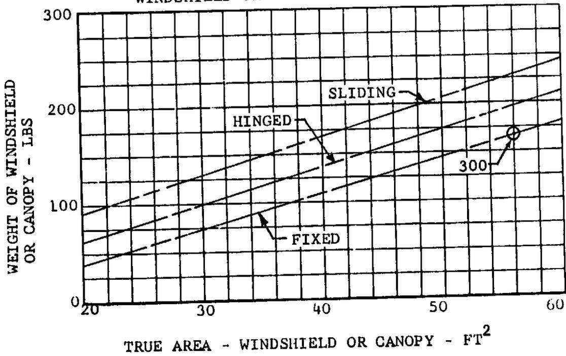
Figure IV-2. Fuselage Weight Estimation Parameters.
