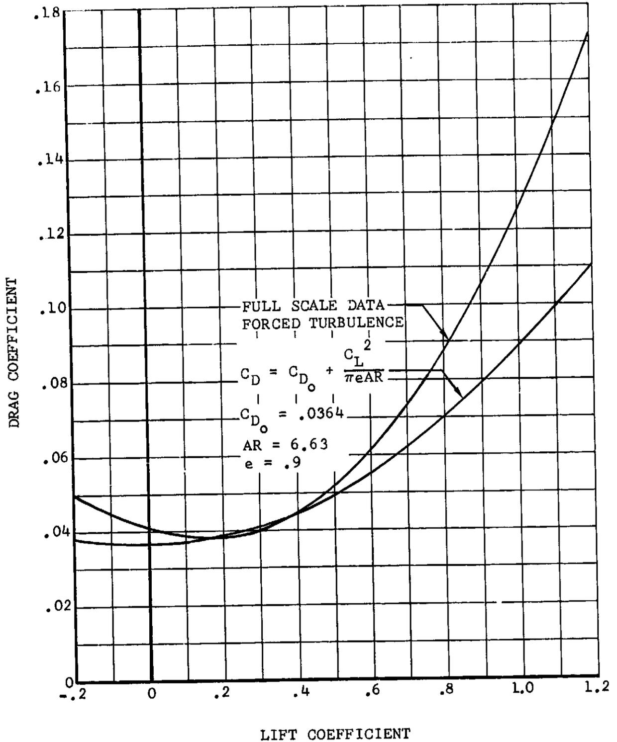
Figure V-5. Comparison of Full-Scale Aircraft Drag, Based on Tunnel Results and Calculated Data.
