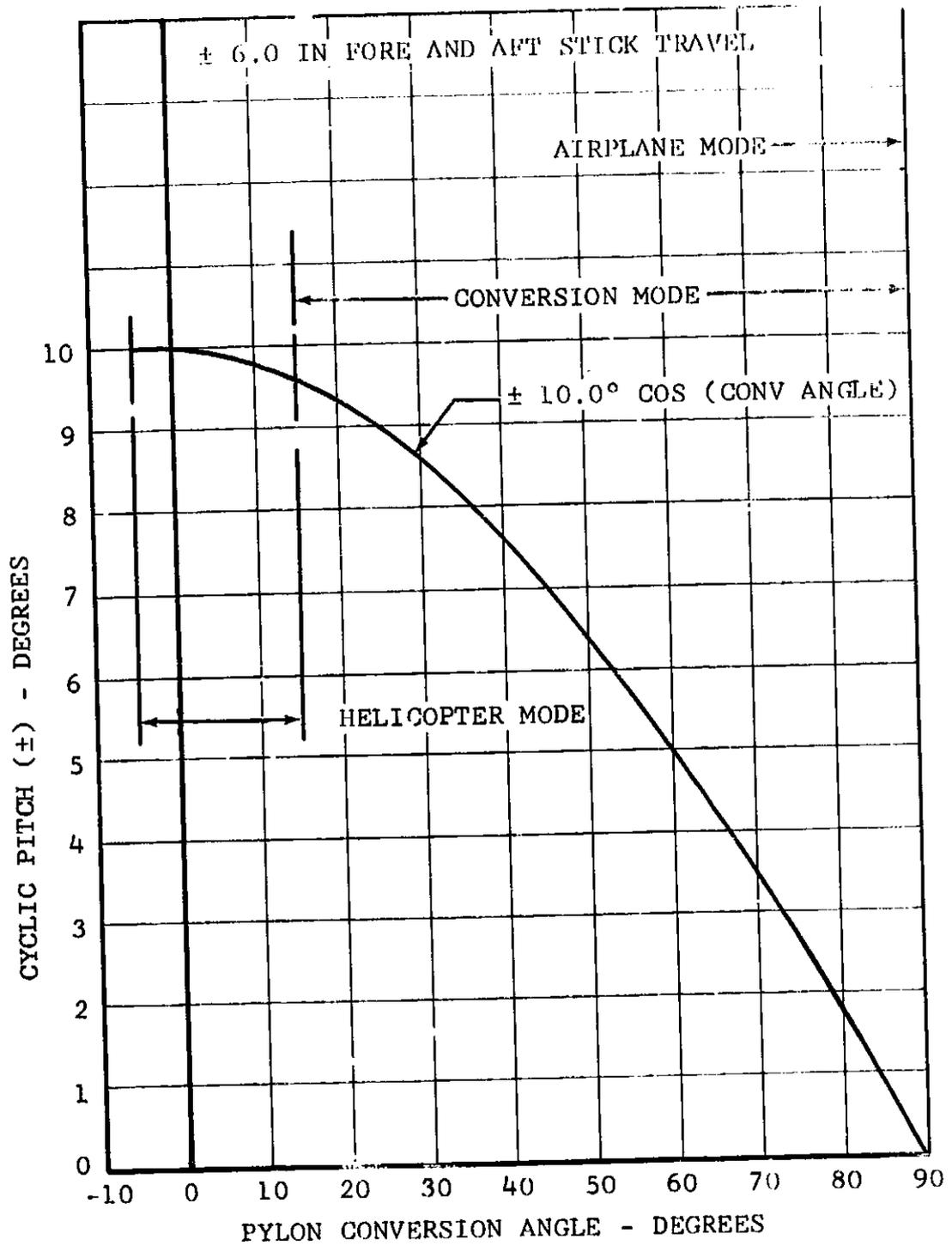
Figure III-9. Fore and Aft Cyclic Pitch Versus Conversion Angle.
