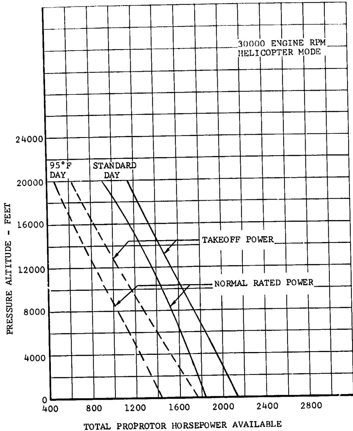
Figure V-16. Twin Engine Proprotor Shaft Horsepower Available, Helicopter Mode.
