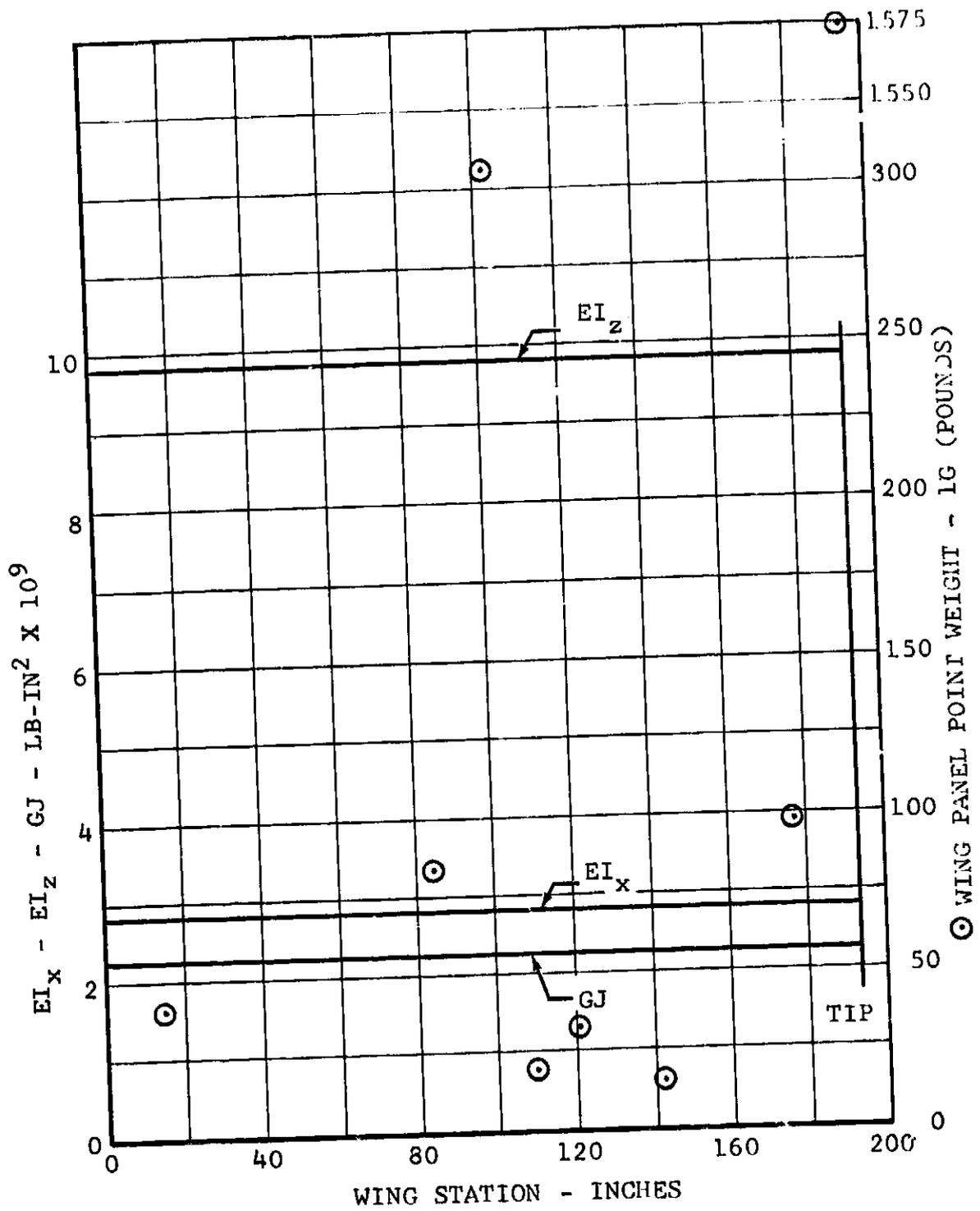
Figure III-3. Wing Stiffness and Panel Point Weight.
