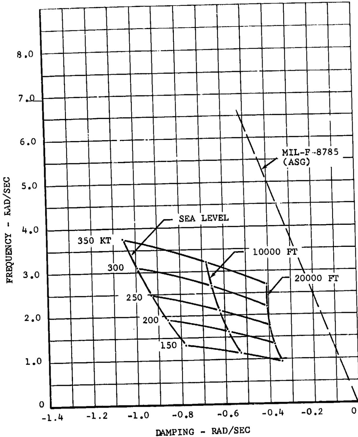
Figure VI-22. Root Locus of Dutch-Roll Mode.
