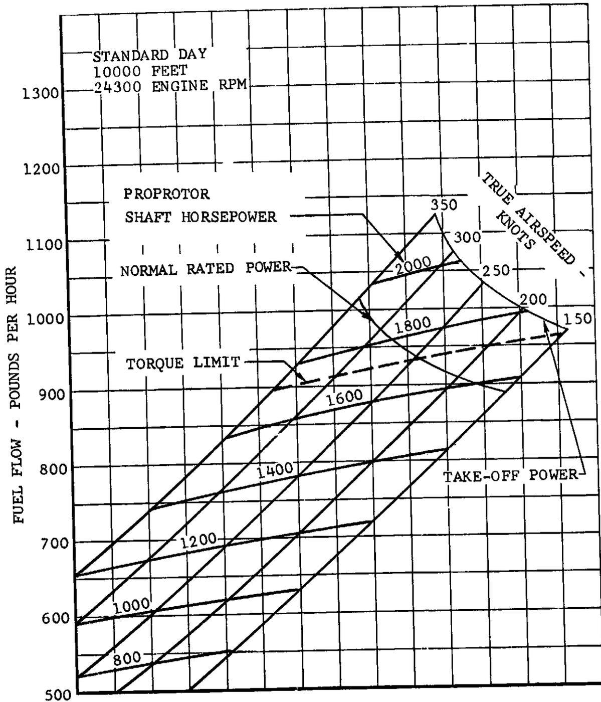
Figure V-20. Fuel Flow, Airplane Mode.
