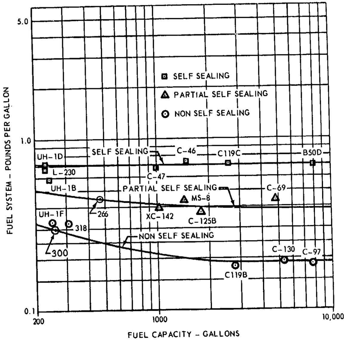
Figure IV-3. Fuel System Weight.
