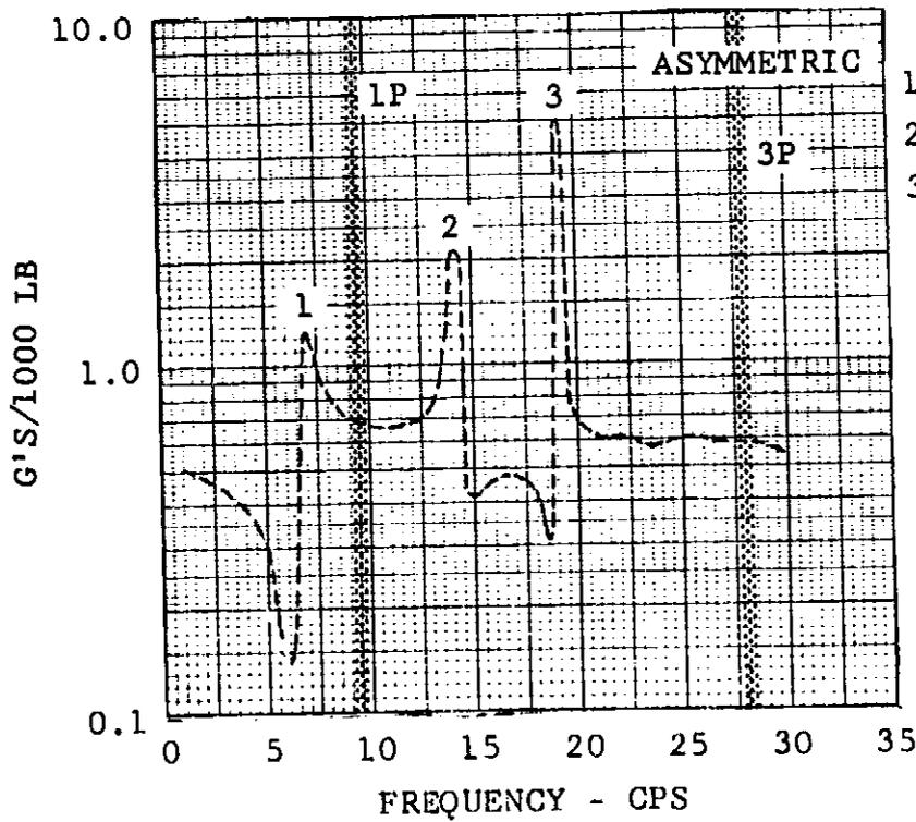
Figure VI-9. Pylon and Crew Station Frequency Response, Helicopter Mode.
