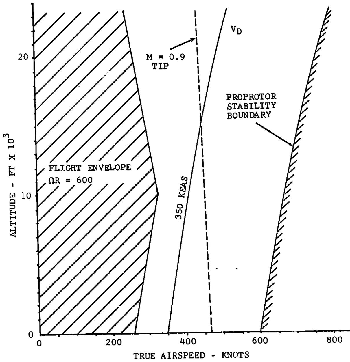
Figure VI-11. Model 300 Proprotor Stability Boundary.
