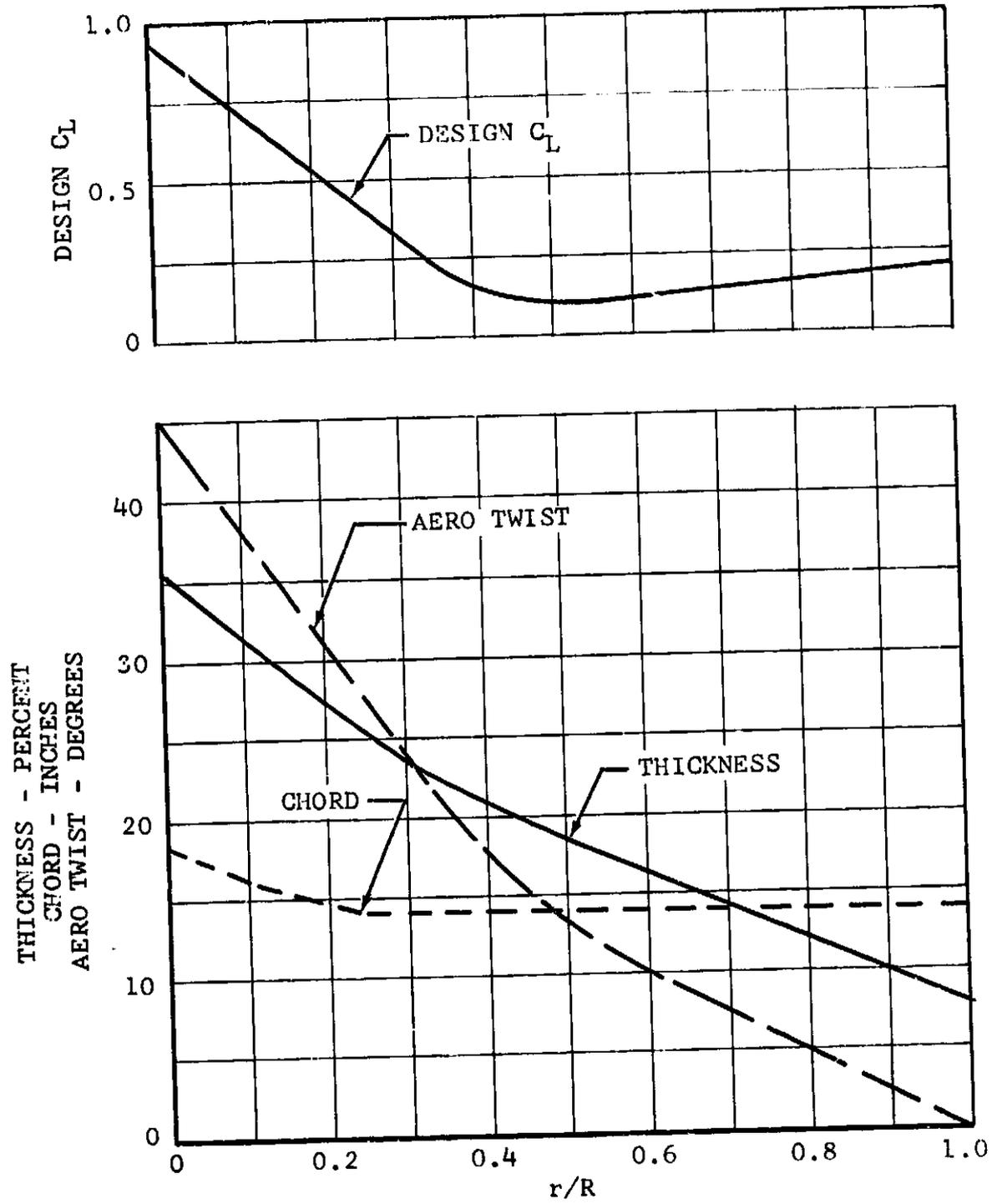
Figure III-1. 25-Foot Proprotor Parameters.
