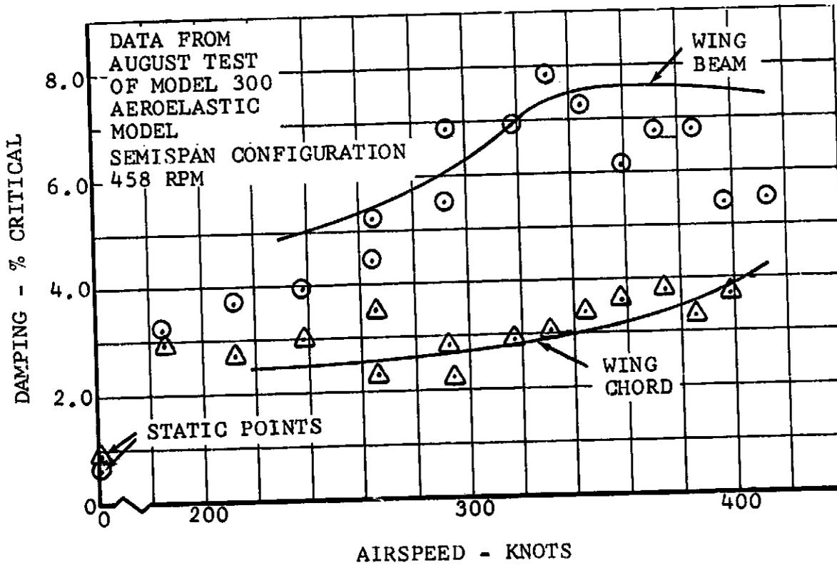
Figure VI-13. Model 300 Aeroelastic Model Proprotor Stability (Full-Scale Frequency and Airspeed).
