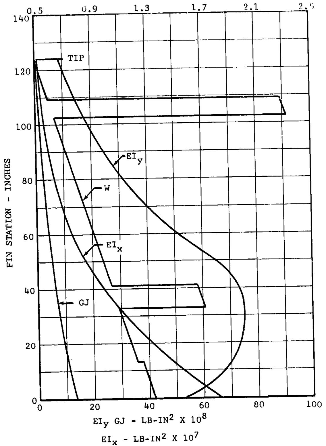
Figure III-5. Vertical Tail Stiffness and Weight Distribution.
