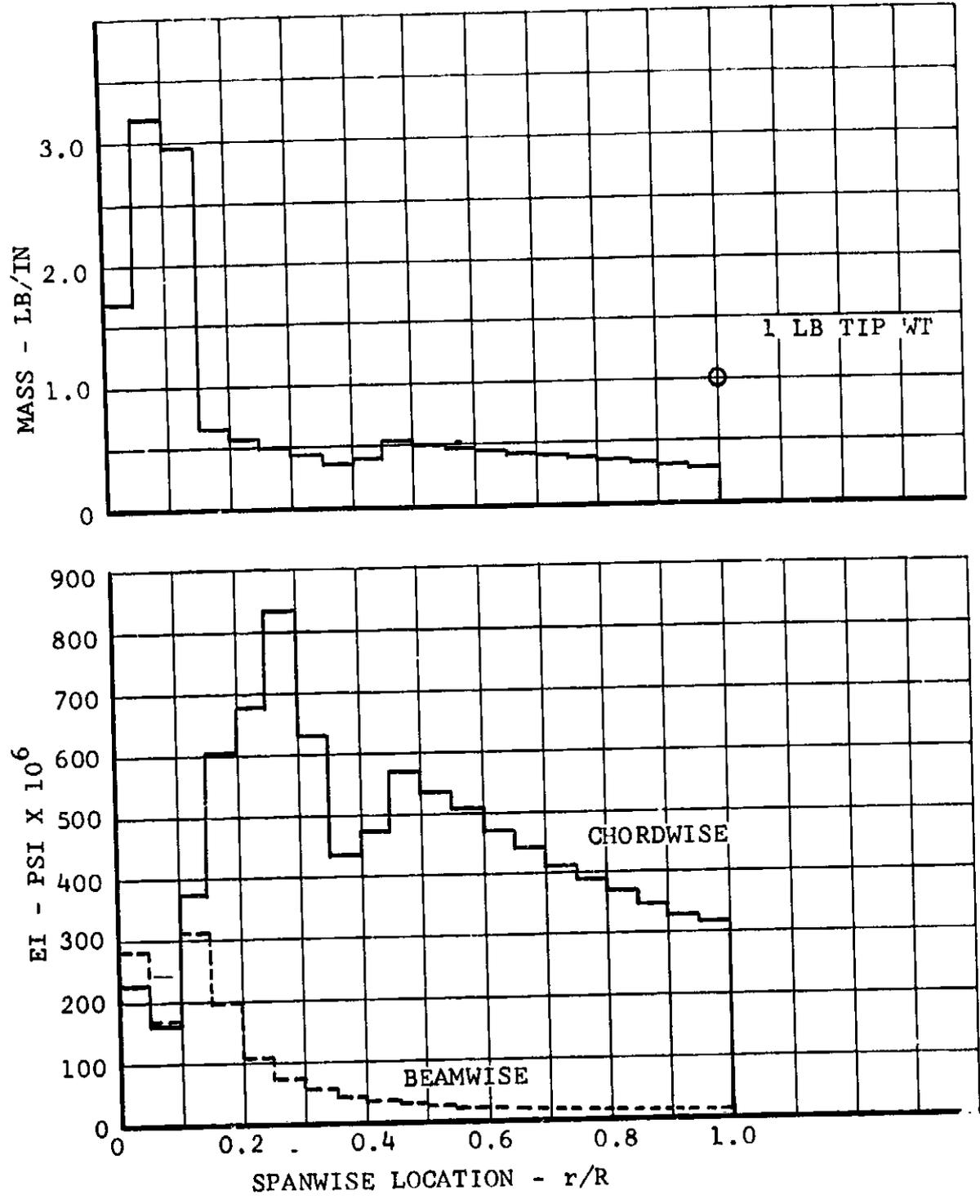
Figure III-2. Proprotor Stiffness and Mass Distribution.
