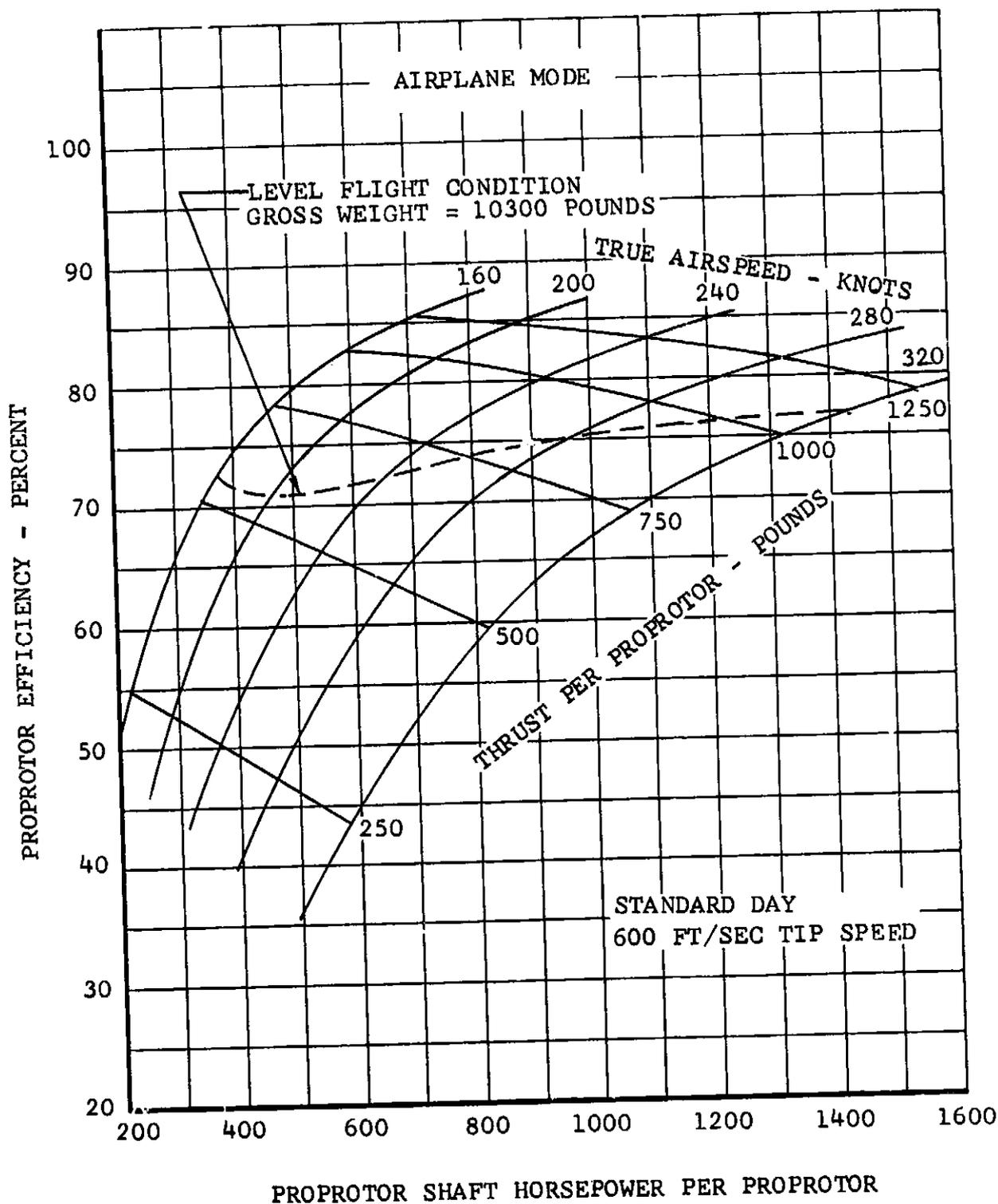
Figure V-13. Proprotor Efficiency Versus Shaft Horsepower Sea Level.
