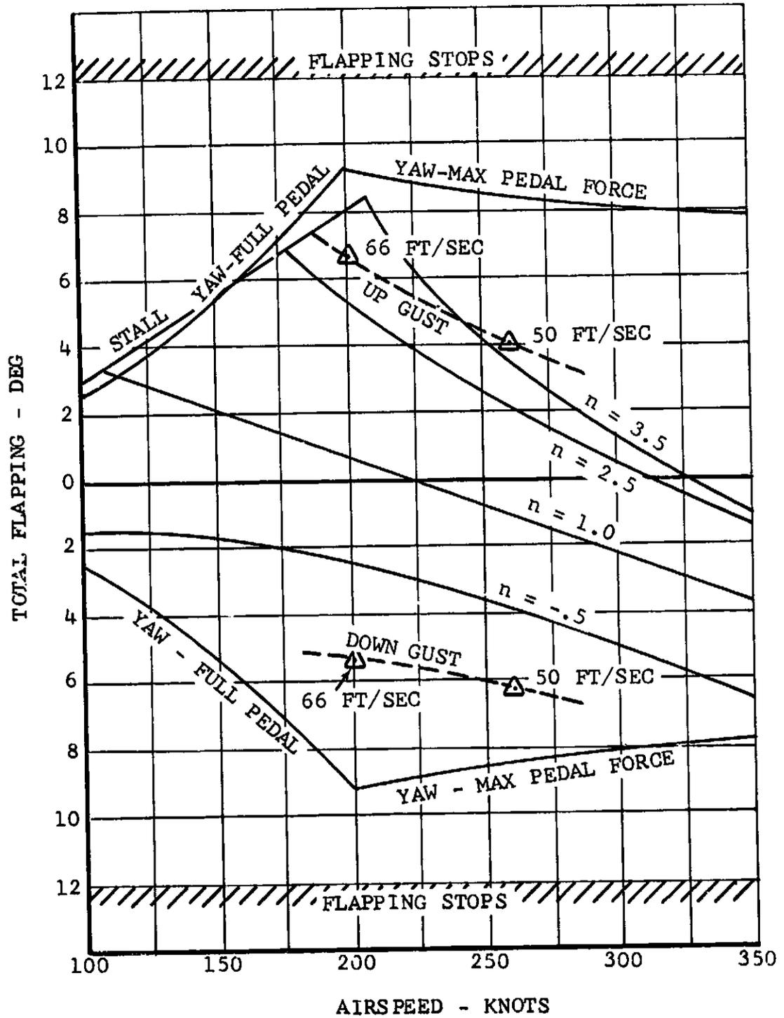
Figure VI-5. Flapping Envelope in Airplane Mode.
