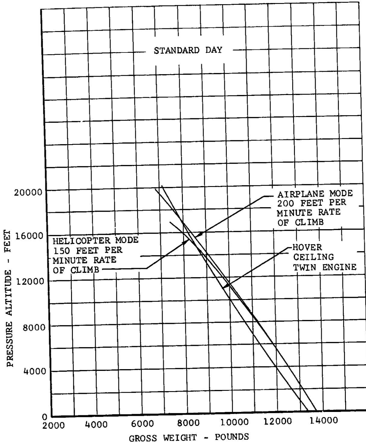
Figure V-37. Single Engine Performance.
