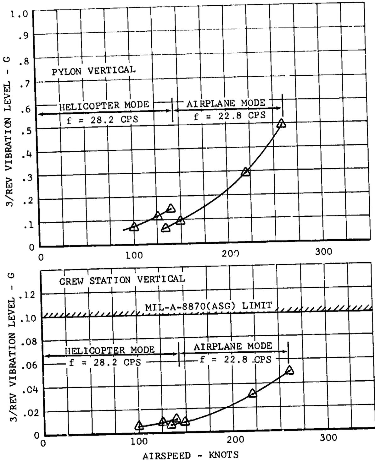
Figure VI-8. Pylon and Crew Station Vibration.
