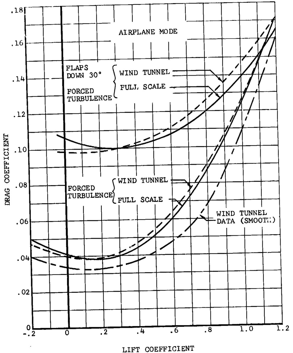
Figure V-4. Airframe Drag Coefficient Versus Lift Coefficient.
