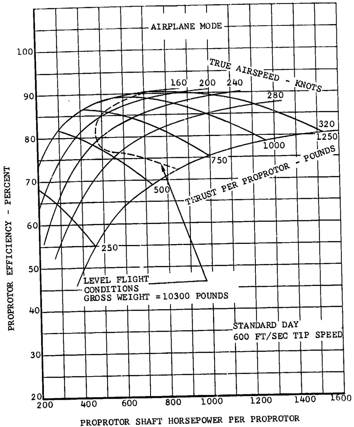
Figure V-15. Proprotor Efficiency Versus Shaft Horsepower 20,000 Feet.
