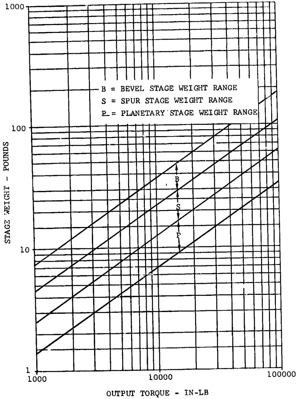
Figure IV-4. Gear Stage Weight.
