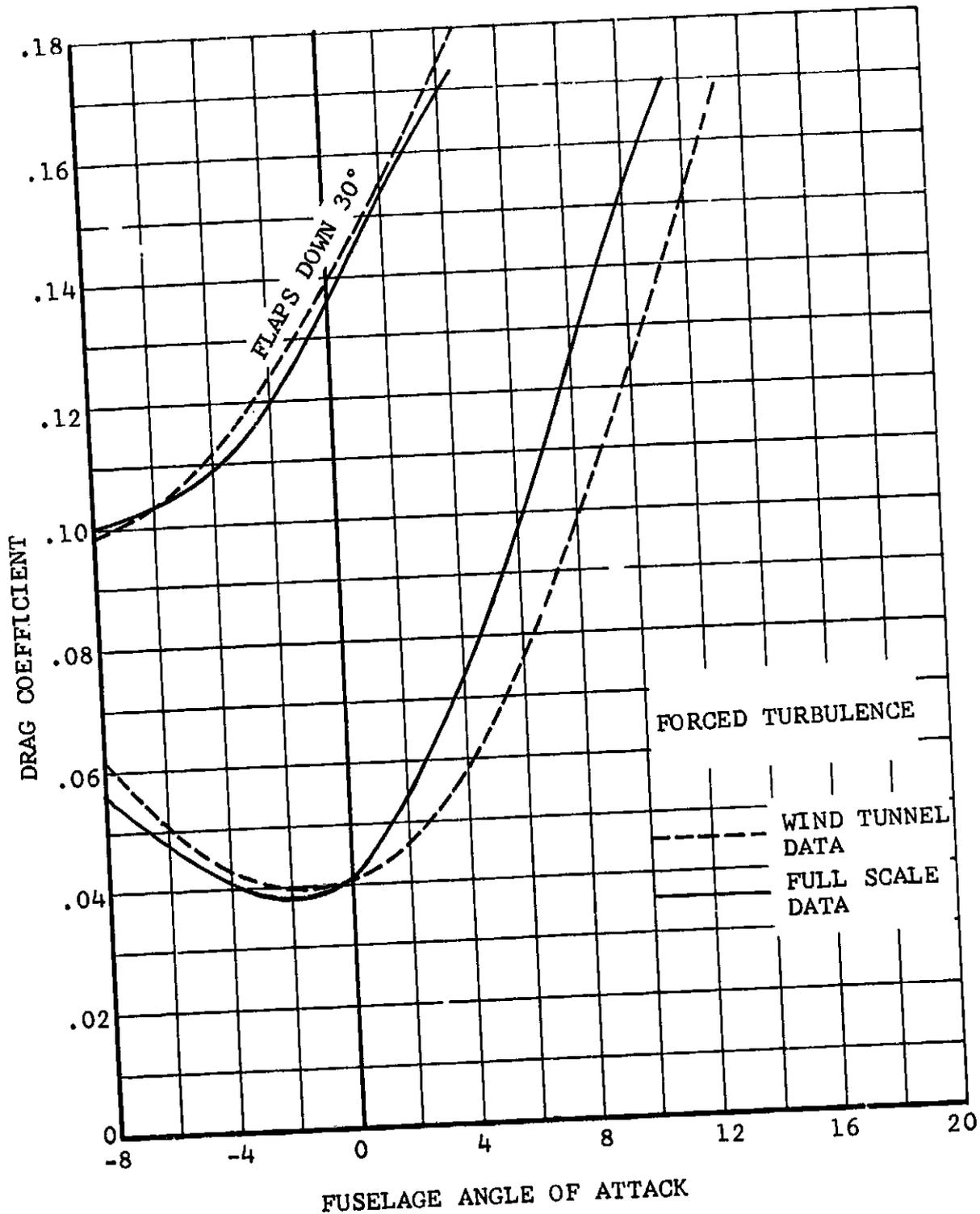
Figure V-3. Airframe Drag Coefficient Versus Fuselage Angle of Attack.
