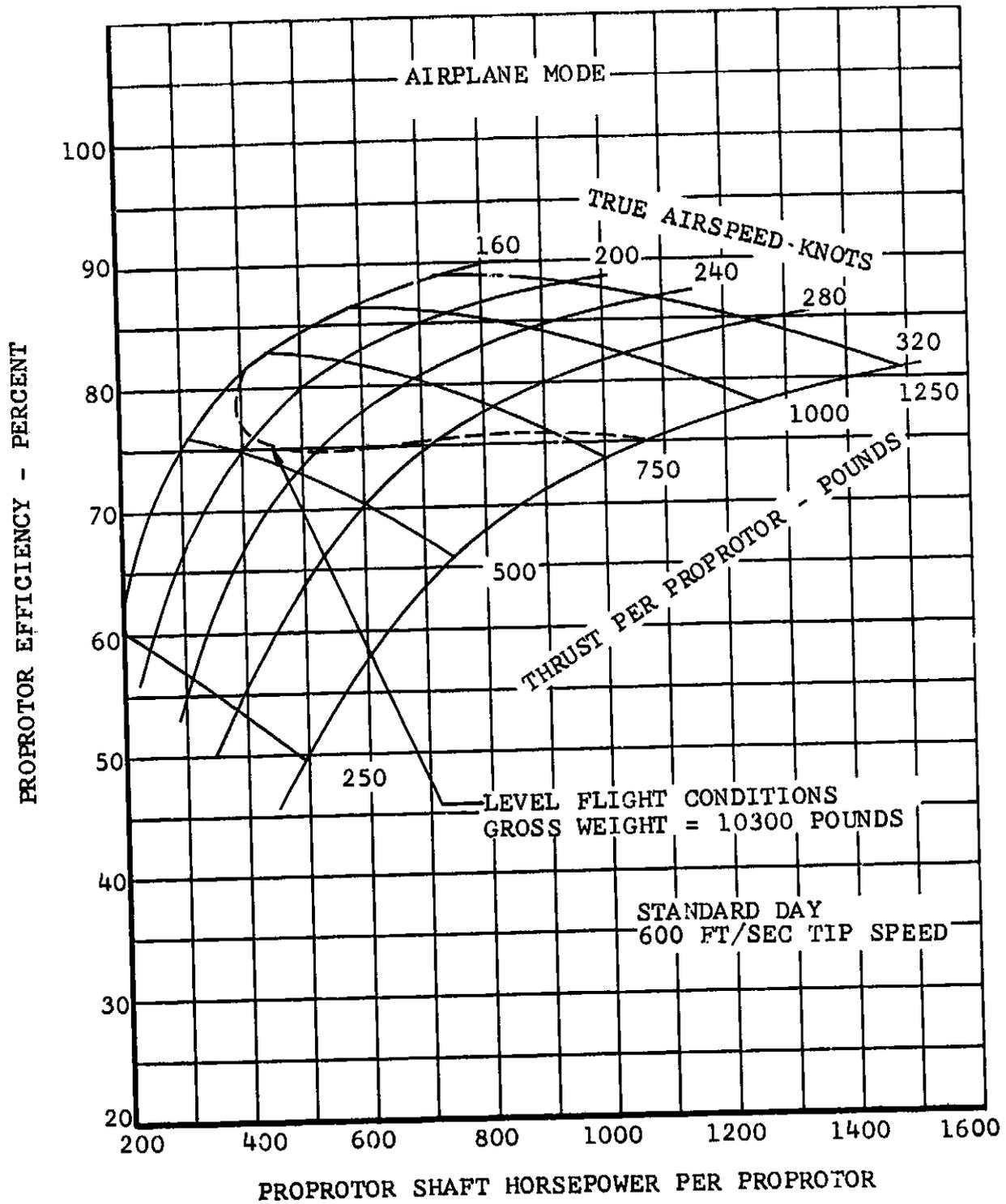
Figure V-14. Proprotor Efficiency Versus Shaft Horsepower 10,000 Feet.
