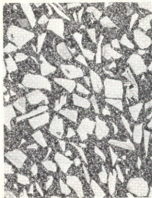
NORTON LOW FIRED SiC DUPLEX GRAIN SIZE: 100 \mu\text{m} , 4 \mu\text{m}
