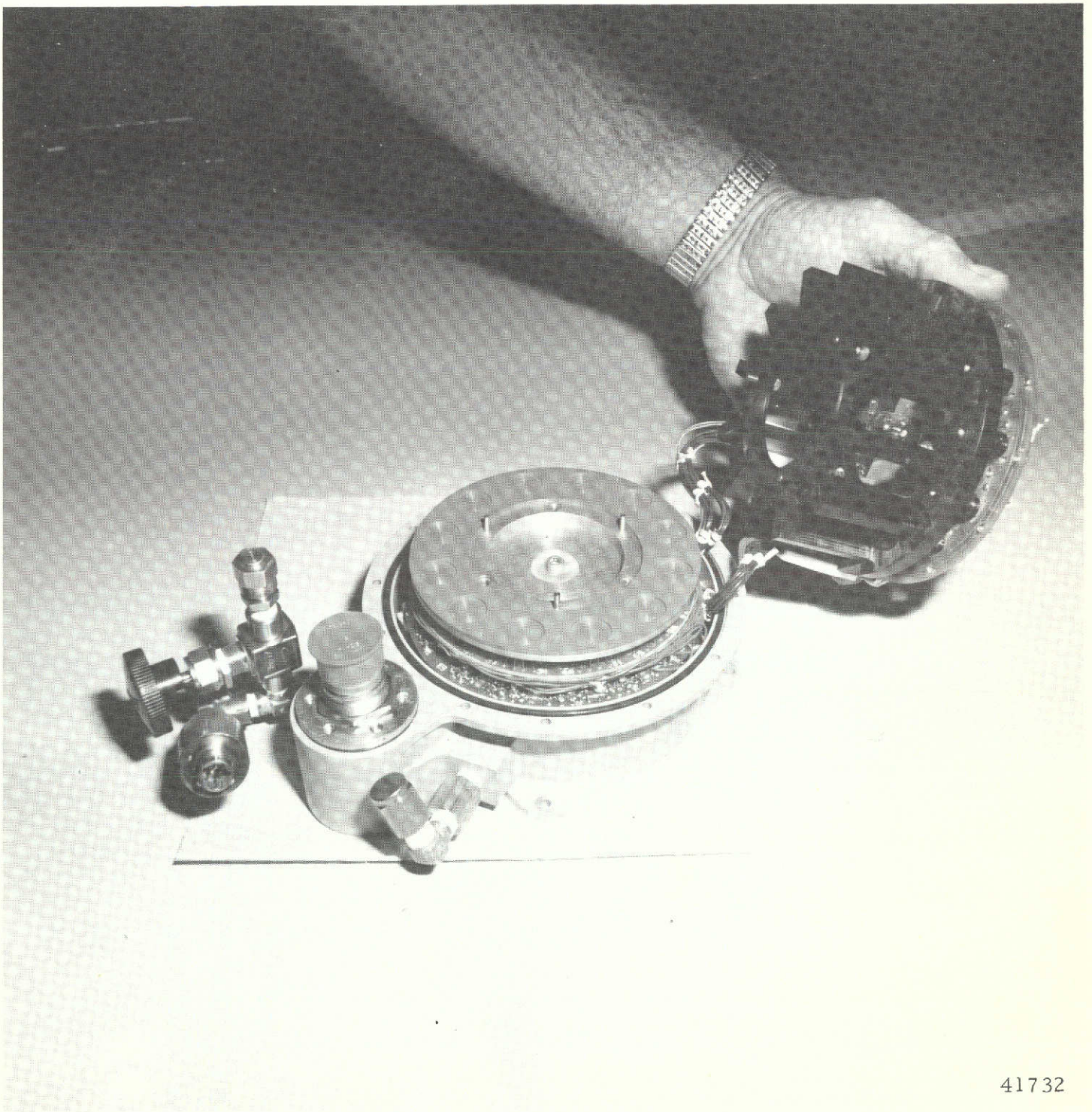
FIGURE 1 - 6 CIRCADIAN PERIODICITY EXPERIMENT VINEGAR GNAT ENCLOSURE
