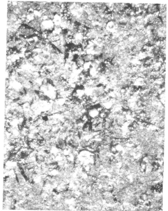
(d) Machined, sanded, and heat-treated in air for 20 hours at 816°C.
