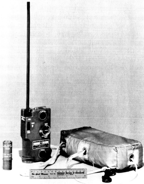
Figure 6.- Apollo swimmer radio, battery pack, and flotation bag.
