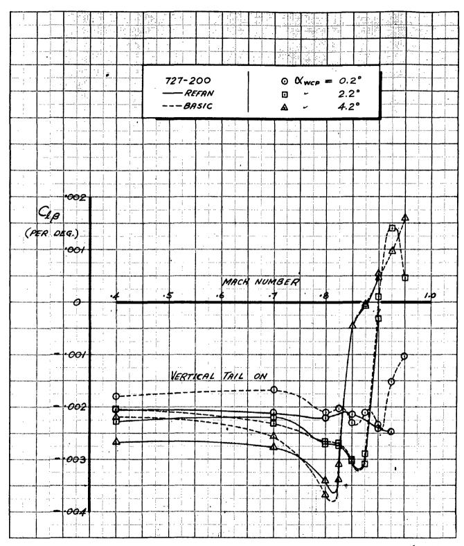
FIGURE 14. - EFFECT OF NASA REFAN NACELLES ON LATERAL STABILITY (CLB)
