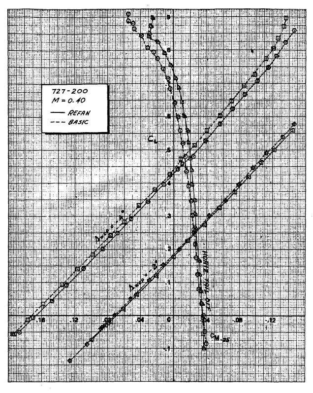
FIGURE 5. - EFFECT OF NASA REFAN NACELLES ON PITCHING MOMENT, 727-200, M = 0.40
