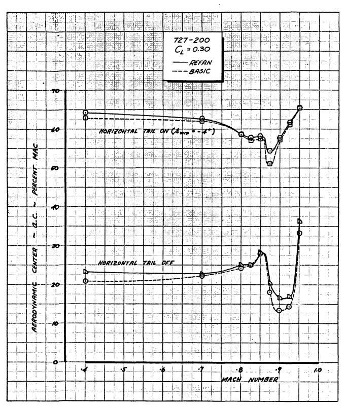
FIGURE 11. - EFFECT OF NASA REFAN NACELLES ON LONGITUDINAL STABILITY, 727-200, C. = 0.30
