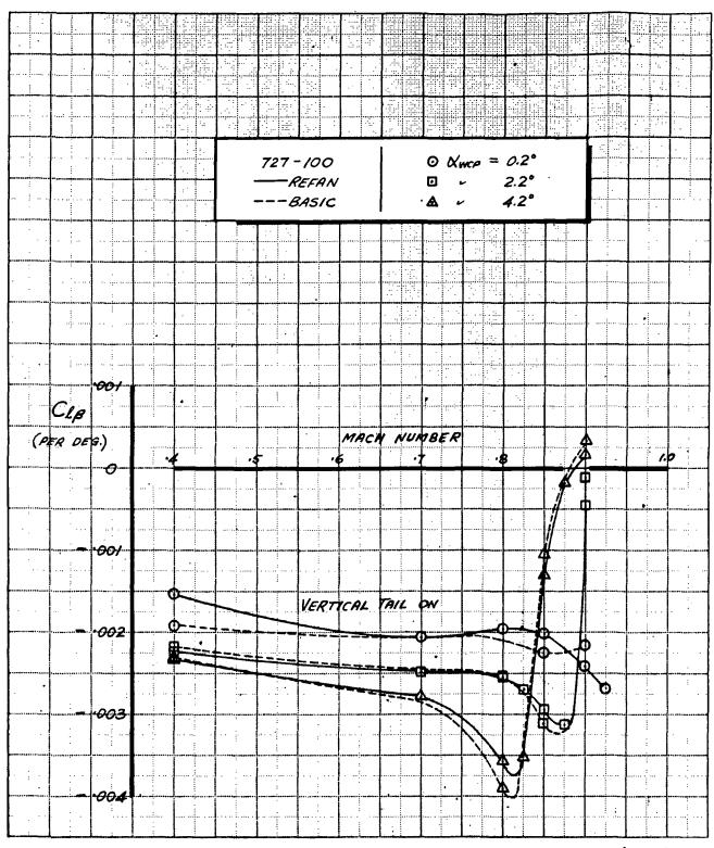
FIGURE 18. - EFFECT OF NASA REFAN NACELLES ON LATERAL STABILITY (CLB), 727-100, VERTICAL TAIL ON
