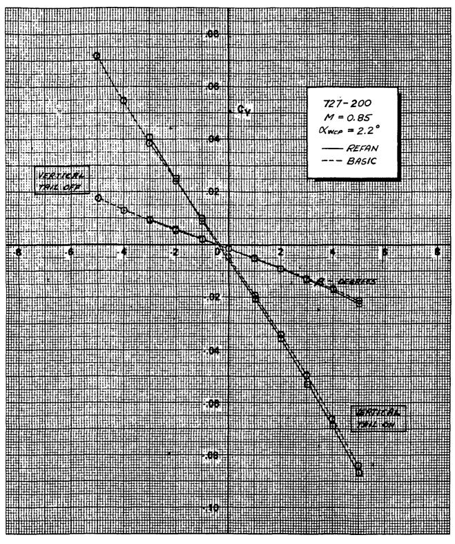
FIGURE 23. - EFFECT OF NASA REFAN NACELLES ON SIDE FORCE, Cy VS B, 727-200, M = 0.85, Xwcp = 2.2°
