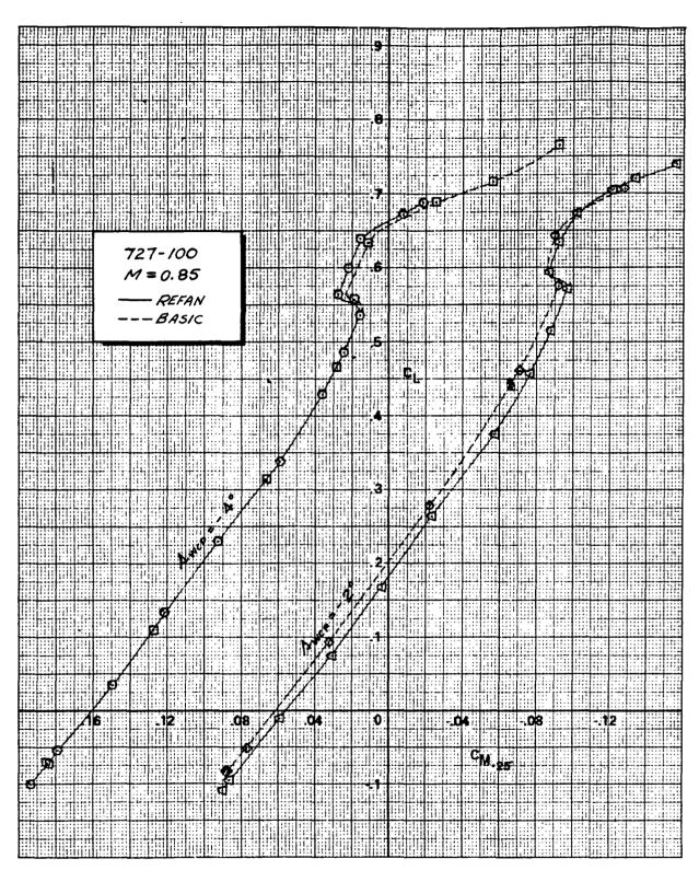
FIGURE 10. - EFFECT OF NASA REFAN NACELLES ON PITCHING MOMENT,
