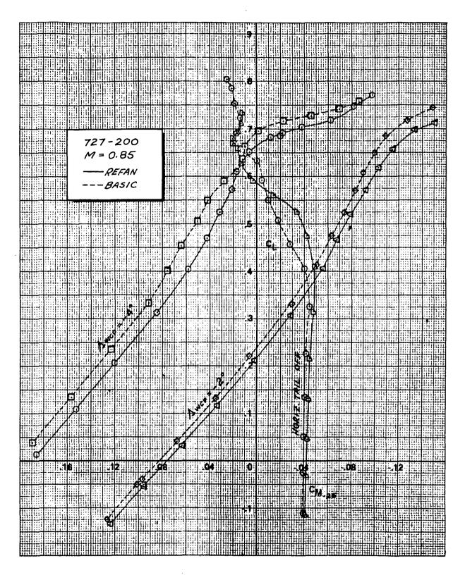
FIGURE 7. - EFFECT OF NASA REFAN NACELLES ON PITCHING MOMENT, 727-200, M = 0.85
