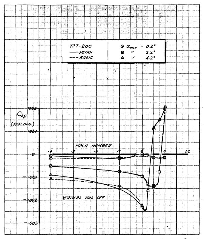
FIGURE 15. - EFFECT OF NASA REFAN NACELLES ON LATERAL STABILITY (CLB)
