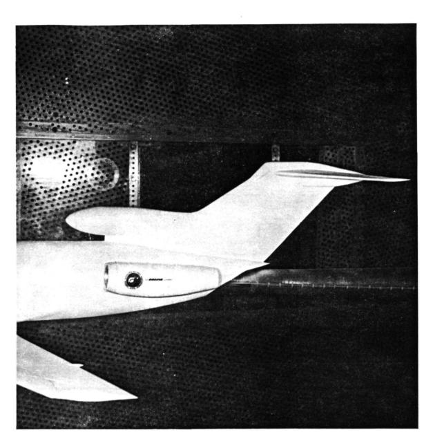
FIGURE 3.-727-200/JT8D-109 NASA REFAN NACELLE INSTALLATION
