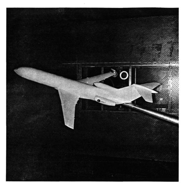
FIGURE 2.—727-200/JT8D-109 NASA REFAN MODEL INSTALLED IN THE CALSPAN CORPORATION TRANSONIC WIND TUNNEL
