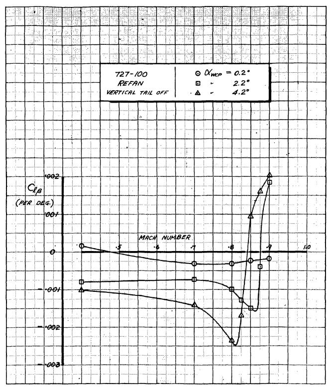
FIGURE 19. - 727-100 REFAN LATERAL STABILITY (CAB), VERTICAL TAIL OFF
