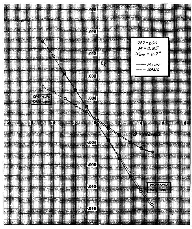
FIGURE 22. - EFFECT OF NASA REFAN NACELLES ON LATERAL STABILITY, CA VS B, 727-200, M = 0.85, Xwcp = 2.2°
