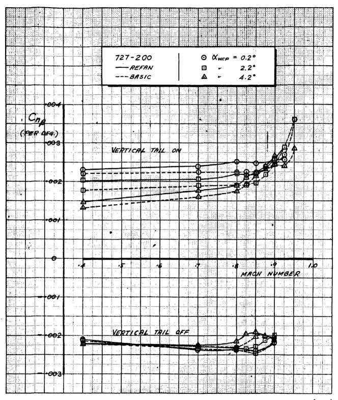
FIGURE 13. - EFFECT OF NASA REFAN NACELLES ON DIRECTIONAL STABILITY (Cng)
