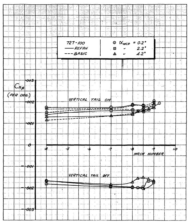
FIGURE 17. - EFFECT OF NASA REFAN NACELLES ON DIRECTIONAL STABILITY (CMB)
