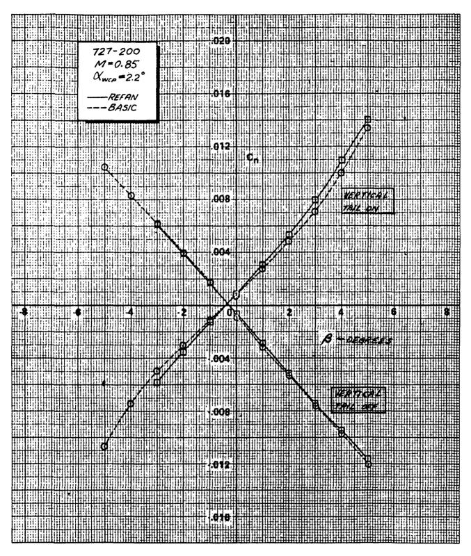
FIGURE 21. - EFFECT OF NASA REFAN NACELLES ON DIRECTIONAL STABILITY,
