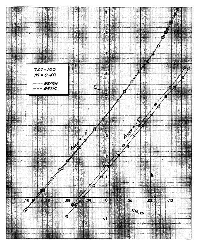
FIGURE 9. - EFFECT OF NASA REFAN NACELLES ON PITCHING MOMENT, 727-100, M = 0.40
