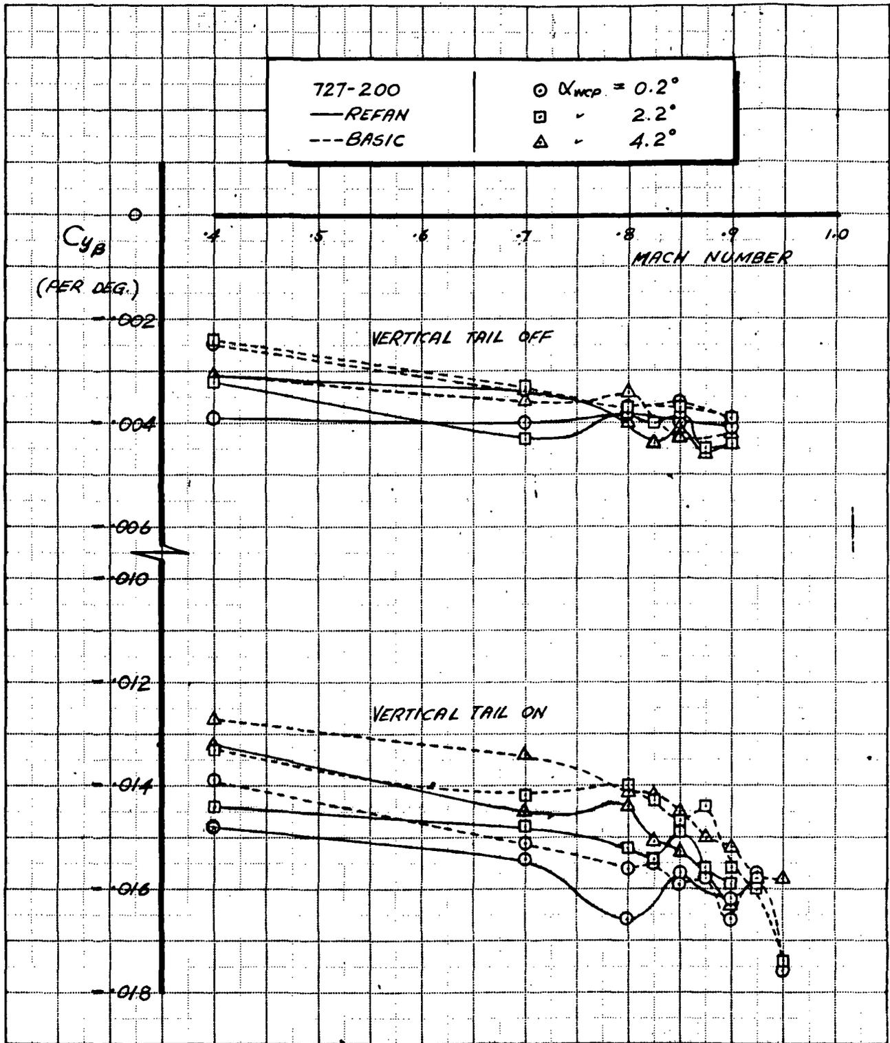
FIGURE 16. - EFFECT OF NASA REFAN NACELLES ON  $C_{y\beta}$ , 727-200
