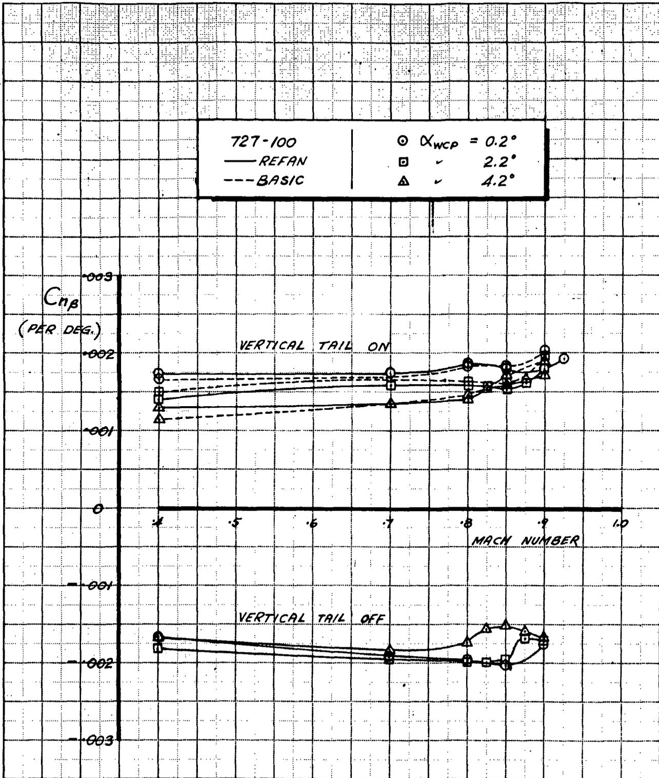
FIGURE 17. - EFFECT OF NASA REFAN NACELLES ON DIRECTIONAL STABILITY ( $C_{m\beta}$ )
