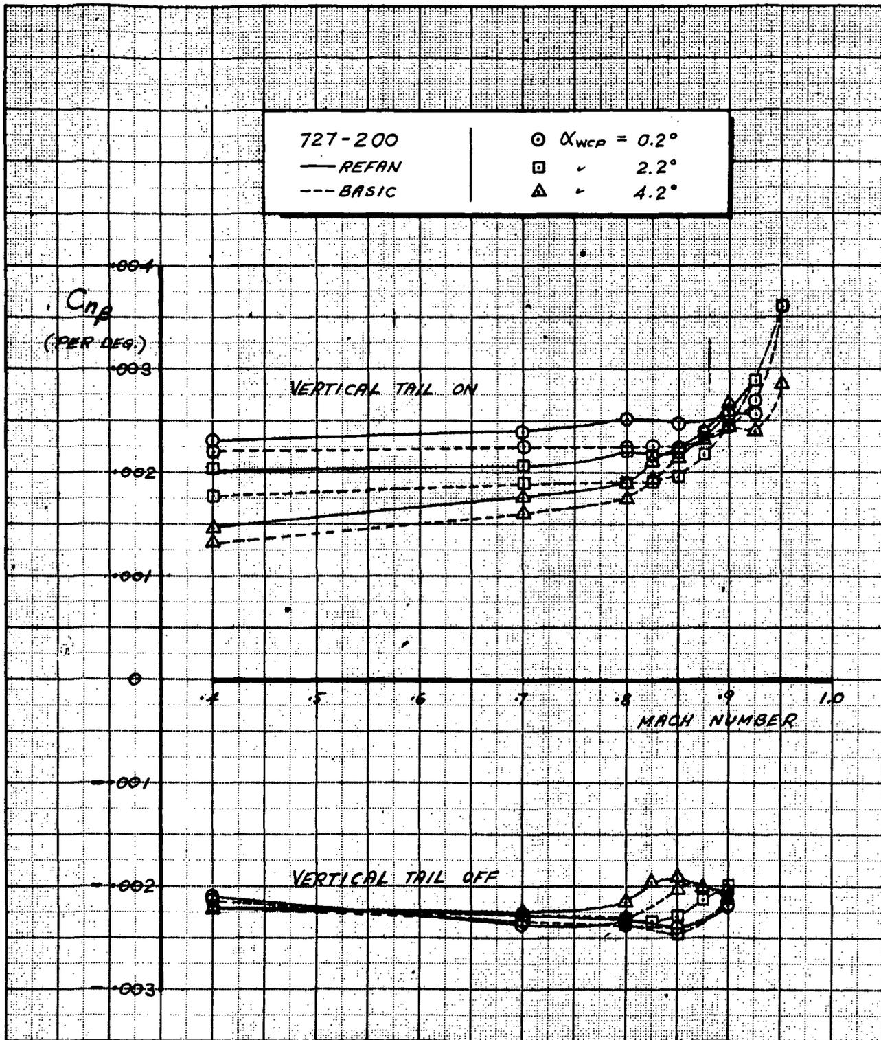
FIGURE 13. - EFFECT OF NASA REFAN NACELLES ON DIRECTIONAL STABILITY ( $C_{n\beta}$ )
