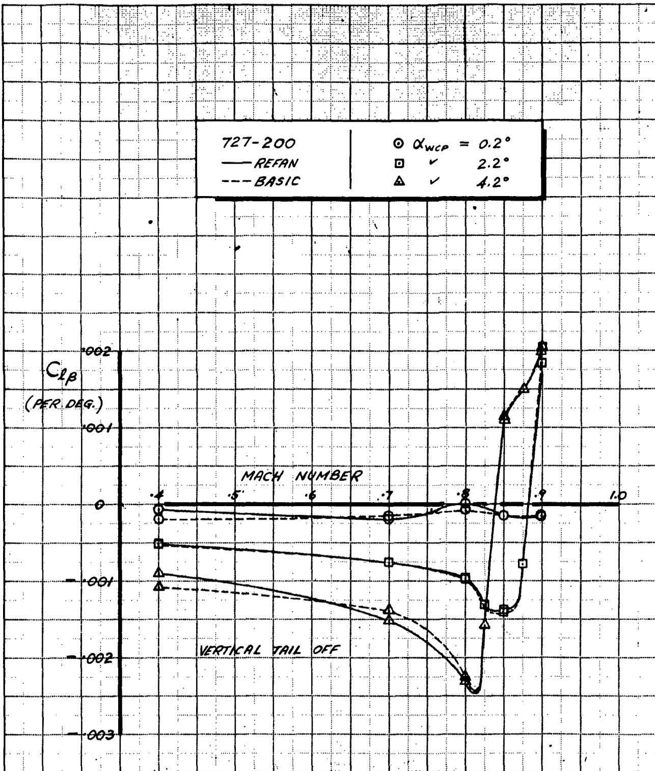
FIGURE 15. - EFFECT OF NASA REFAN NACELLES ON LATERAL STABILITY ( $C_{l\beta}$ )
