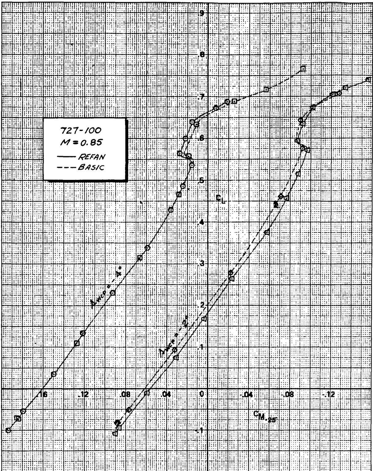
FIGURE 10. - EFFECT OF NASA REFAN NACELLES ON PITCHING MOMENT, 727-100,  $M = 0.85$
