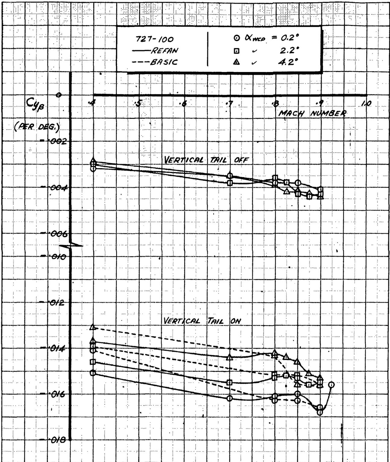
FIGURE 20. - EFFECT OF NASA REFAN NACELLES ON  $C_{y\beta}$ , 727-100
