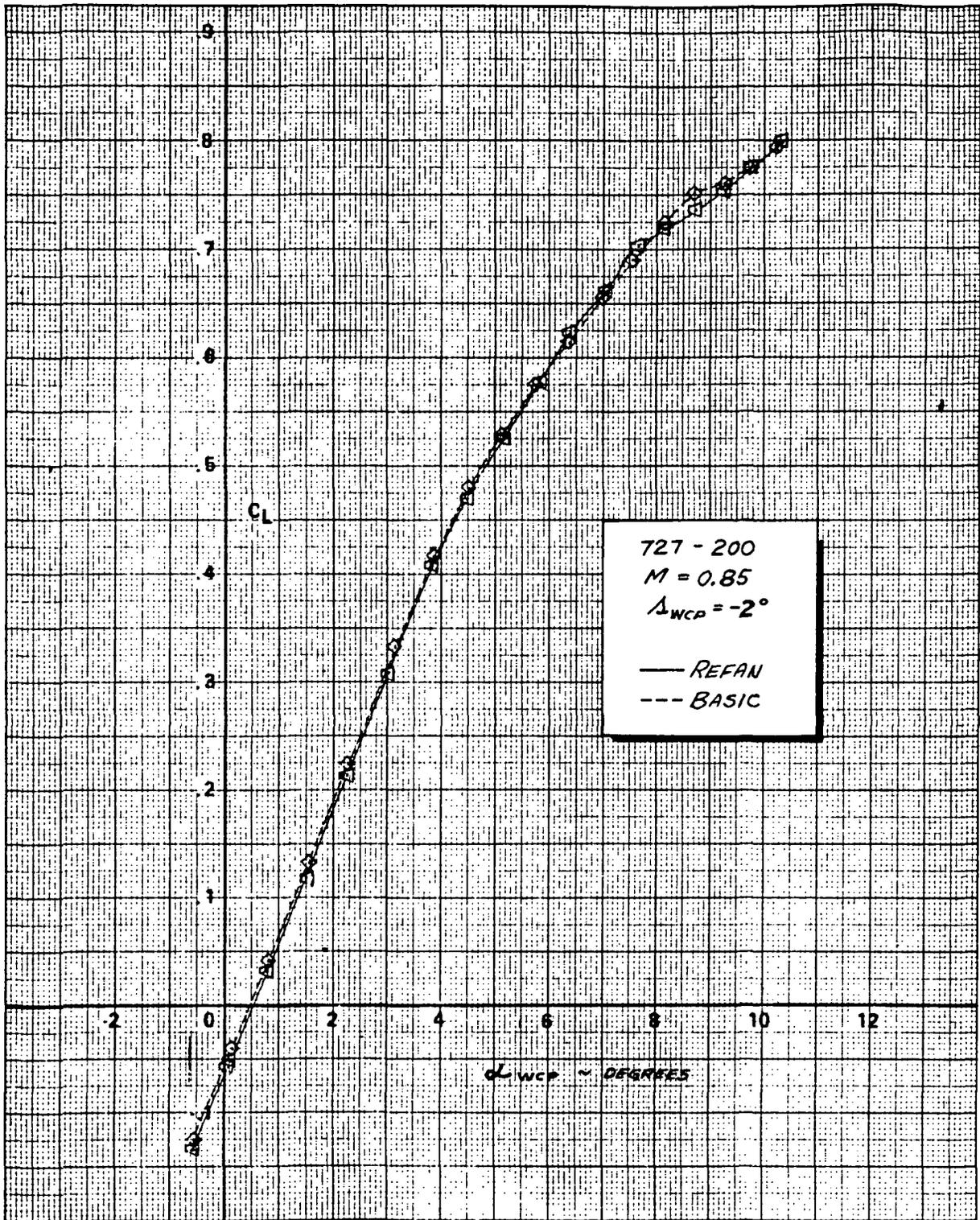
FIGURE 12.- EFFECT ON NASA REFAN NACELLES ON LIFT
