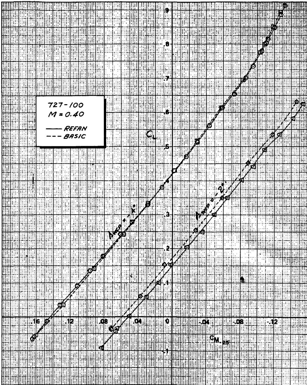
FIGURE 9. - EFFECT OF NASA REFAN NACELLES ON PITCHING MOMENT, T2T-100, M = 0.40
