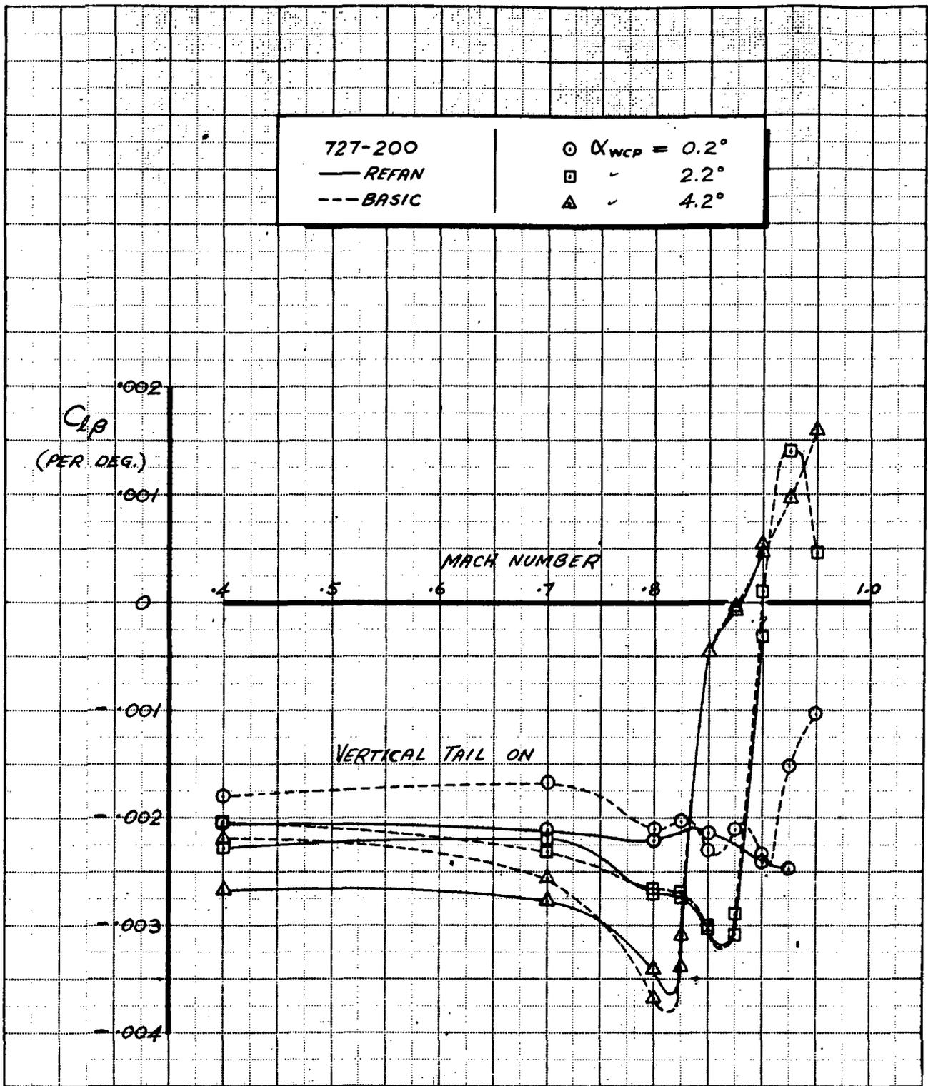
FIGURE 14. - EFFECT OF NASA REFAN NACELLES ON LATERAL STABILITY ( $C_{l_p}$ )
