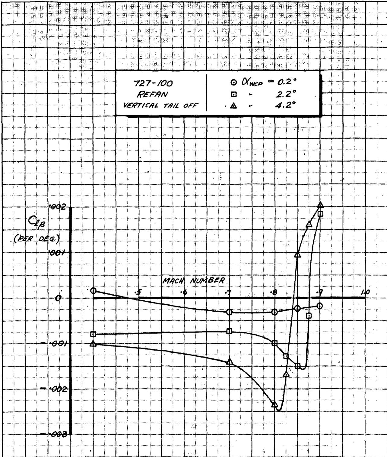
FIGURE 19. - 727-100 REFAN LATERAL STABILITY ( $C_{l\beta}$ ), VERTICAL TAIL OFF
