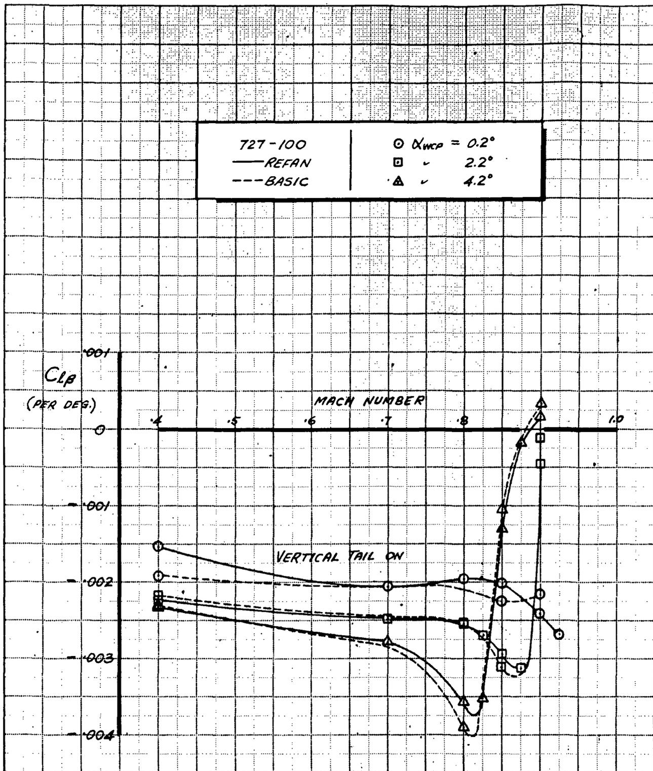
FIGURE 18. - EFFECT OF NASA REFAN NACELLES ON LATERAL STABILITY ( $C_{l\beta}$ ),
