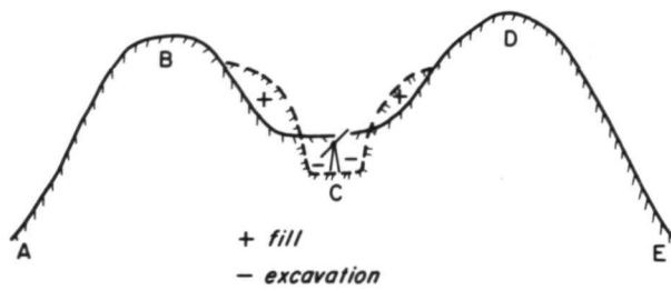
Fig. 9 Proposed type of terrain modification for the purpose of augmenting average wind speeds
