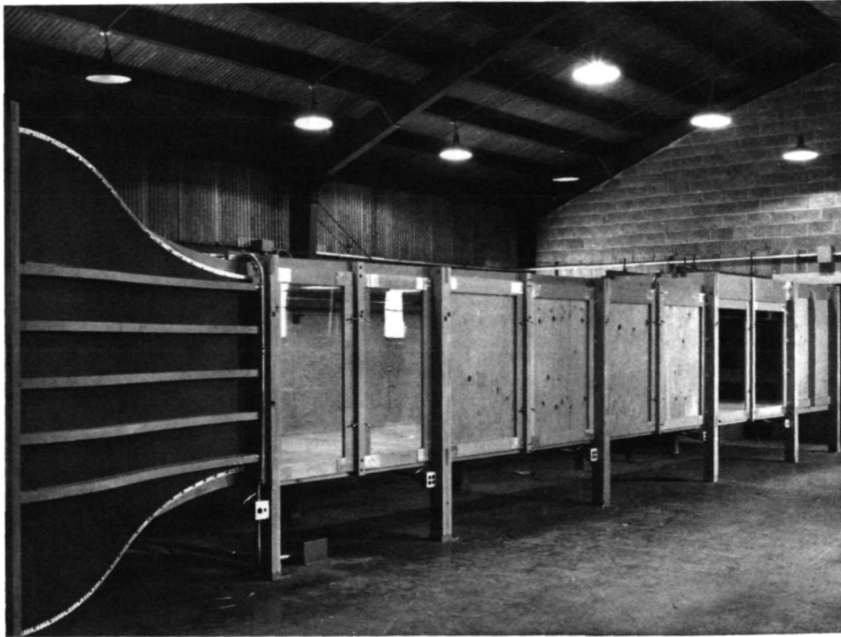
Fig. 8 The exterior of the test section of the wind tunnel; direction of air flow is from left to right.
