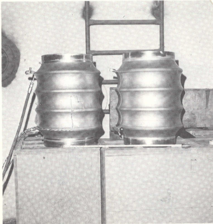
Figure 5-16. - Tension Membrane Jackets Welded to Dummy Inner Lines
