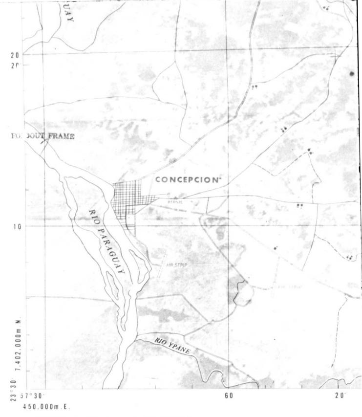
Prepared by the IAGS EROS team in the Panama Canal Zone, February 1974 as an initial photogrammetric experiment with SKYLAB photography (camera S190A Station 5) taken September 1973 Planimetric map features compiled by photogrammetric methods (WILD A9) Road classification and land mark features were extracted from 1.50,000 field classification data 1971. Authorization for use and distribution of this map was approved by the Paraguayan Government February 1974.
