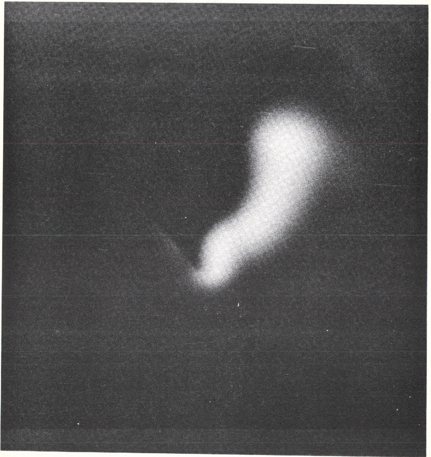
Figure 13. Photograph of the lithium trail of 16 September taken from the Convair 990 with the same film, filter and exposure as Figure 8. The useable field for the interference filter is only 7^\circ for the lithium resonance line at 6708\text{\AA} , and thus, only a portion of the trail is recorded.
