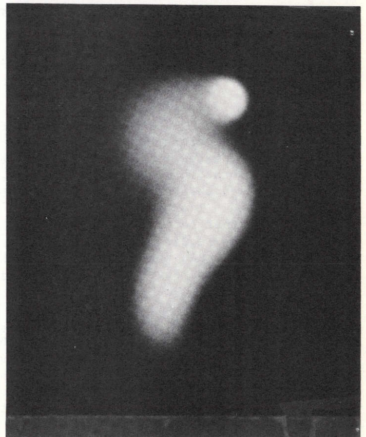
Figure 5. Photographs of the barium release of 16 September taken with the BIC triangulation cameras aboard the NASA Convair 990. The exposures are 1/10 sec at F/4 on Kodak 2485 film at a rate of one per second. The frames are at 1, 2, 3, and 4 seconds after barium release.
