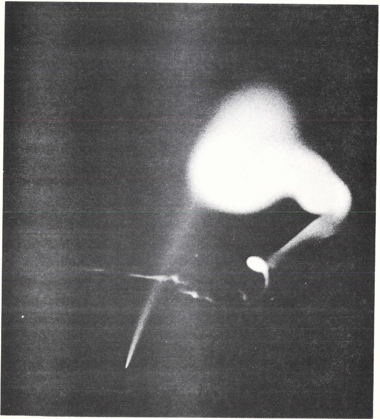
Figure 7. Photograph of the lithium trail taken with 70 mm cameras from the 14° side windows of the Convair 990. The exposure is 1/10 second at F/2.5 on Kodak 2475. The time is 4.5 minutes after launch of the rocket.
