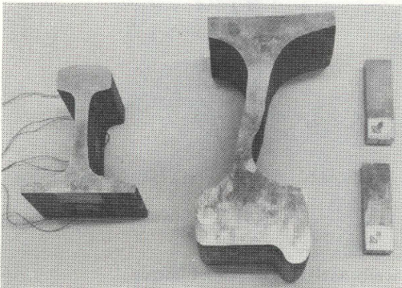
Test sections of a rail and railcar wheel prior to a test.
