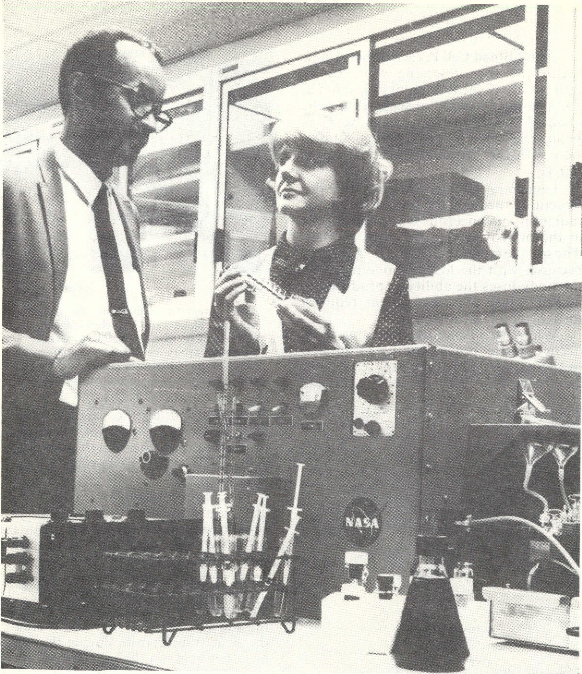
Scientists at the NASA Goddard Space Flight Center have developed a rapid technique for determining the presence of bacteria in biological fluid samples. The early prototype of the instrument shown provides an answer in 15 minutes as compared to 48 to 72 hours required by the conventional laboratory method.
