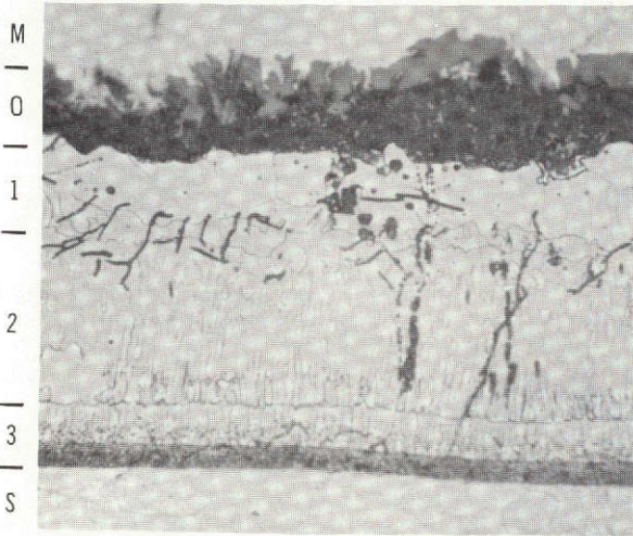
(a) R512E coated Cb-752 after 5 cycles.
