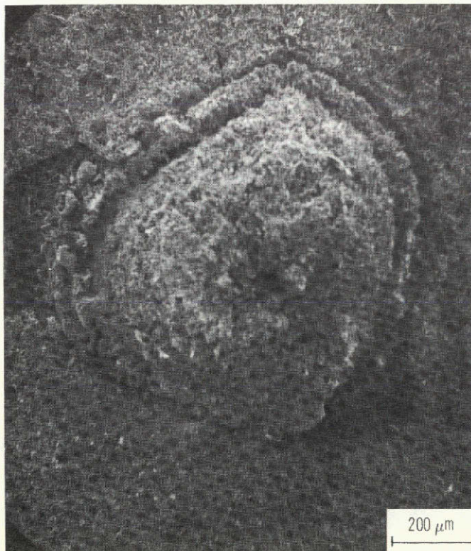
Figure 11. - Scanning electron micrograph showing plugging of 0.092-centimeter through-hole defect in R512E coated FS-85 with substrate oxide after five plasma arc exposure cycles at 1390° C. Scanning electron microscope conditions: 7 picoamperes, 25 kilovolts.
