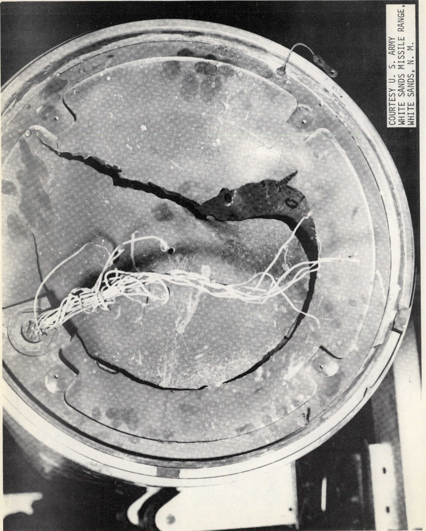
Figure 6-2. Post-Flight HCO CALROC 21.021 Payload, Vacuum Dome Rupture.
