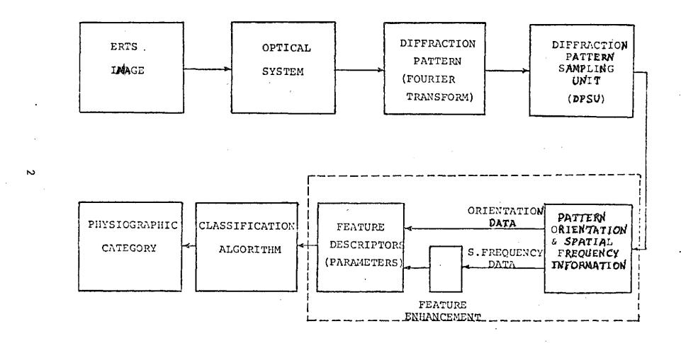
Figure 1. Block diagram of optical processing and pattern recognition system.
