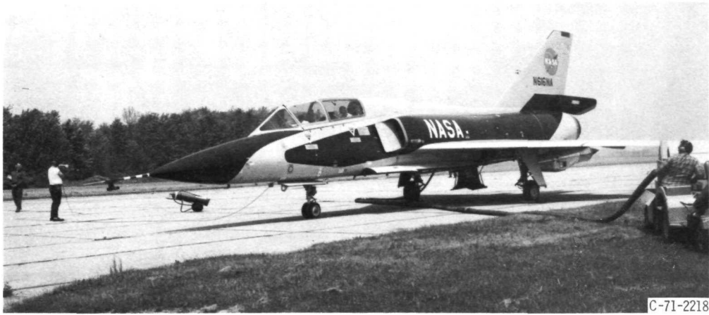
Figure 11. - Location of external source of cooling air for static tests.
