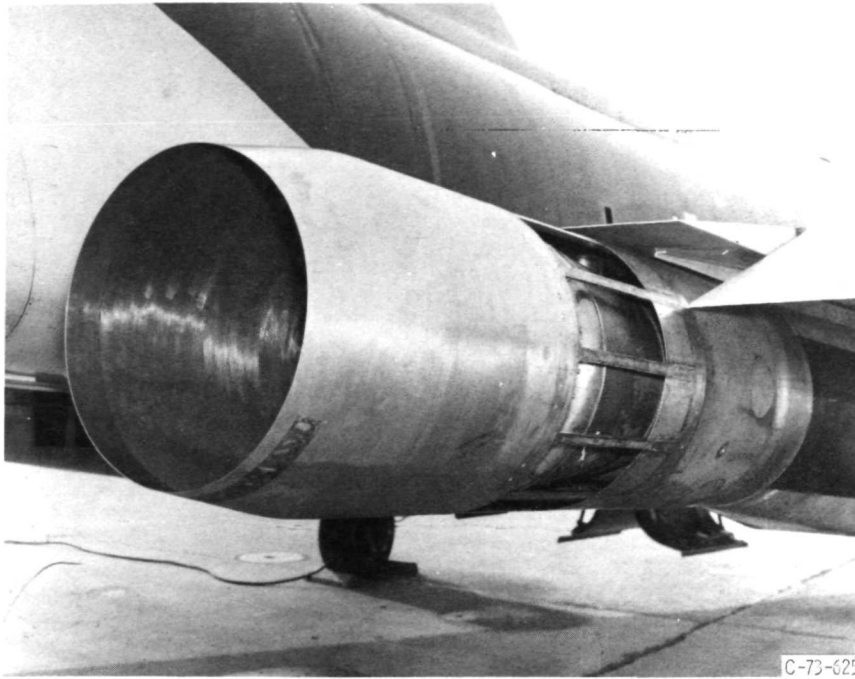
(e) 104-Tube nozzle with acoustic shroud; overall view.
