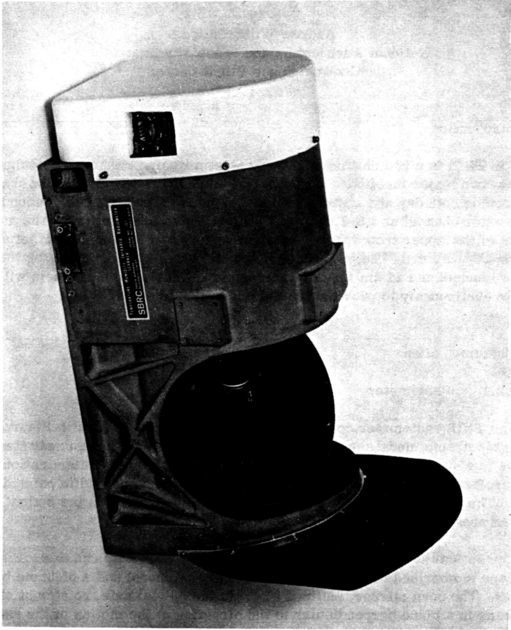
Figure 2-1. The Temperature Humidity Infrared Radiometer
