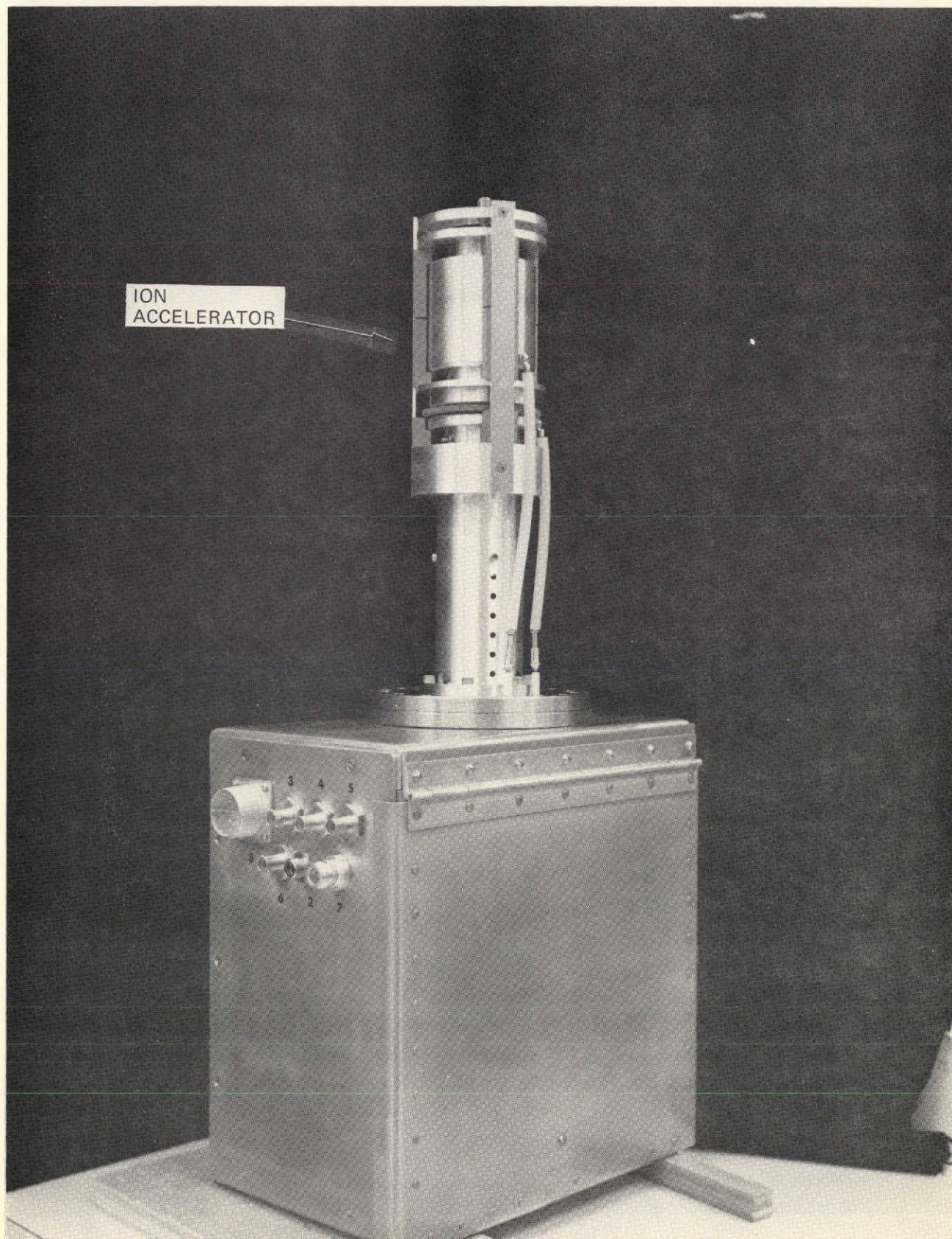
Figure 17: PLASMA GENERATOR ENCLOSURE WITH ION ACCELERATOR ATTACHED
