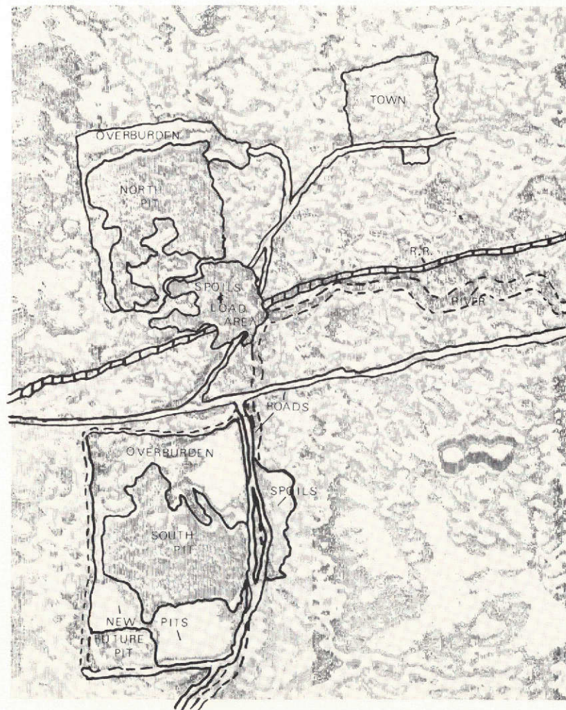
Figure 3b. Interpreted isodensity contour map compiled from an isodensitracing of the S-190B photograph shown in 3a.
