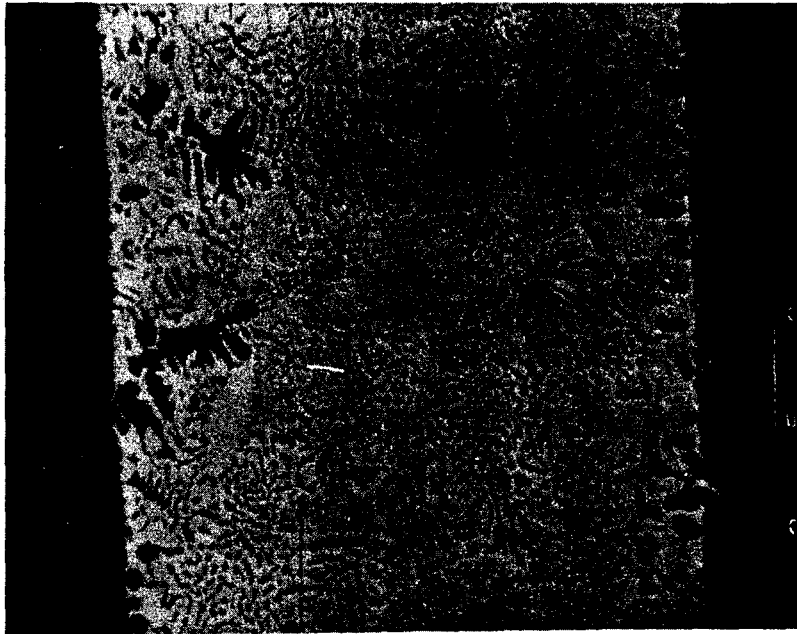
FIG. 19 SCANNING ELECTRON MICROGRAPH OF SLN-4-20mm - 120° SHOWING THE TWO KINDS OF PRIMARY PHASES. (250X)
