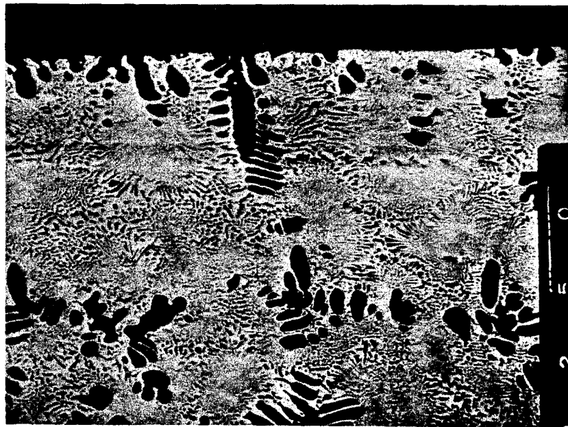
FIG. 34 SCANNING ELECTRON MICROGRAPH OF MCS 6-11.7mm - 260° SHOWING THE NORMAL EUTECTIC ADJACENT TO STAINLESS SURFACE (AT TOP). (500X)
