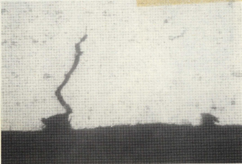
Figure 3.- These photomicrographs show polished and etched cross sections of the I.D. away from the leak site. The shallow, open flaws result from the forming operation while the deeper tighter flaws are fatigue cracks. It is obvious that the forming tears provide enough stress concentration to initiate fatigue cracks. Magnification: 500X
