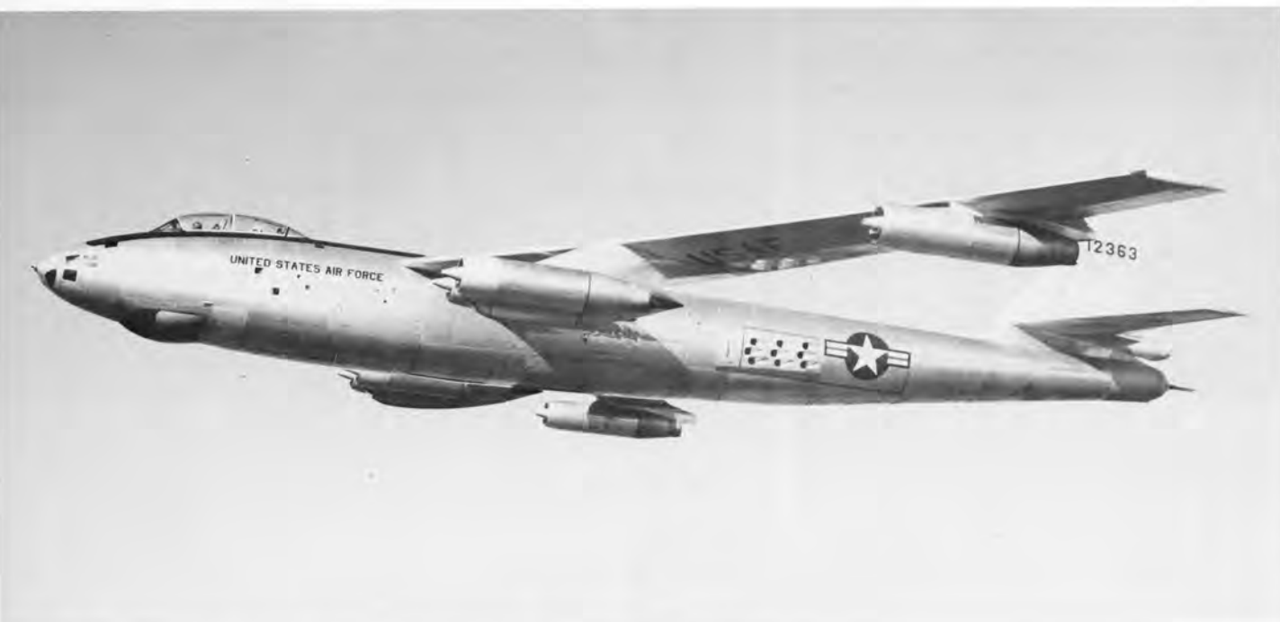
BOEING B-47E: Its thin, swept-wing layout influenced later designs.
