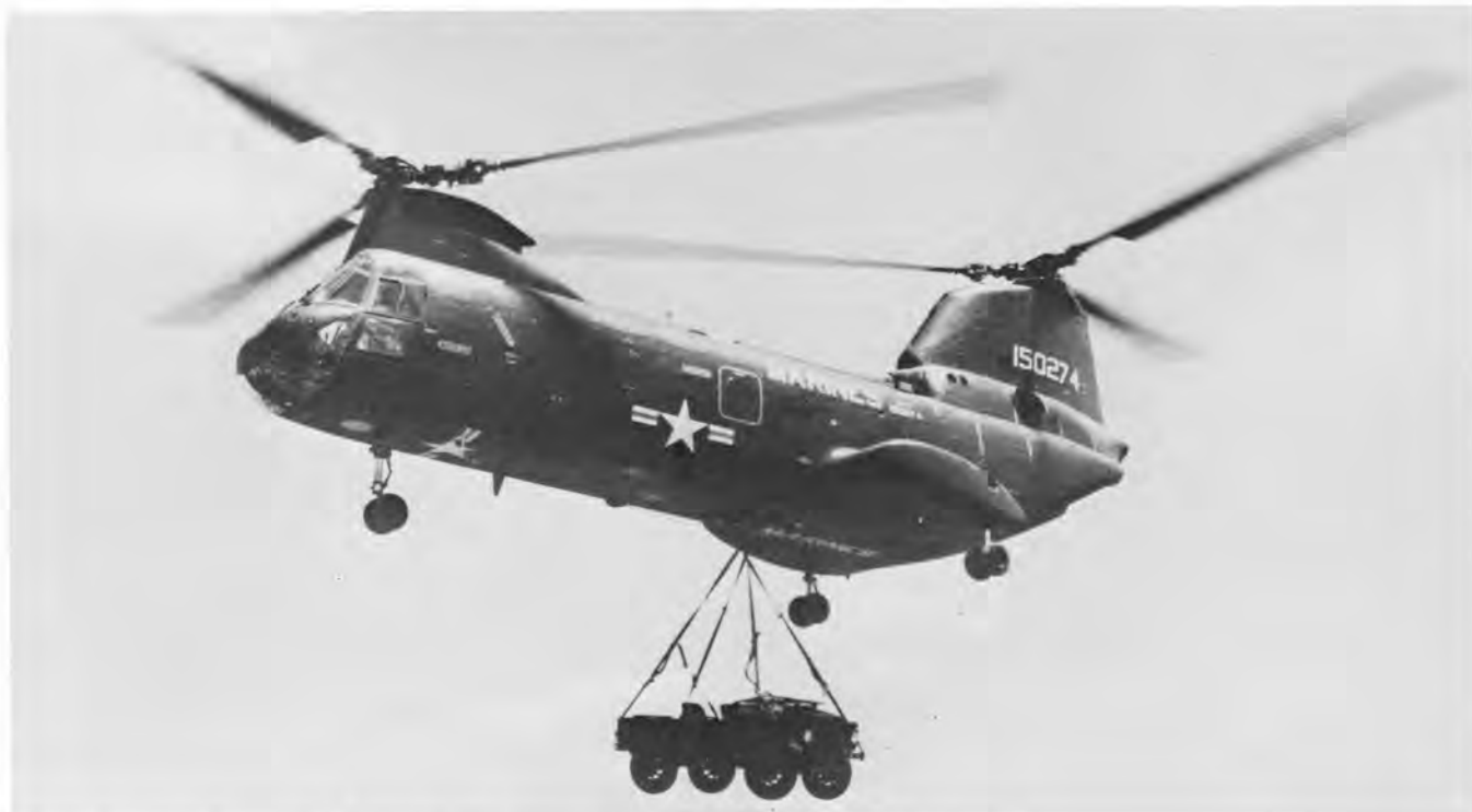
VERTOL CH-46A: The "Sea Knight" was designed to move USMC combat elements.
