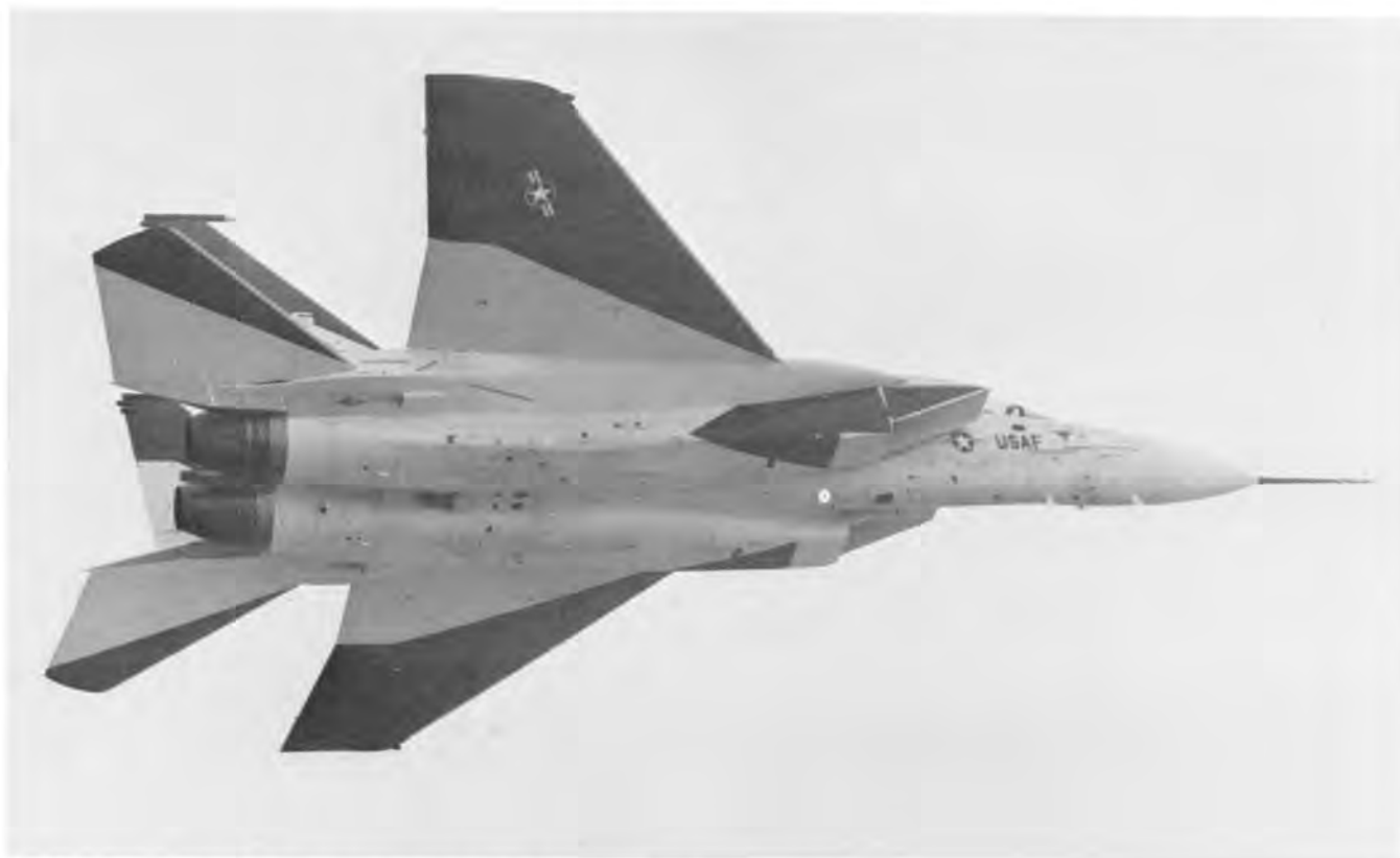
McDONNELL-DOUGLAS F-15A: Its large wing increases its maneuverability.
