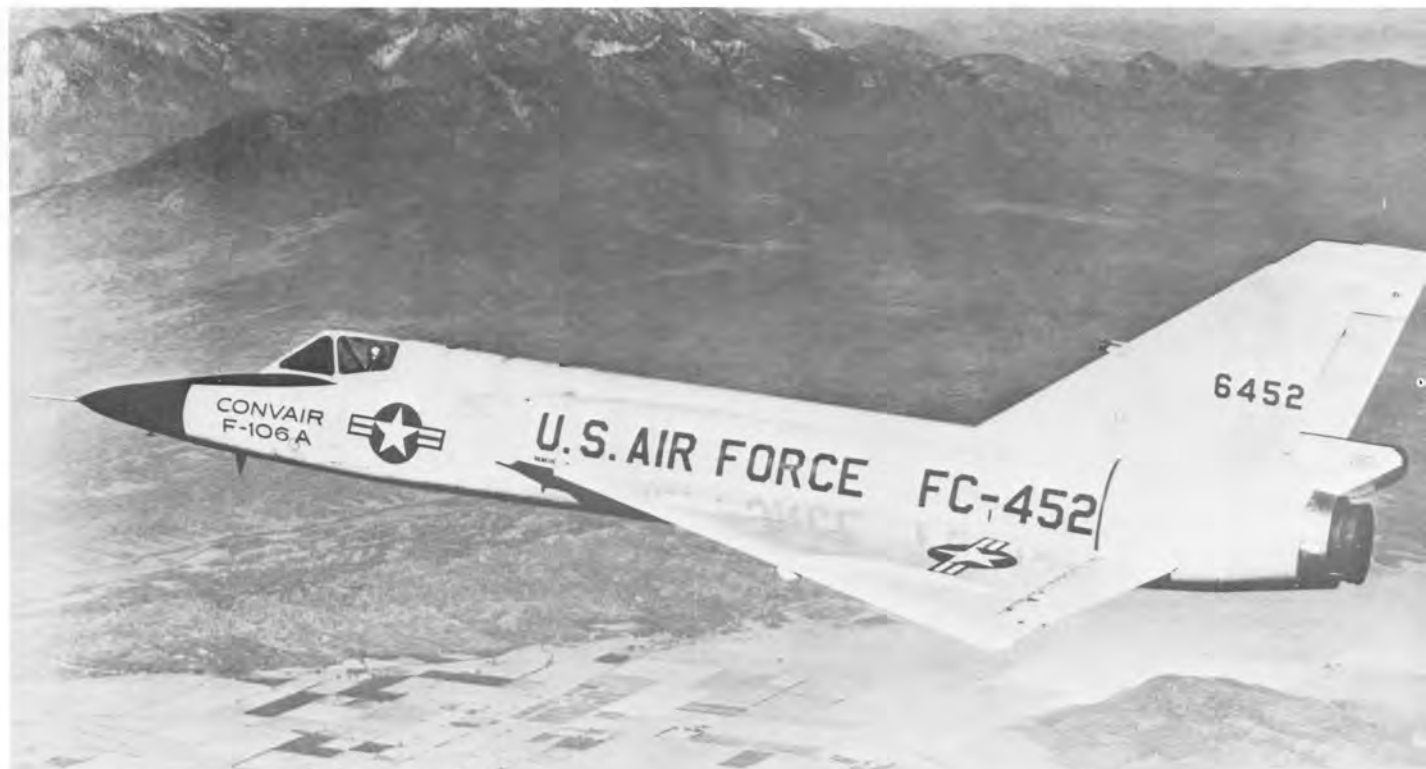
CONVAIR F-106A: The pilot is along for the ride in this automatic interceptor.
