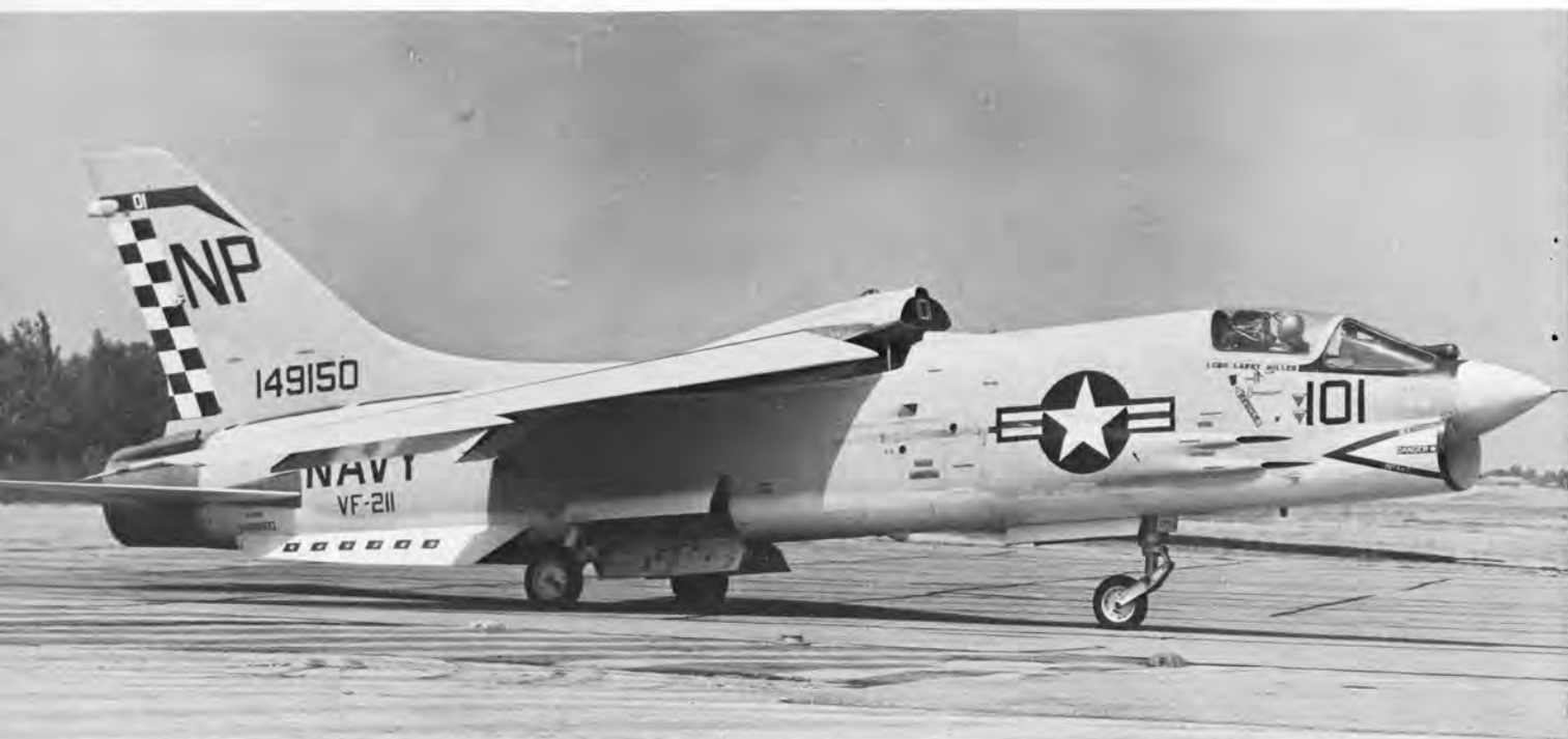
VOUGHT F-8E: The area rule reduced the "Crusader" transonic drag.
