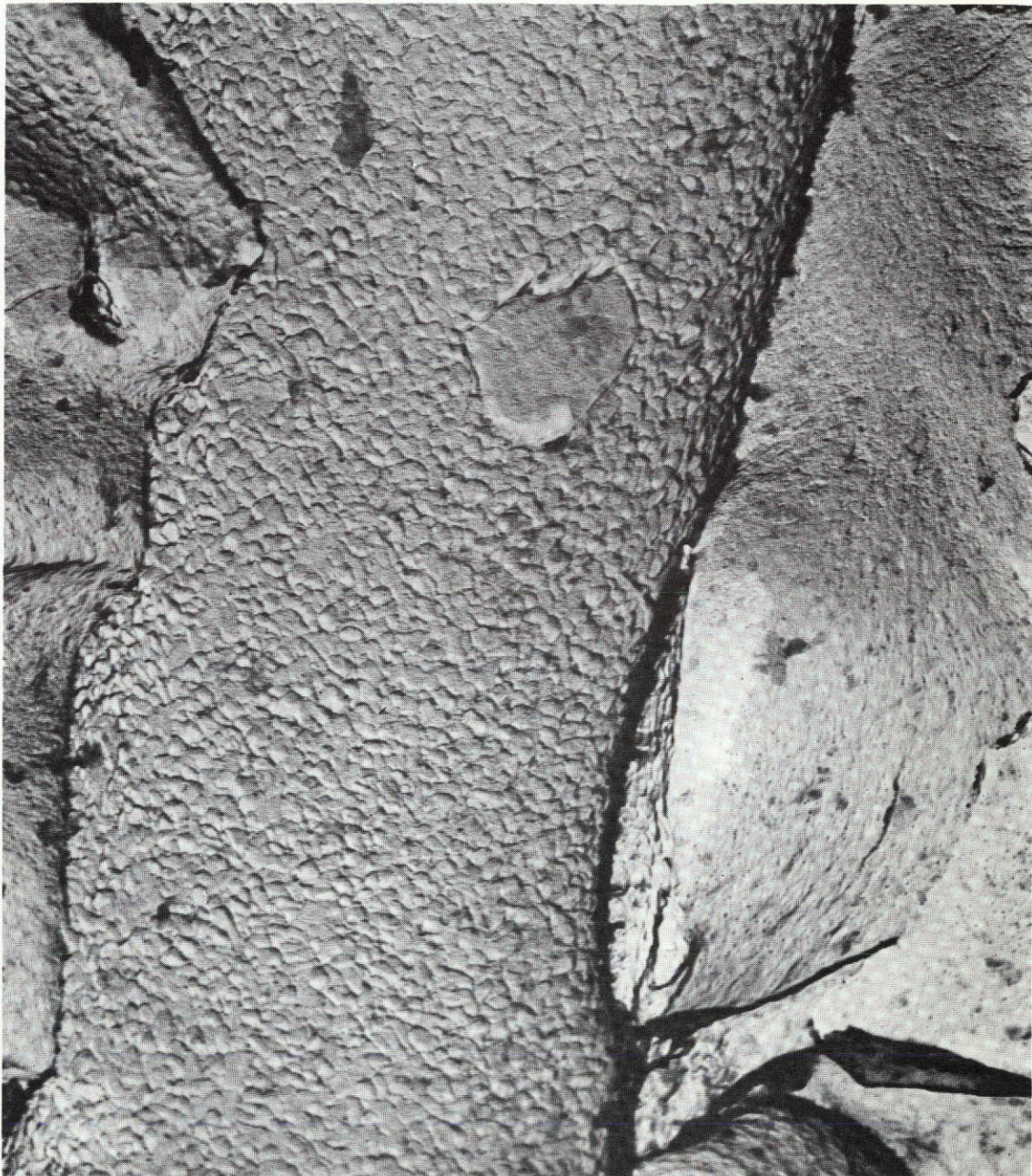
Figure 16. Blown Mullite Fiber Following 1259C Thermal Cycling (Run F-4)
