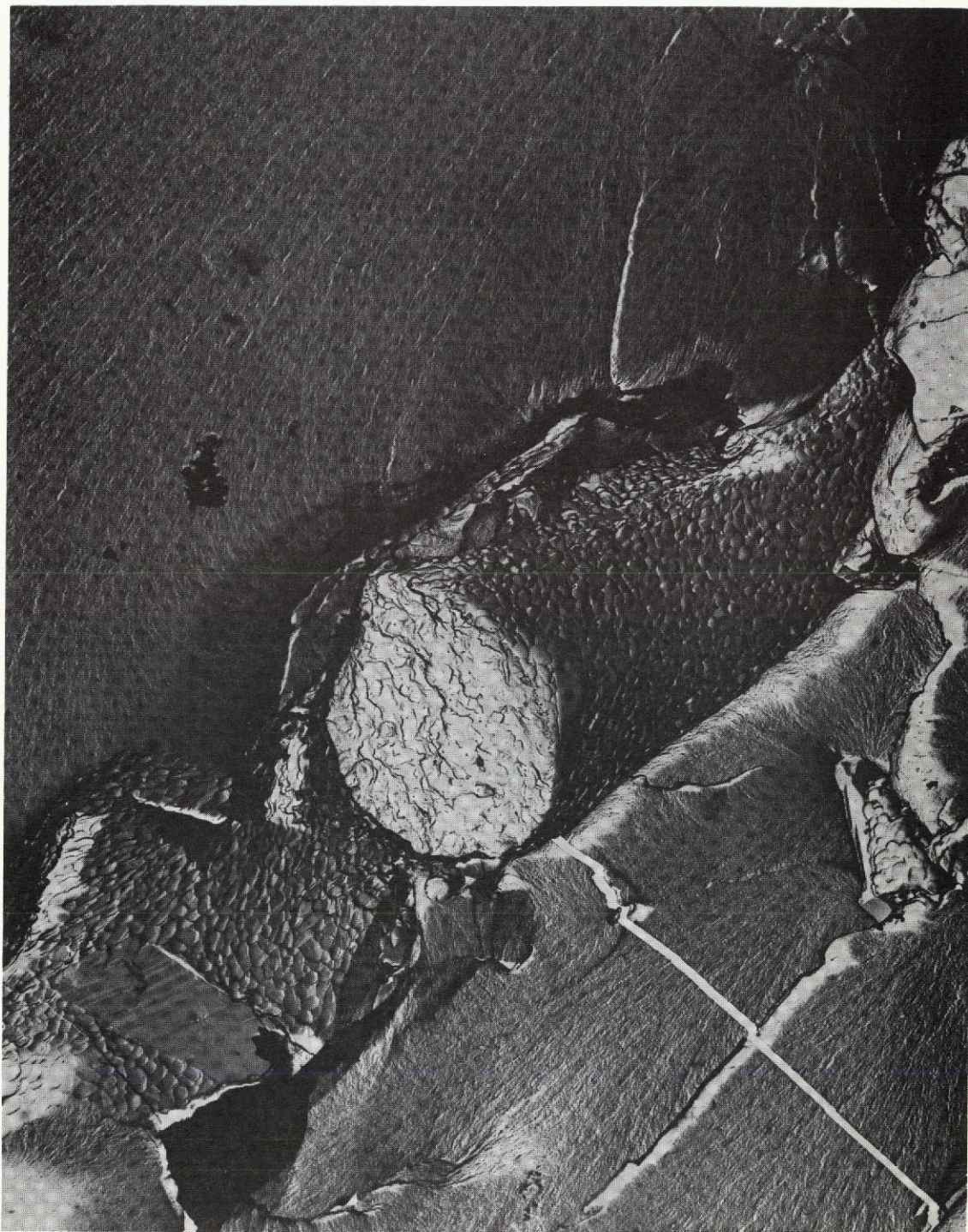
Figure 30. Mullite Fiber With 0.10% MgO Added, After 1371C Thermal Exposure
