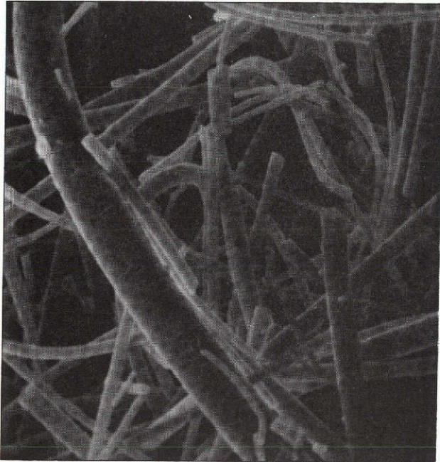
Figure 28. Mullite Fiber With 5% CrO 3 Added, After 1371C Thermal Exposure
