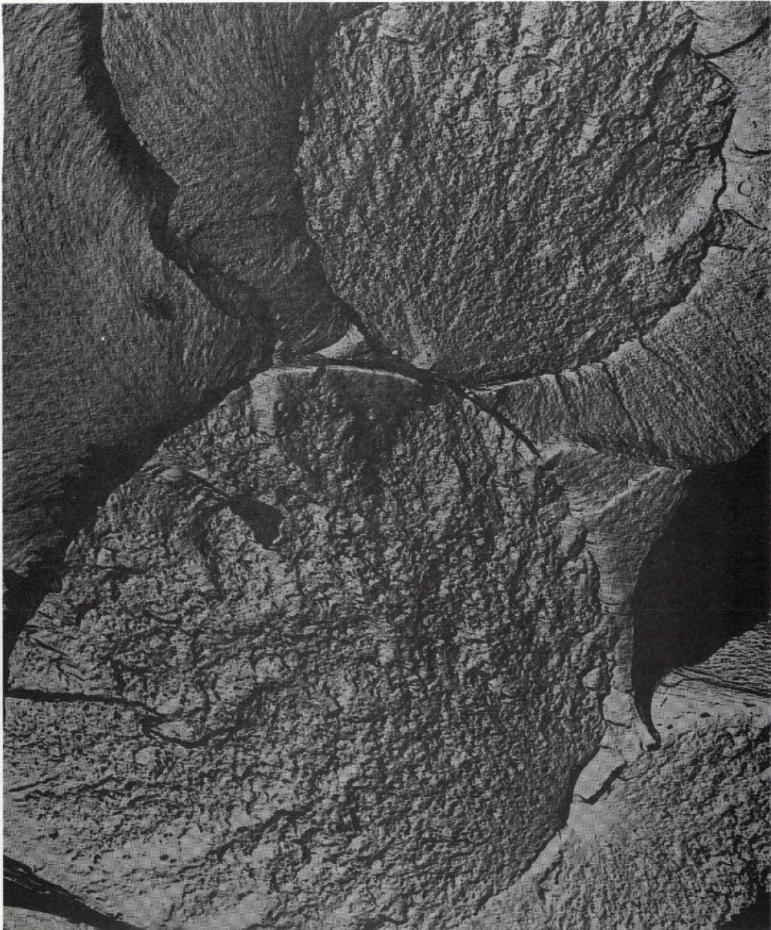
Figure 24. Fiber From 10-Pound Lot Showing No Apparent Crystallinity
