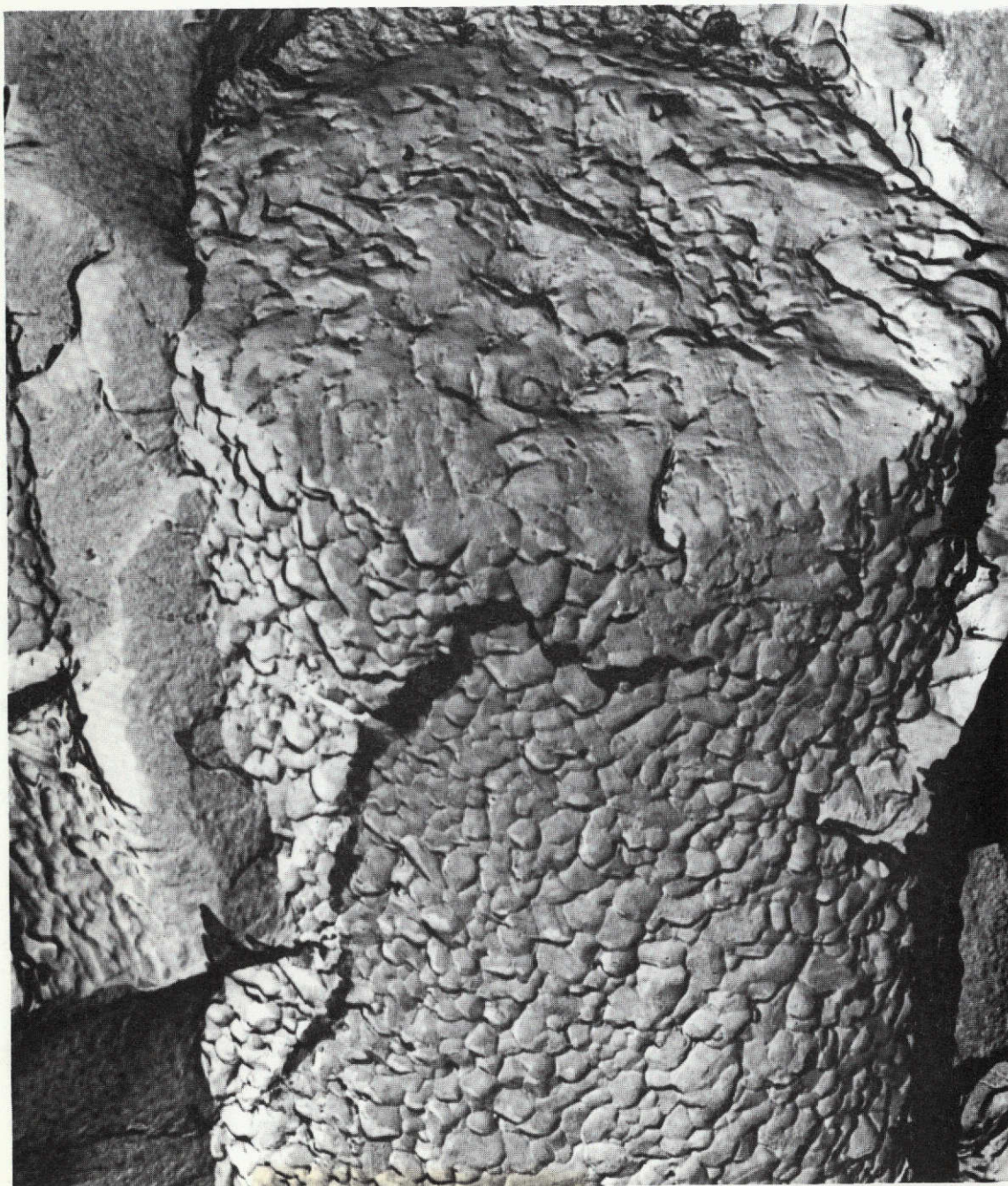
Figure 17. Blown Mullite Fiber Following 1371C Exposure (Lot F-1)
