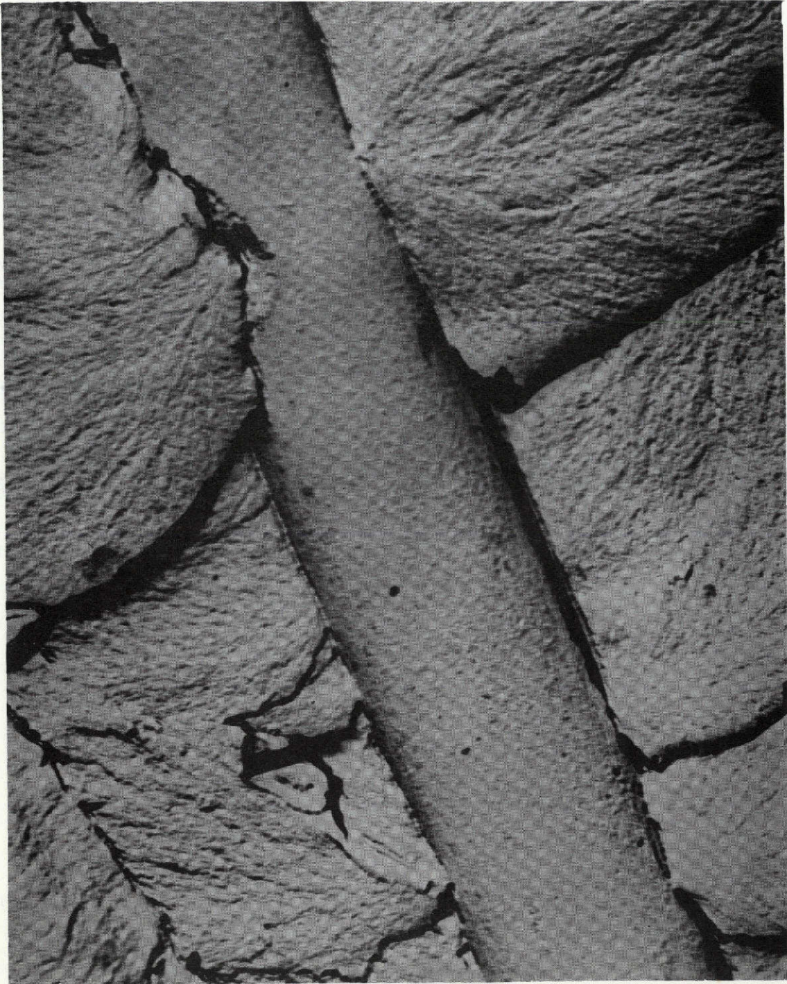
Figure 10. Surface of DE-2 As-Manufactured Fiber
