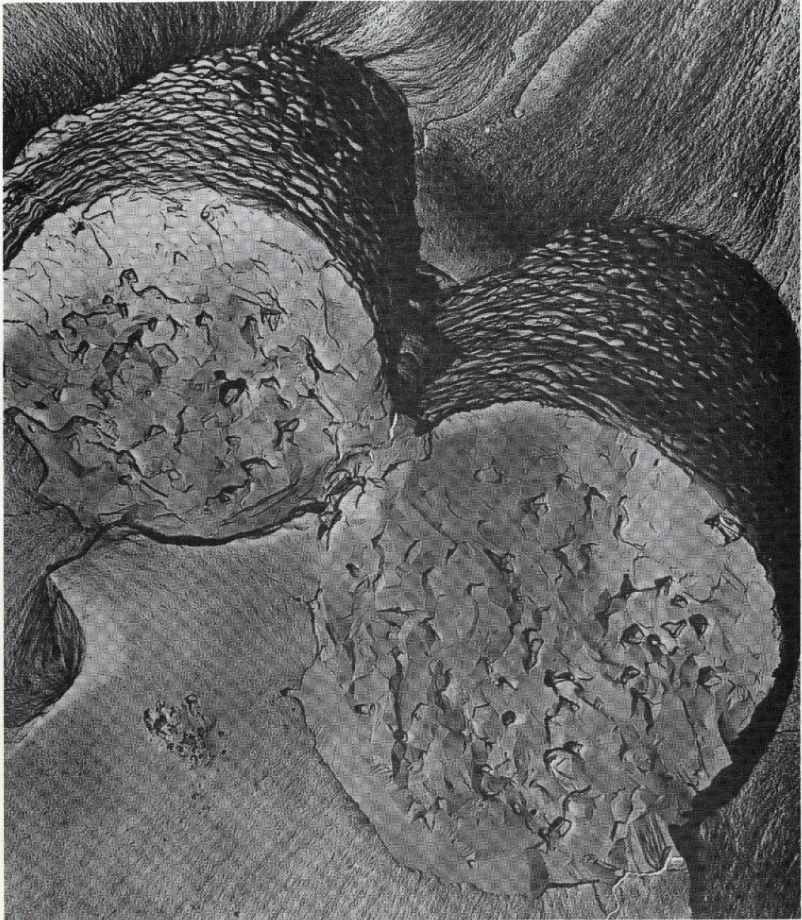
Figure 29. Mullite Fiber After 1425C Thermal Exposure
