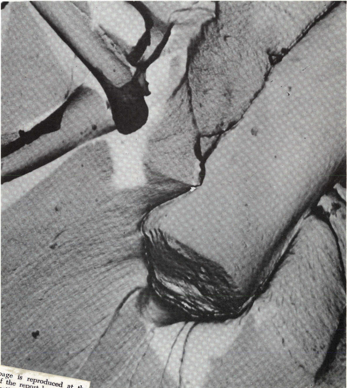
Figure 11. Surface of DE-9 As-Manufactured Fiber
