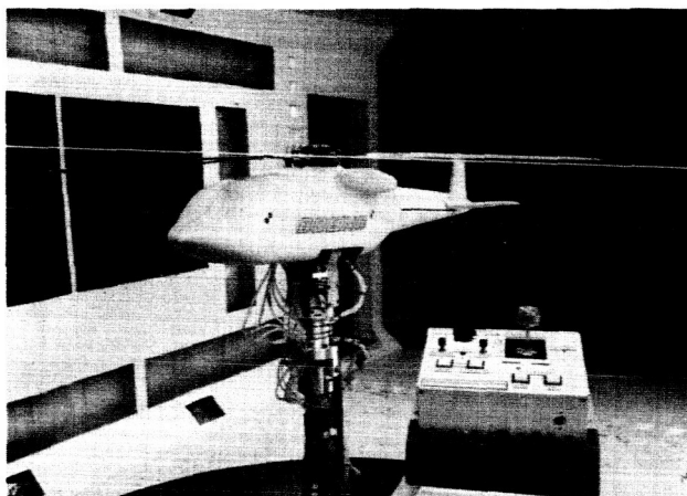
Figure 1. Dynamic Model Helicopter With 5.5-Foot-Diameter Single Rotor
