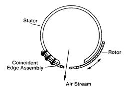
The improved nozzles have been used for hot (177°C) air at 414 kN (60 psig) pressure. Higher pressures are possible with provision for structural integrity.
