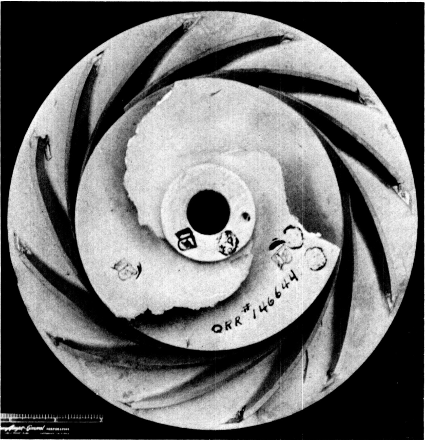
FIGURE 16.— Typical impeller blade failure.
