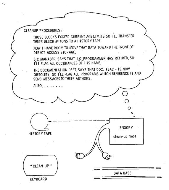
Finite direct-access storage plus a rapid turnover in relevant "facts" will require periodic "cleaning" of the data base. Obsolete data will be dumped onto history tapes in a manner suitable for later recovery if necessary. Additional mechanizable procedures of system management may be implemented.
