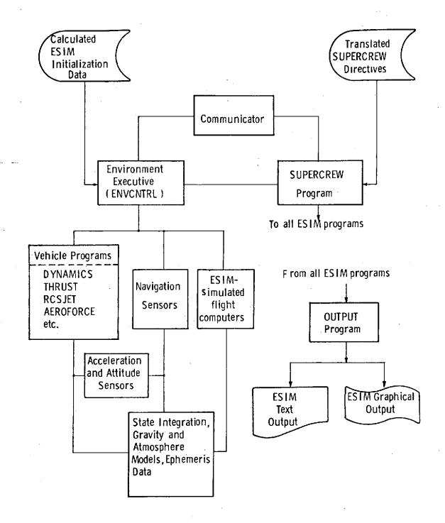
Figure 4-4. External-environment Simulator (ESIM)
