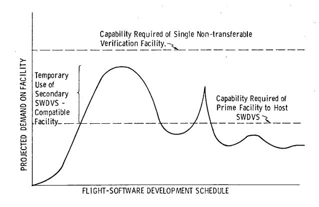
Figure 1-3. Alternate Methods of Responding to Projected Demand on the SWDVS Facility.
