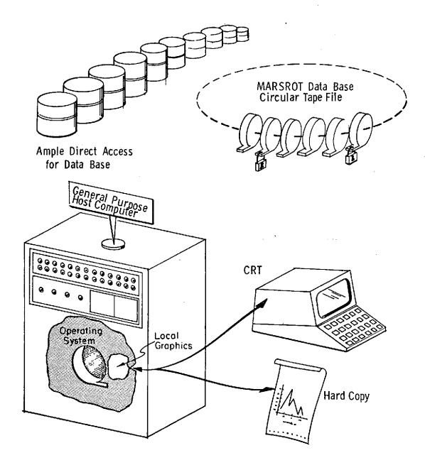
The SWDVS is hosted on a general purpose computer facility consisting of hardware and the necessary software to interface with that hardware.
