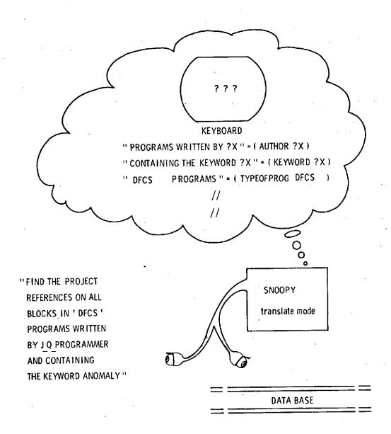
Operation in retrieval mode can become complex as the "descriptions" and "facts" become numerous and diverse. For this reason, SNOOPY assists users by providing a translation (preprocessing) capability. The input to SNOOPY is a limited-vocabulary, simple-grammar English; the output is the equivalent "descriptions", formatted for direct execution by the retrieval program.
