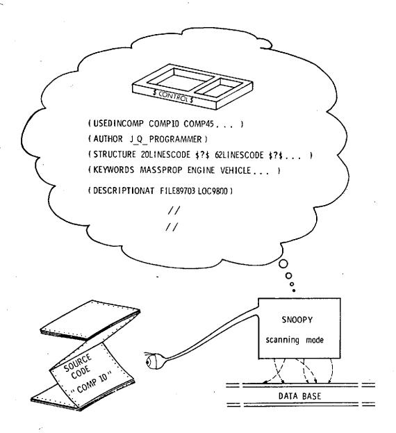
Anumber of block-specific, programmer-generated "facts" are scanned, catalogued, and stored in a "descriptor" portion of the SWDVS data base. These facts can be imbedded in the program, itself, transferred from the operating system, or typed in at consoles. To facilitate later retrieval, SNOOPY utilizes the list structure, a high degree of redundancy, and extensive cross-referencing.
