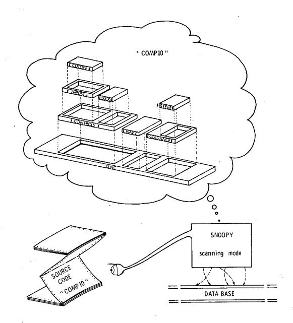
SNOOPY scans all source code at compile and recompile time, searching "blocks" as specified by the programmer. Names are assigned to each block (e.g., CONTROL) and the structure within the specific compilation is recorded. (See Figure 2-2 in the Scenario.)
