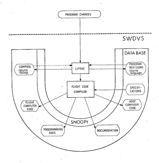
Figure 3-2. Software Design Functional Diagram
