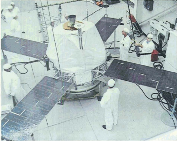
Mariner spacecraft being readied for launch. White shroud protects spacecraft mechanisms. Television cameras and other instruments are out of sight at the bottom. Solar panels are extended, and technicians indicate the scale of the spacecraft. (Jet Propulsion Laboratory)
