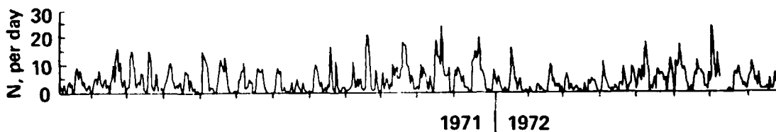
Figure 3.— Moonquake activity, recorded by the Apollo 14 passive seismic experiment (from Latham et al. , 1973), for the time period February 7, 1971 to July 27, 1972. Times of peak activity occur when the Moon is nearest to the Earth in its orbit (perigee) and farthest from the Earth (apogee).
