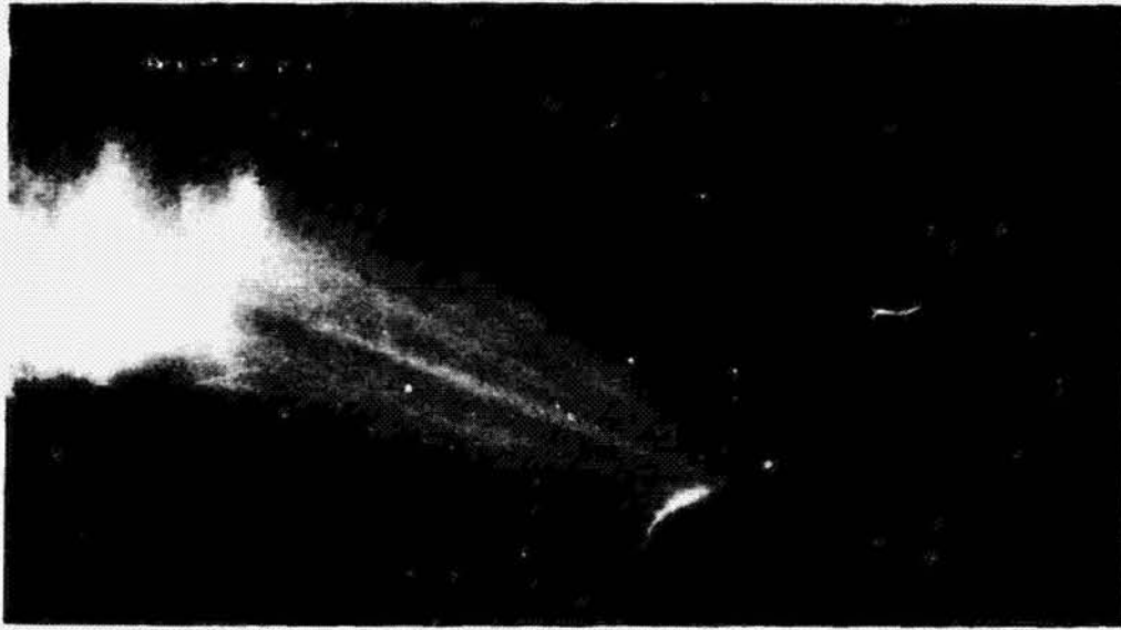
Fig. 5. An open shutter photograph of the luminosity produced by a hypervelocity impact against quartz sand. Projectile trajectory is from right to left at an angle of 30^\circ to the target surface. Note that the long streamers of high-speed incandescent material jetted out by the collision have produced secondary impacts and incandescence on the (left) side of the vacuum chamber. 30 caliber lexan projectile, weight 0.3 gram; 6.5 km/sec impact velocity.
