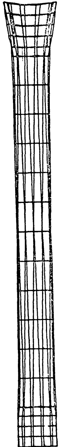
(c) LONGITUDINAL MODE SHOWING SOME TOR- SION. 196.1 Hz
