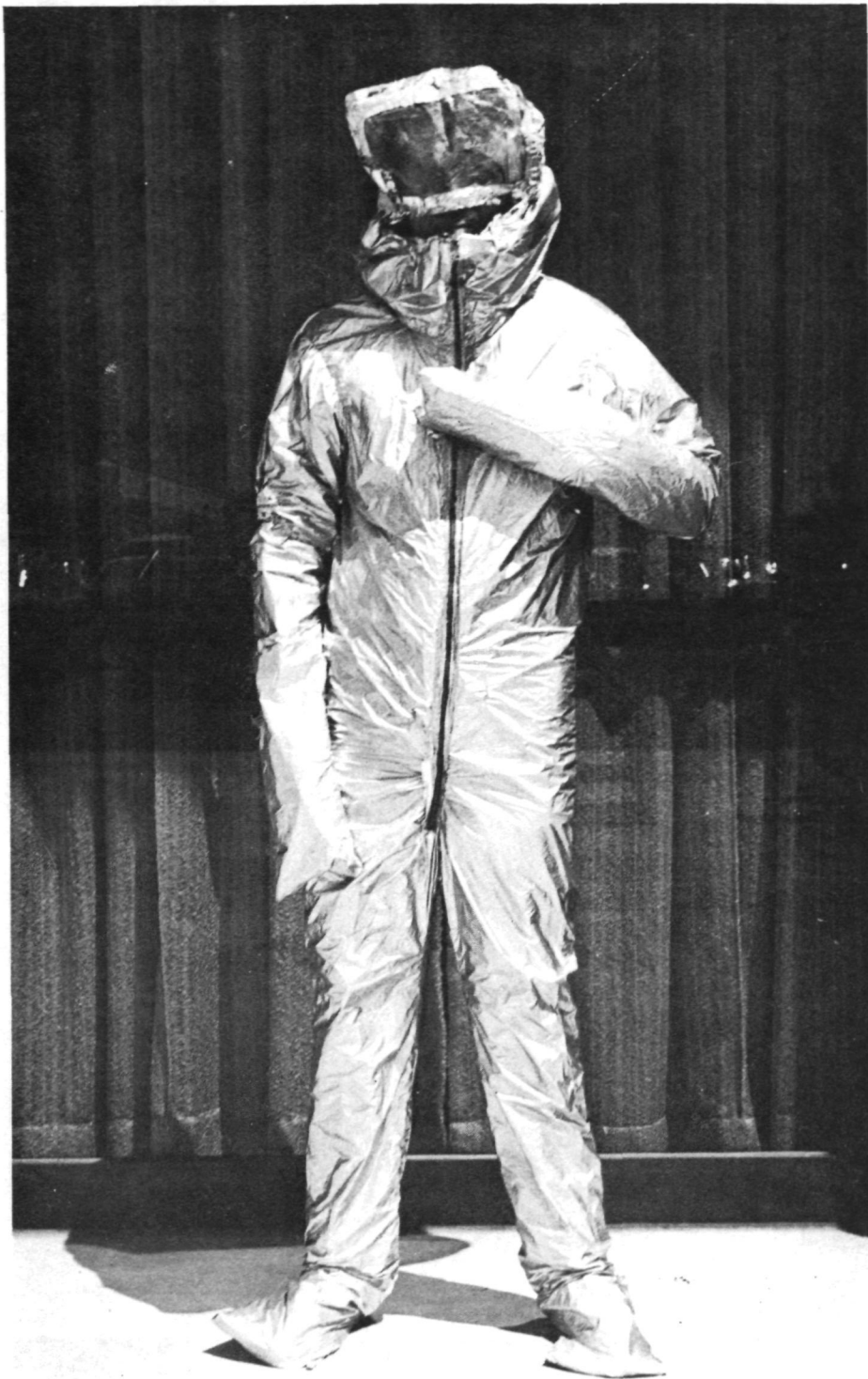
Figure 4 - Emergency Survival Suit of Reflective Insulating Films
