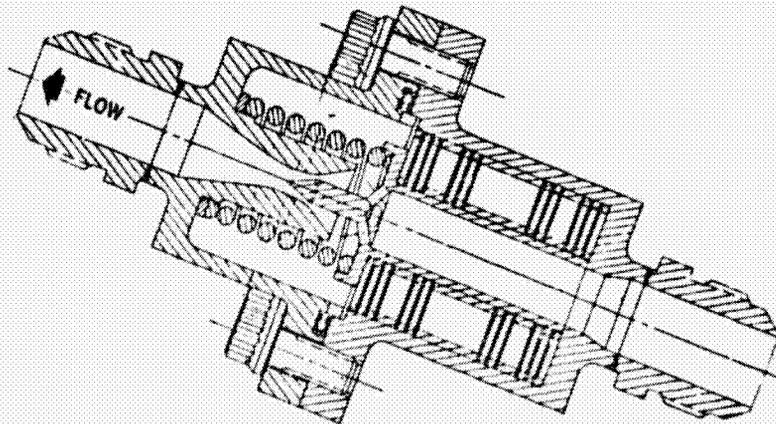
of construction were 300 series of stainless steel for all parts except the flexure reference coil spring. These were made from Inconel 718 and Type 302 stainless steel, respectively. The flexure assembly was a brazed assembly.
