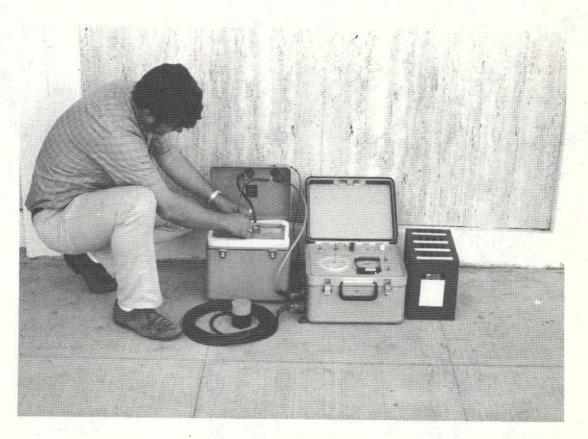
Figure 2. Equipment used in DSC installations (from left, DCP electronics, event counter, 1 year battery)
