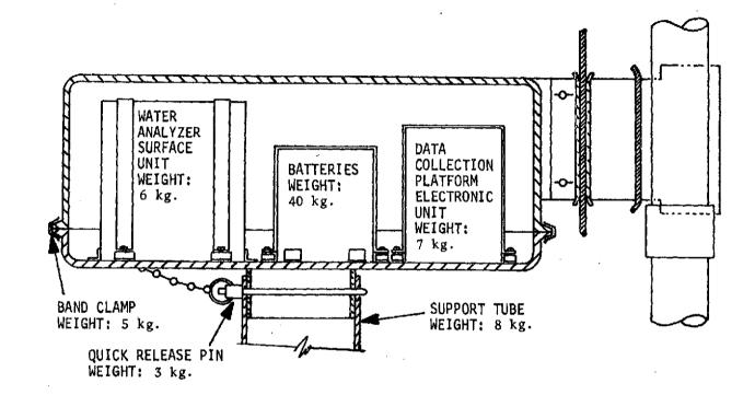
Figure 2. Buoy cross section
