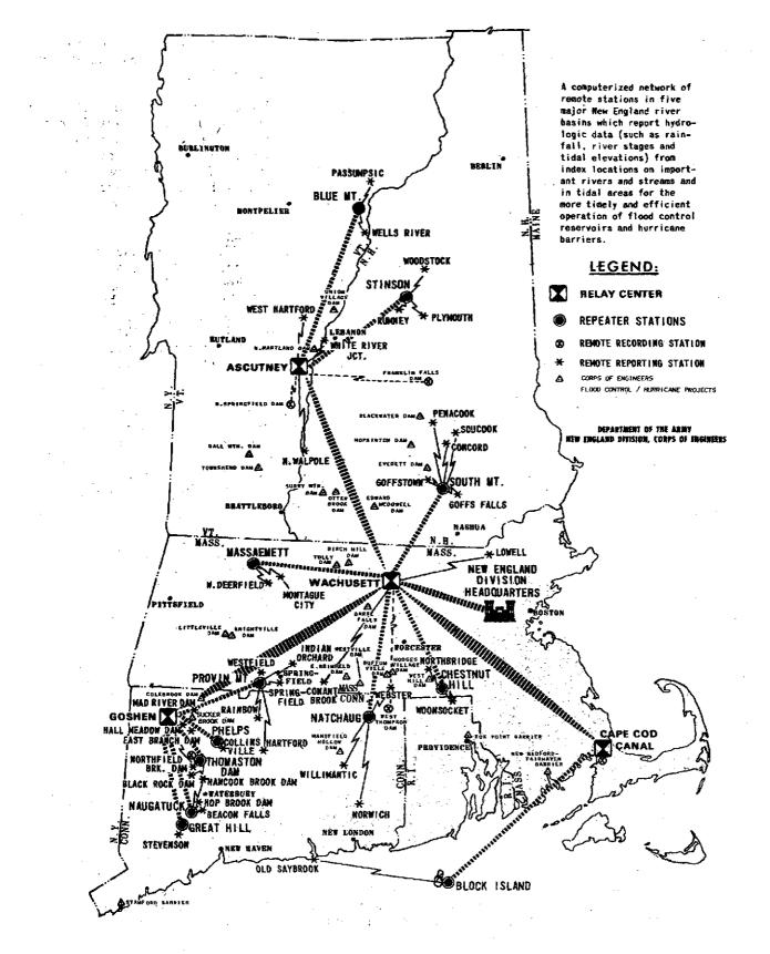
Figure 1. Automatic hydrologic radio reporting network
