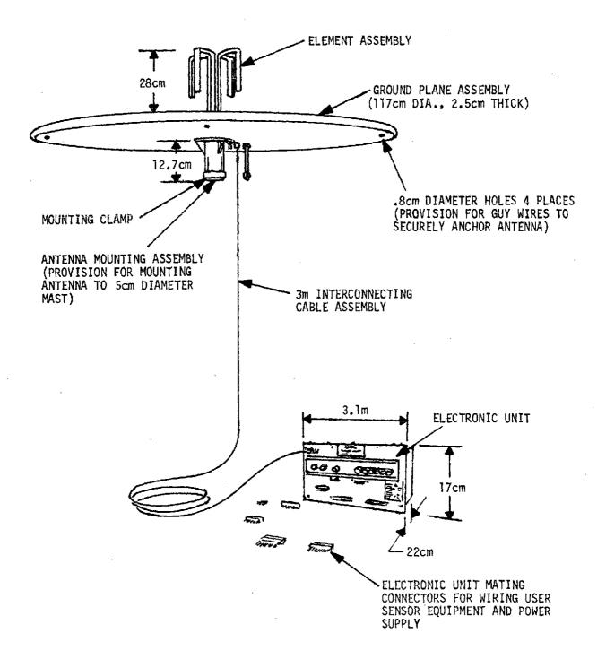
Figure 4. Data collection platform and antenna
