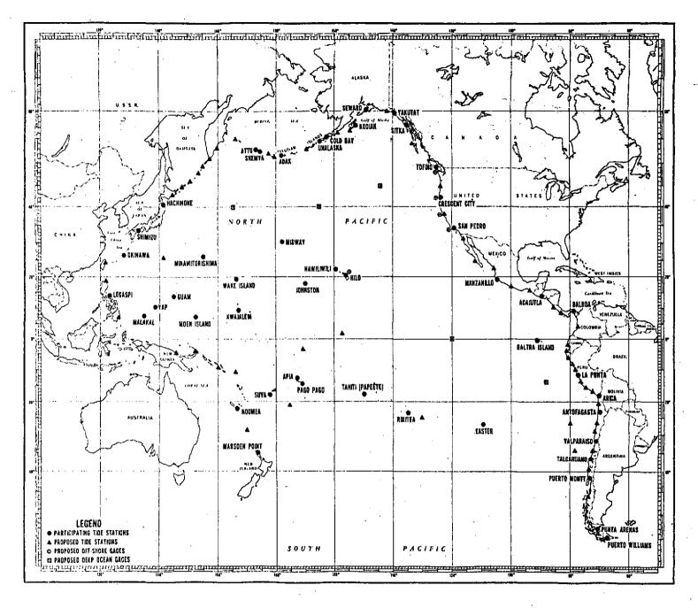
Figure 1. Participating and proposed tide stations in the Pacific Tsunami Warning System
