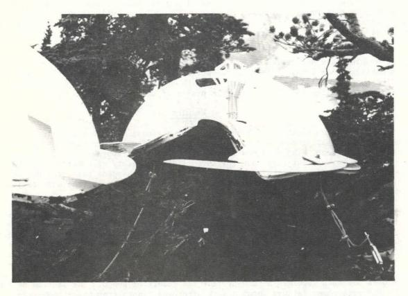
Figure 9. Antennas on Mt. Lassen destroyed by ice and snow
