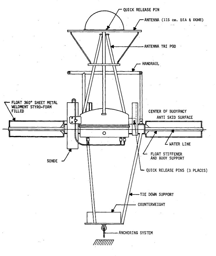
Figure 3. Salt water application earth resources buoy
