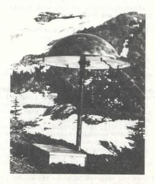
Figure 4. Typical installation of seismic event counter antenna, transmitter, batteries and steel box containing event counter are visible
