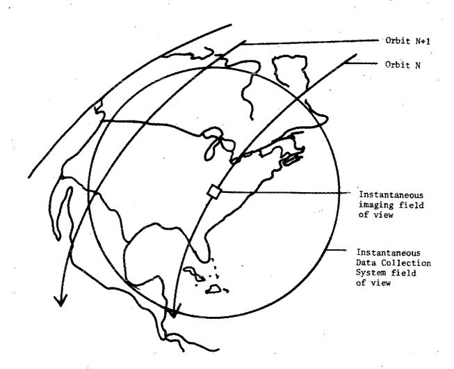
Figure 3. Sketch of two orbital transits over North America showing instantaneous fields of view of imaging and data collection system
